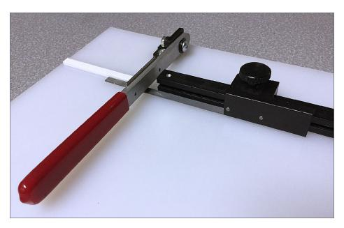
19. A closer view shows the fence and the sliding stop. You can see a piece of painted stripwood under the razor blade and up against the stop.
