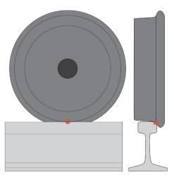
1. The electrical contact between wheels & rail is on the inside rail head and guite small.
