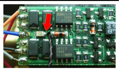
6. NCE D14SR negative (ground) connection location on the decoder circuit board. *Photo by Marcus Ammann*
