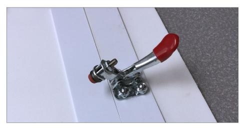
14. Here the hold-down toggle clamp is in the released position.
