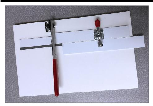
12. This experimental tool is set up to cut a piece of strip-wood. The moveable fence is held in place with a hold-down toggle clamp. Holding a piece of 1/4" material (a slider) between the stop and the fence didn't work out.
