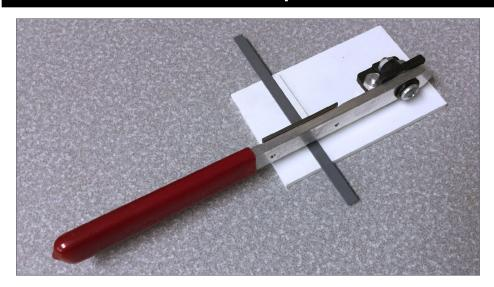
10. This tool to just cut a single piece of material to a desired length.
