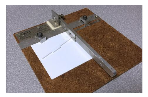
7. This is a custom cutting base for making angled cuts. The fence glued to the cutting base is at the angle required. A stop is bonded to the cutting base to result in multiple parts with both ends cut to the desired angle.
