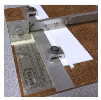
The fence on the replacement base needs to be positioned so that the Chopper clamps can hold it in place. I used 0.125" x 0.100"
