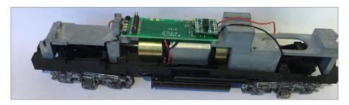
7. This is a new Atlas Silver DC decoder replacement. The Decoder Buddy installs in both directions and screws-in directly. In this locomotive the connector board should be accessible through the hatch on top.
