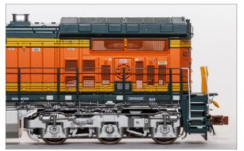
5. Close-up of rear radiator section and truck detail.
