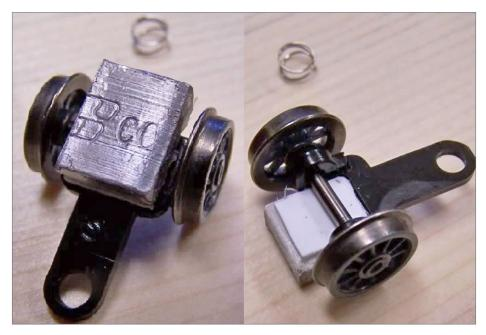
1. HVT Dave chose not to reduce weight on the drivers of his engine, so he removed the pilot truck spring, then added a weight directly to this Bachmann 2-6-0 pilot truck. The changes solved his derailment issues instantly. The top view (left) and bottom view (right) show the automotive stick-on wheel weight. HVT Dave photo
