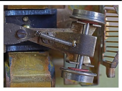
2. Some engines have a coil spring attached to the frame (left) and to the pilot truck (right). A longer spring will reduce down-force and a shorter spring increases it. Other engines will have a coil spring placed vertically to exert pressure. Clipping off one coil could increase pressure. Adding a spacer or stretching the spring will decrease pressure.
