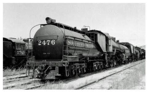
5. A unique feature for the Mayfield Branch engines was a road pilot mounted on the rear of the tenders. This modification was made because the locomotives ran backward between Los Gatos and San Jose at the end of the runs. To my knowledge, no other SP locomotives were modified in this way.
