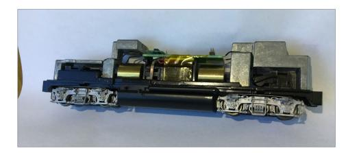
9. This is an Atlas dual-mode decoder replacement. First, place Kapton tape on the bottom of the Decoder Buddy. Then attach it to the motor with a piece of Kapton tape from one side of the motor to the other. For a little more room and a little neater installation, the clips that held the old decoder can be cut flush with the decoder support before attaching the decoder with the Kapton tape.
