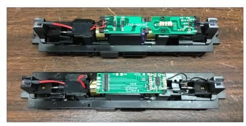
10. Two of Jim Moe's Proto1000 RSC2s before (top) and after (bottom) installing the Decoder Buddy. Sugar cube speakers might now fit in the extra space.
