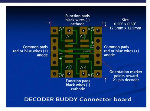
attaching function leads. With all function leads attached on this connector board, it allows for easily disconnecting the function leads when removing the loco shell for maintenance.
