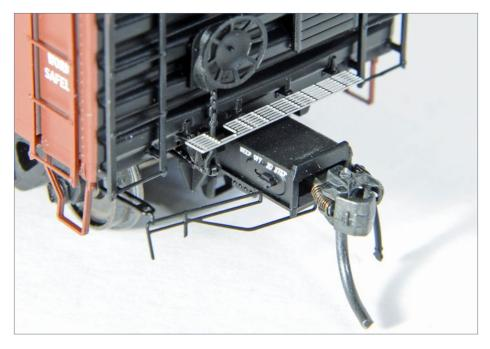
6. The coupler release lever on this Tangent Pullman-Standard PS-1 Mini-Hy cube boxcar telescopes to accommodate movement in the cushioned draft gear.
