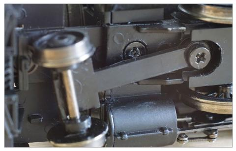
3. This plastic pilot truck could be weighted, if necessary. This one, on a small HO Bachmann 2-8-0, functions very well as it is.
