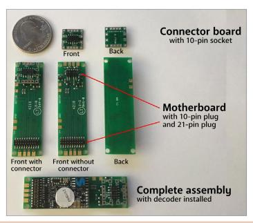
5. This picture shows both sides of the connector board and motherboard, all the associated plugs and sockets, and an installed decoder.
