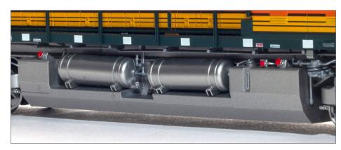
6. Close-up of fuel tank and air tank details.
