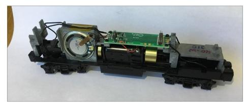
8. This is a mid-run Atlas Gold GP40 QSI replacement. There are eight wires to solder to the motherboard pads, or 10 if you include a stay-alive device.
