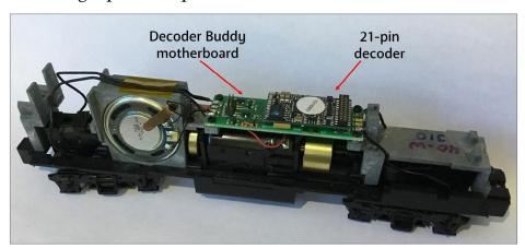
1. This is a completely installed and wired Decoder Buddy motherboard and a 21-pin decoder in an Atlas GP38 or GP40 frame.
