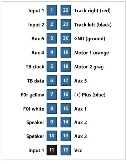
6. Standard NEM 21-pin decoder pin configuration used by decoder manufacturers.
