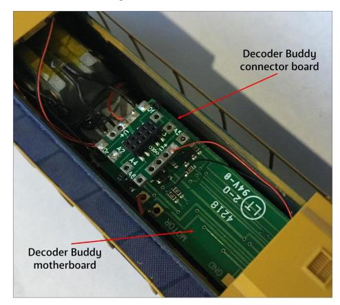
2. This shows the Decoder Buddy connector board installed with wiring to the LEDs attached. The 21-pin decoder is not installed for clarity. The shell is an Atlas GP38 of the dual-mode era.
