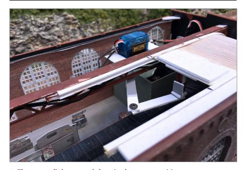
9. The servo, linkage, and door in the open position.
