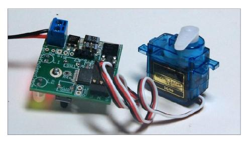
8. The Singlet control board and servo mechanism that powers the door. *Photo compliments of Tam Valley Depot*
