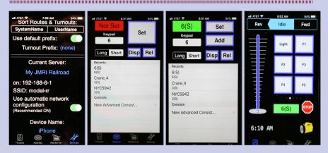
16-19. WiThrottle setup: server setup, enter loco address, set loco address, change to throttle and run!
