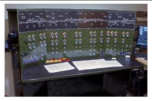
11. The UCW uses Centralized Track Control signaling and has this CTC machine adapted from real CTC machine parts salvaged by Rod Loder. Under the hood, Lee uses Bruce Chubb's CMRI to run the CTC panel and the associated signals on the layout.
