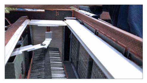
11. The linkage arms and attachment to the underside of the door. You can see some of the patchwork linkage arms where adjustments were made for smooth operation.
