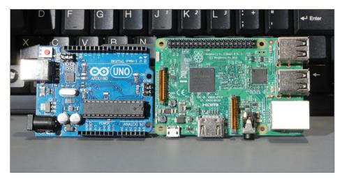
1. Arduino Uno (left) and Raspberry Pi 3B (right).
