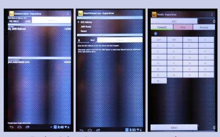
20-22. Engine Driver Setup: server setup, set loco address, change to throttle and run!
