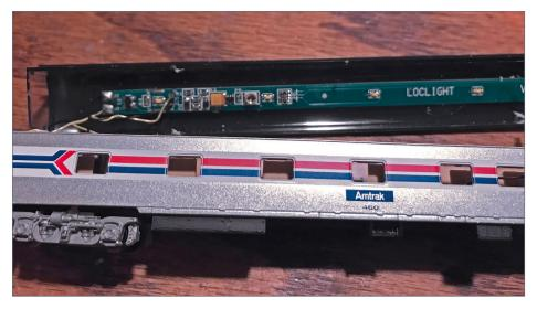
8. Circuit board mounted in the roof.
