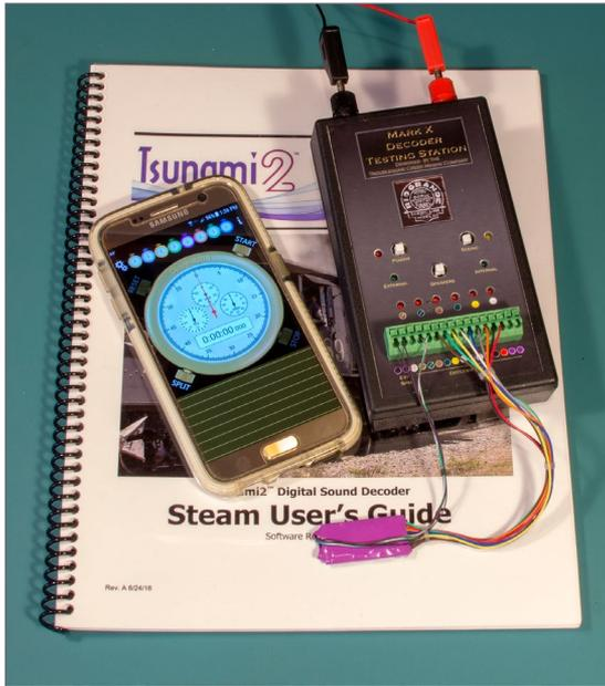
Prior to removing the decoder from the testing station, I will **<Write All Sheets>** and **<Save to Roster>** in DecoderPro. I do the remainder of programming after I
