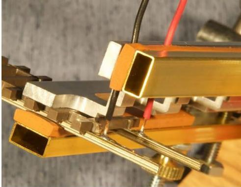
**Solder lead wires to bottom of rails**
