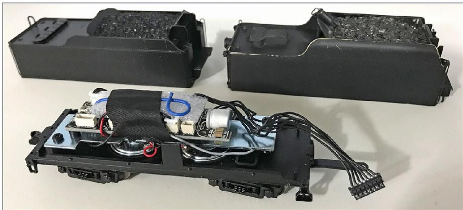
9. Broadway Limited tender chassis with electronics and twin speakers. In the back are the two different tender bodies – see the text for details.
