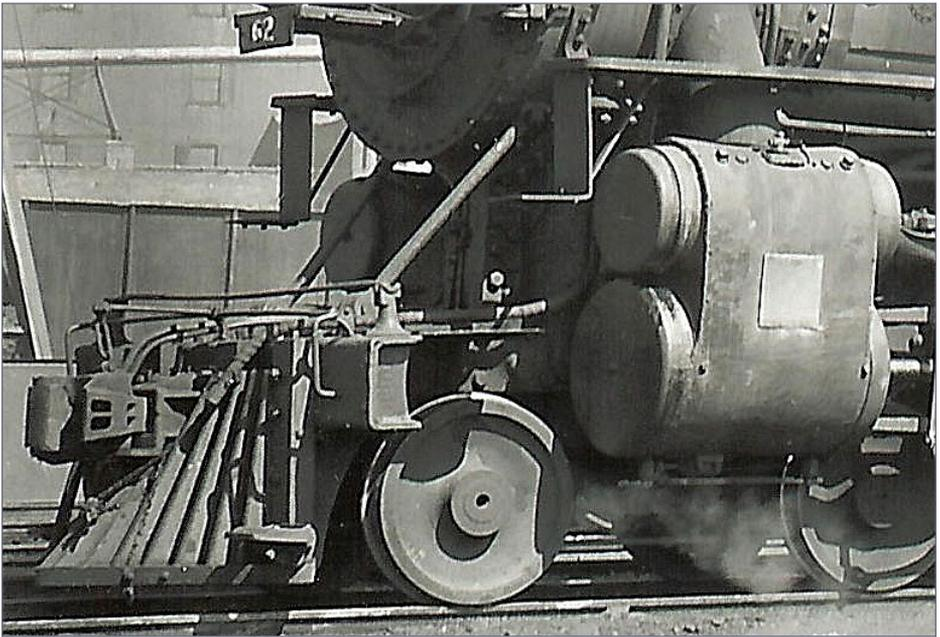
14. Loco pilot and its proximity to the front wheel of the pony truck.
