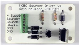
**Model Railroad Control Systems (MRCS)** is selling Sounder Driver, a compact circuit that boosts a logic low input and drives up to 10A @ 50V (momentary) load such as a telegraph sounder. The
