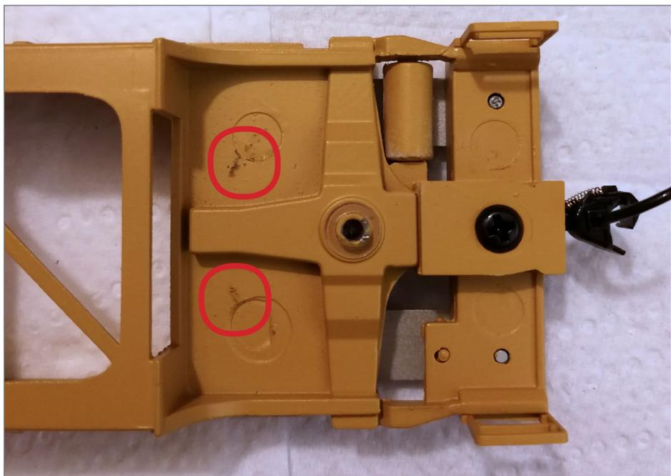
3. Here you can see the marks left by the wheels on the metal frame (marked by red circles).
