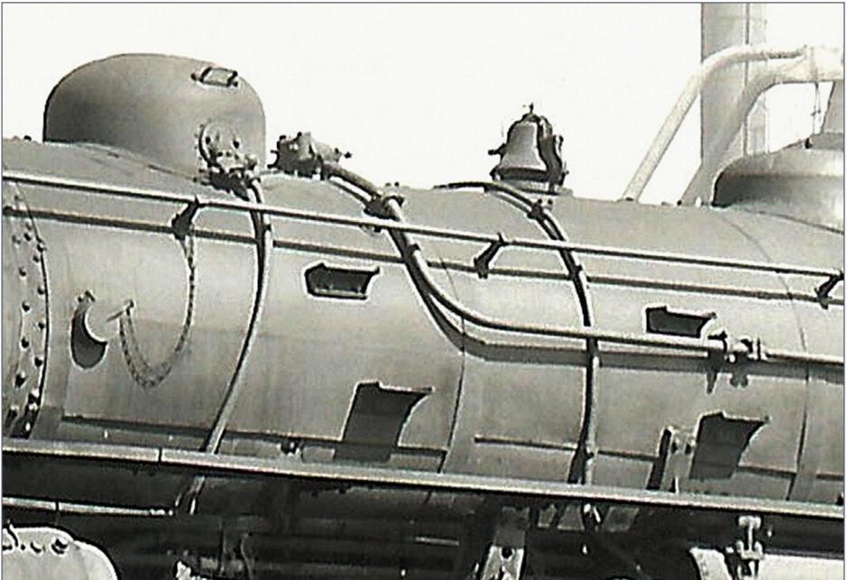
17. Boiler mid-section on the prototype loco.
