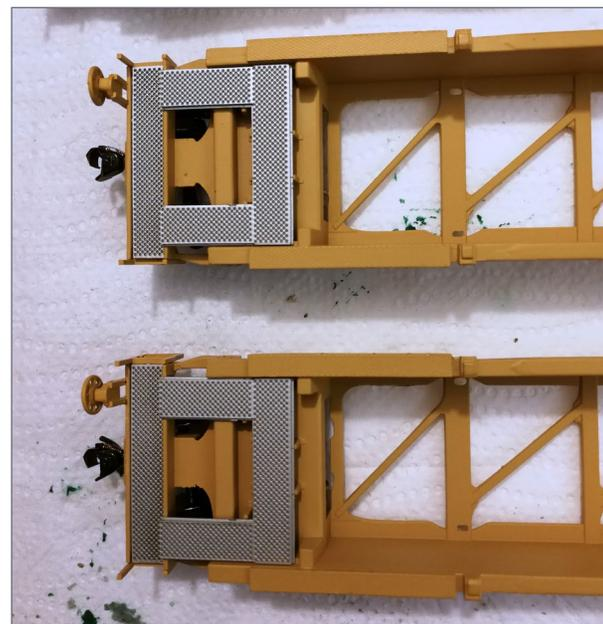
7. On top you can see a well car in its original state, below you see it after the modifications. You can barely see the notches, and they won't be visible at all when the car is loaded.
