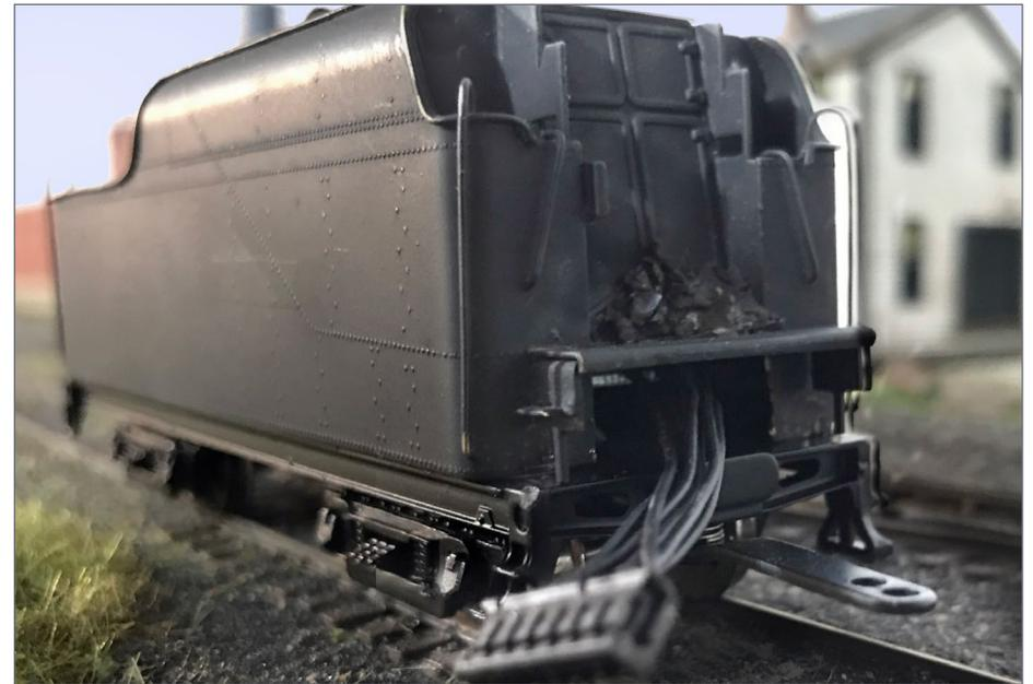
10. I needed to cut a slot in the replacement tender body to allow all the wires to pass through.
