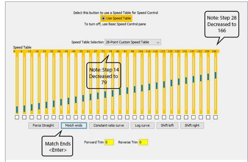
6. Adjusted linear speed curve.
