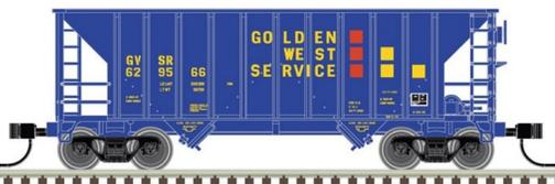
Atlas has included N scale versions of a Greenville 100-ton twin-bay open hopper car in its second quarter release. The prototype cars were used to haul a wide range of bulk commodities including rock, ballast, dirt, sand, gravel, and on some occasions, taconite ore.
