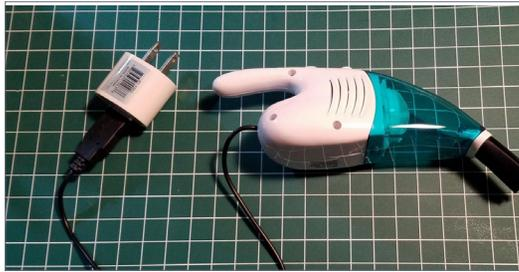
5. A two-prong USB adapter powers this palm-sized vacuum cleaner for layout work. *Two photos by Randolph Ghertler*
