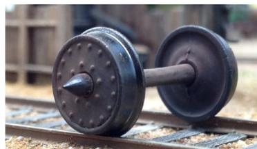
The wheel inserts are available for both 33-inch and 36-inch wheels in frets of 10, 14, 20, and 28 inserts.
