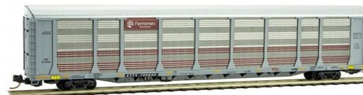
This Ferromex 89-foot tri-level enclosed autorack car represents a prototype built by Trinity
