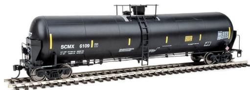
Walthers plans to release a new run of 55-foot 30,145 gallon tank cars this month. Walthers HO scale Proto series model is based on a Trinity
