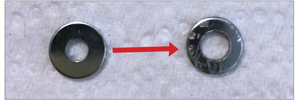
4. The original washer on the left, the same with its enlarged hole on the right.
