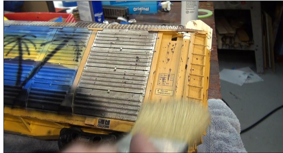
21. I rusted the rack a little with burnt umber oil paint speckled onto the sides of the model with a paint brush handle. The oils were then pulled down with a 1" artists brush to form rust streaks. With that, the model is ready for revenue service on your garden railroad, adding a splash of color to an already nice model. ☑
