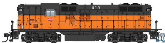
The release includes a Milwaukee Road version that follows a prototype in service from 1959 to the early 1980s. Details include spark arrestors, two single-chime horns, and a winterization hatch. Milwaukee Road's GP9s did not have dynamic brakes.
