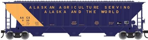
The design of Atlas's new Trainman series 4750 cu. ft. covered hopper with triple discharge bays is based on a Thrall-built prototype.
