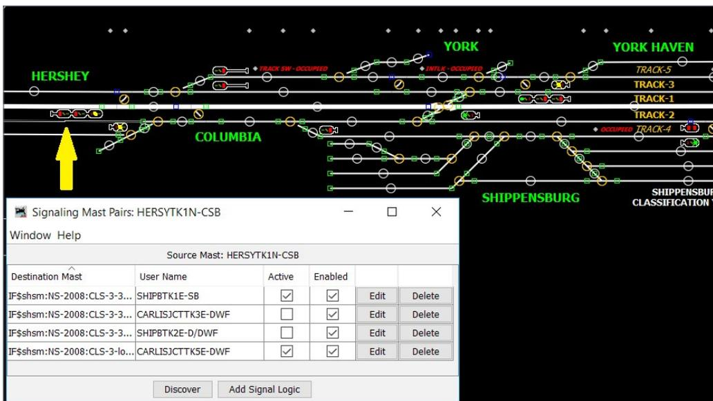
The signal mast in [33] is HERSYTK1N-CSB (Hershey, Track 1, north, cantilevered signal bridge). It has four routes that require signal logic to another mast and/or dwarf signal.
