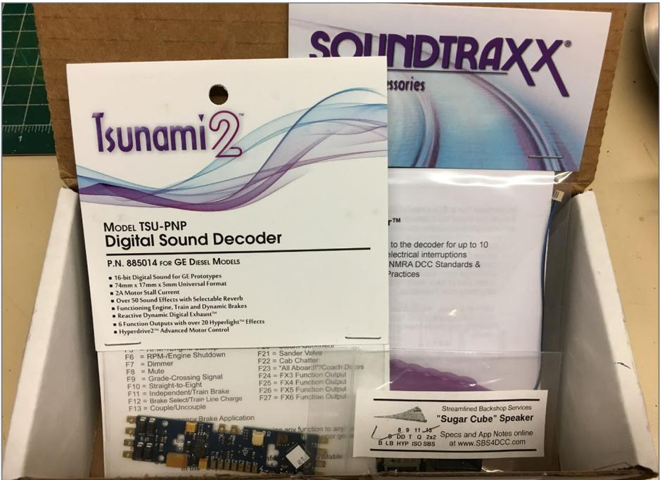
2. The sound equipment I purchased for the project: Tsunami2 decoder, CurrentKeeper, and a sugar cube speaker. I always like to test this as soon as possible to make sure everything works well while it is still under warranty.
