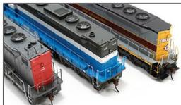
SP and GN long hood end is flat to allow room for steam generator equipment while the EL includes a pointed end. Note the steam generators are road specific.
