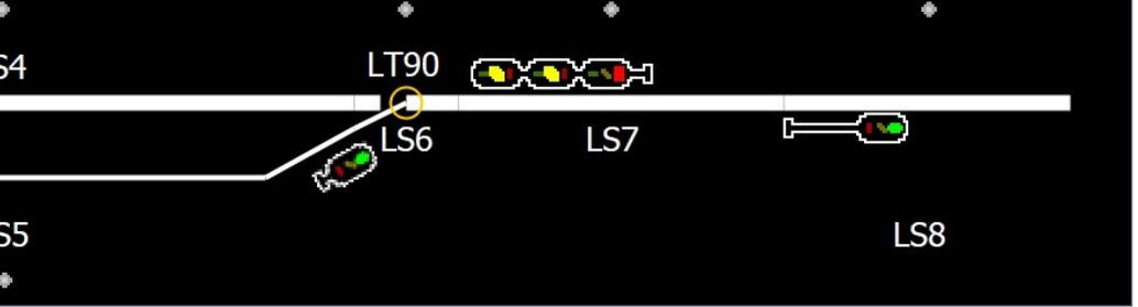
33↓. The triple-head mast signal to the top left corner of the signal logic window requires four sets of signal logic in Panel Pro to operate correctly.
