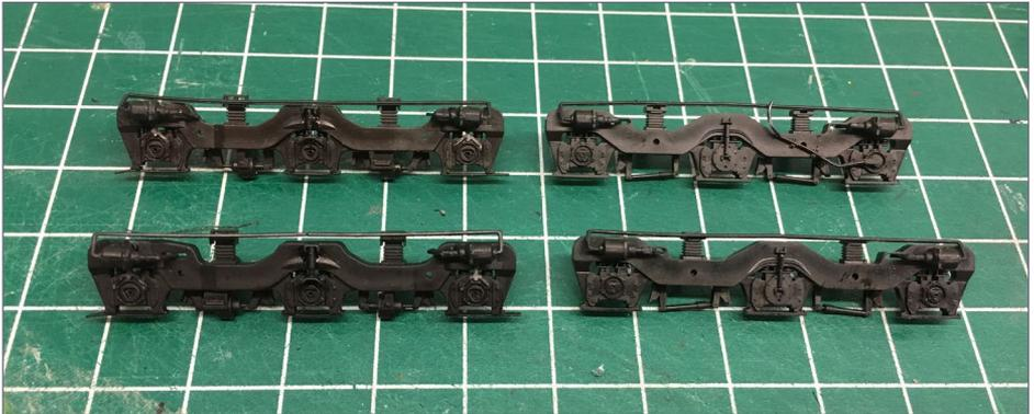
9. The Adirondack side frames after “rebuilding” (on the left), next to the newer GSC side frames. I used parts from the other pair of GSC side frames to update the Adirondack side frames. Now they look very similar, except for the placement of the holes.
