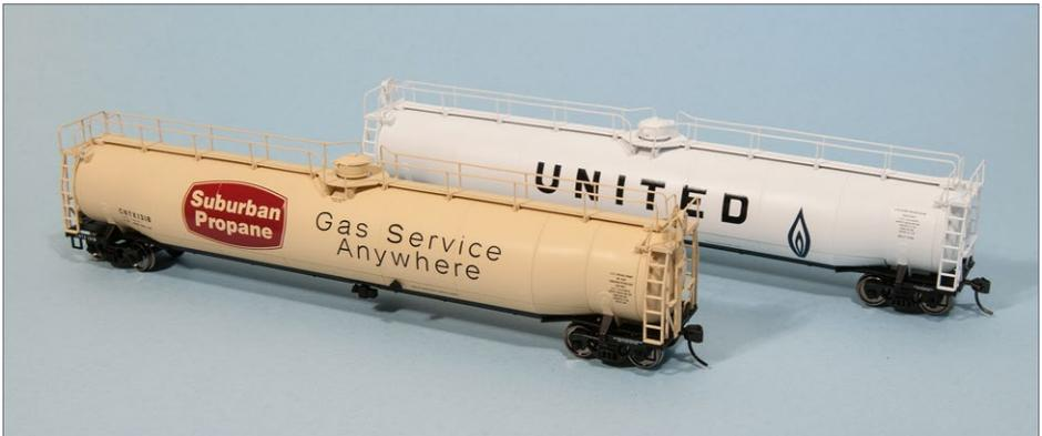
1. Atlas produced whale-belly 33,000-gallon tank cars stenciled for liquefied petroleum gas (LPG) service which carry build dates between March 1964 and September 1969. They can be found at swap meets and from online sellers. Walthers offered a "65' LPG Tank Car" lettered with an 11-68 build date. *Graham Line photo*
