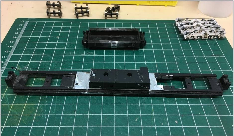
6. I had to mill down the ends of the metal block on the bottom of the chassis so the extended C30-7 fuel tank would fit. This was made easy work thanks to my Dremel motor tool. This also shows the fuel tank before painting, and the trucks after painting.
