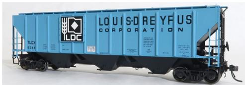
details include different stirrup steps, roof hatches, jacking pads, tow loops, discharge gates, side air lines, running board supports,
