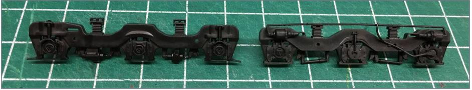
7. Compare the older Adirondack truck side frame and the newer GSC truck side frame. The Adirondack side frame is on the left and the GSC side frame is on the right.
