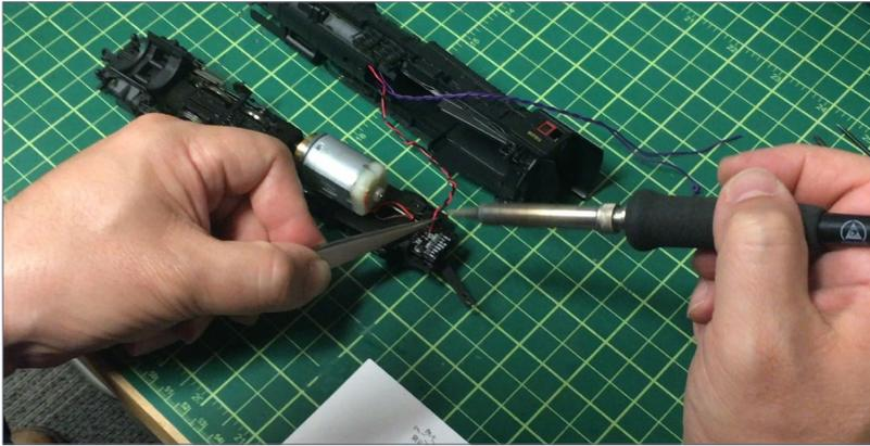
27. He makes a map of the wires, power positive and negative, the light wire feeds and speaker feeds, by drawing a diagram of the existing wires on a piece of paper. Following this chart, George solders the wires through the plug. He then reattaches the boiler to the power assembly.
