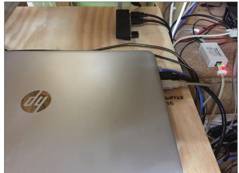
1. Here are the NCE Power Pro 5-amp Command Station and the RR CirKits LocoBuffer USB. These are connected to a computer computer via high speed USB ports. To ensure optimum transfer of data, use the fastest ports on your computer.
