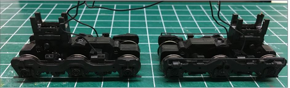
8. Test-fitting the older Adirondack side frame on one of the C40-8 truck assemblies. Again, the older Adirondack truck is on the left, and the newer GSC truck is on the right.
