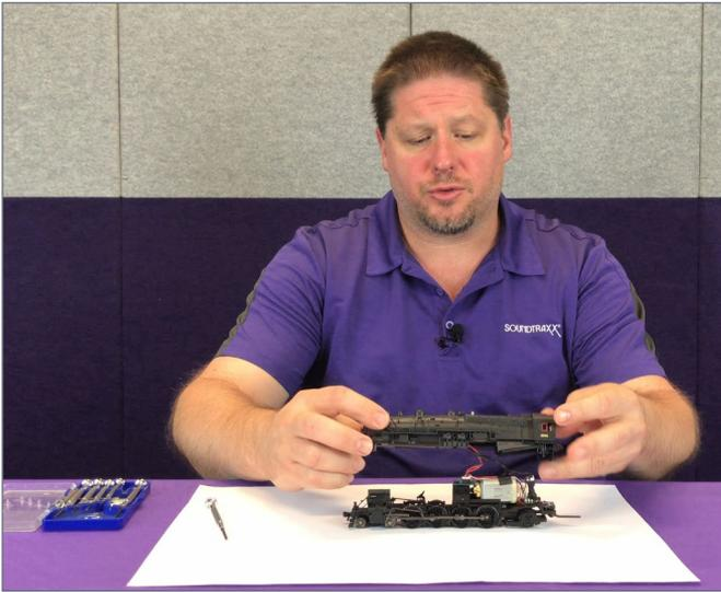
25. He removes the weight and smoke unit, which will not be reinstalled.
