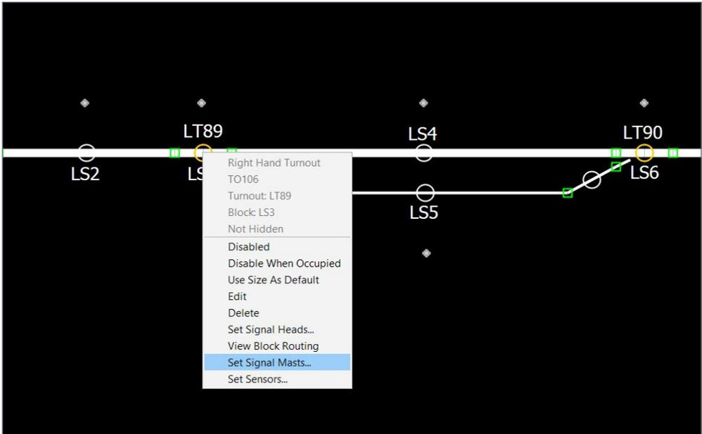
22. The “set a signal mast” at a turnout feature allows you to add a signal to the throat for the continuing and/or diverging routes of a turnout.
