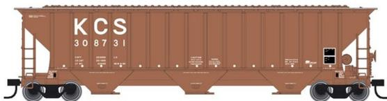
Design of the Trainman series model is based on a Thrall 4750 cu. ft. prototype with triple discharge bays.
