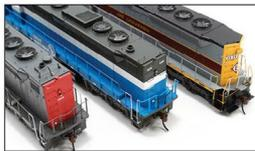
SP and GN long hood end is flat to allow room for steam generator equipment while the EL includes a pointed end. Note the steam generators are road specific.
