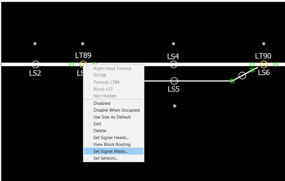
22. The “set a signal mast” at a turnout feature allows you to add a signal to the throat for the continuing and/or diverging routes of a turnout.
