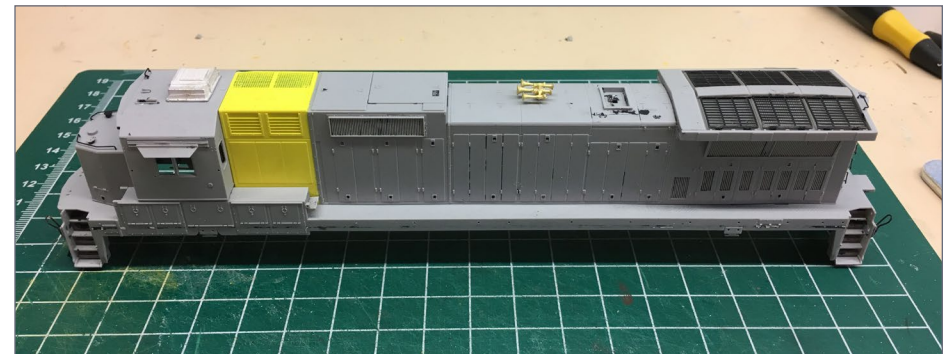
13. Test-fit the parts on the sill to make sure they have been filed down appropriately. The air conditioner is added to the top of the cab and the new five-chime brass air horn is attached to the center of the long hood. I will wait to add the exhaust stack so I don't have to repaint it silver.
