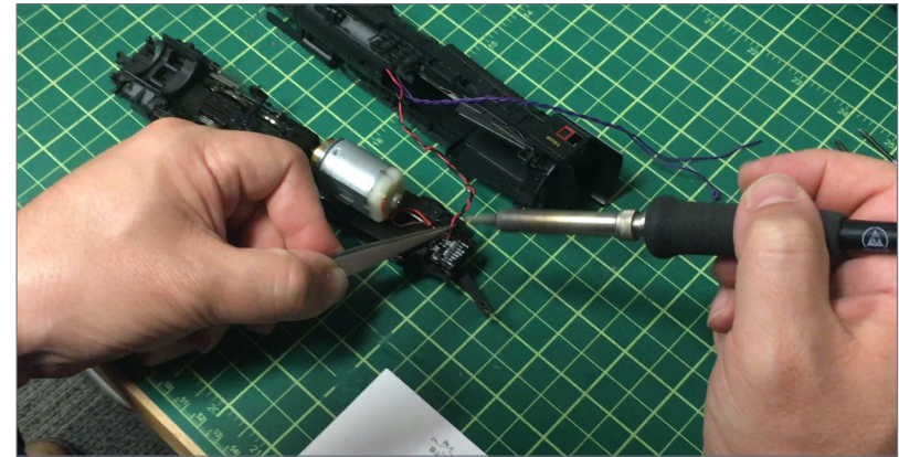
27. He makes a map of the wires, power positive and negative, the light wire feeds and speaker feeds, by drawing a diagram of the existing wires on a piece of paper. Following this chart, George solders the wires through the plug. He then reattaches the boiler to the power assembly.
