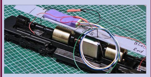
**57. Solder to decoder leads:** Thread some shrink tubing on the black and red decoder leads, and then solder the corresponding truck feeds to the same color decoder wire. Shrink the tubing over the bare solder joints to insulate them.
