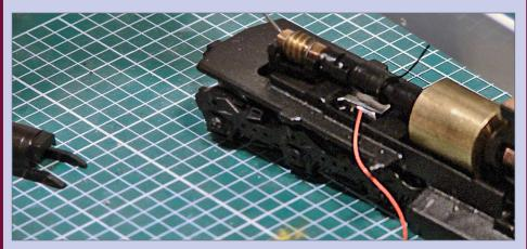
**54. Reinstall worm gears:** Install the worm gear on the truck and apply a drop of oil to the worm gear and each of the square worm gear bearings. Repeat for the other truck.
