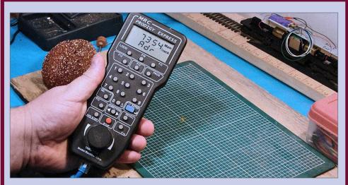
**59. Set loco address:** Having verified there are no shorts, put the loco on the programming track and set its address.
