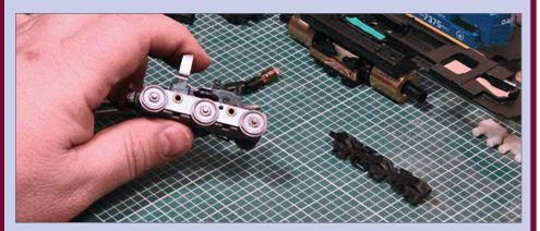
**18b. Success!** The side frame has been removed and the plastic pins are intact.
