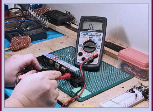
**58. Test for shorts:** Using the connectivity setting on a multimeter, check for shorts between the wheels and the motor housing, as well as between the wheels on the left and right sides.
