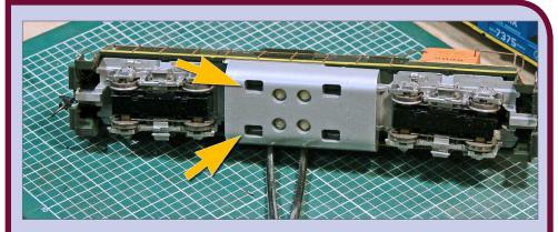
4. Some locos use bottom pins: These bottom internal shell retainers are used on some Blue Box locos.
