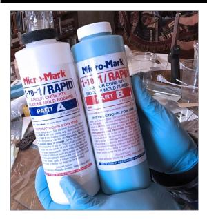
4. After letting the glue cure, it was time to mix and pour the rubber using the twopart material from the Micro-Mark resin casting starter set. Pour some of Part A in one cup and an equal amount of Part B in another cup.
