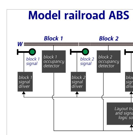
6. To make this simple four-block ABS system work for east-bound trains, these components are needed. If we also want signals for westbound trains, we will need another complete set of signals facing the opposite direction along the other
