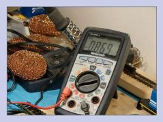
**7c. Reverse reading:** Stall current reading in reverse.
