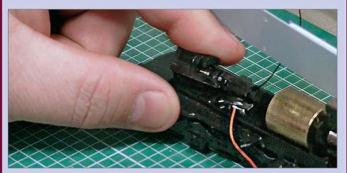
**55. Replace worm gear covers:** Snap the worm gear cover clip on. Repeat for the other truck.
