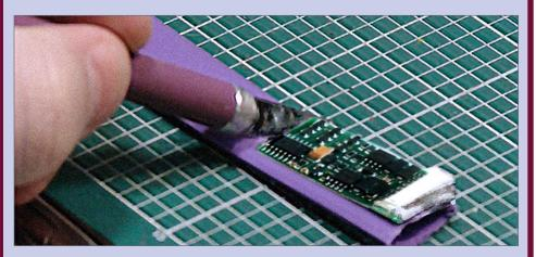
**37. Cut 1/2" shrink tubing:** Using the decoder as a guide, cut some 1/2" shrink tubing to length.
