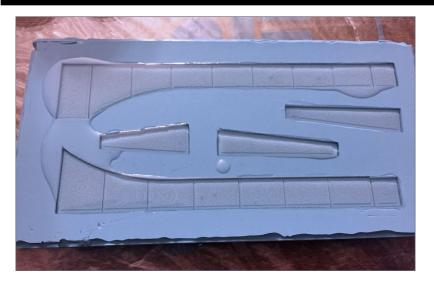
17. As before, I mixed equal parts of A and B together in a clear cup, then slowly poured the resin into the mold, doing my best to avoid bubbles. And – important (as I discovered later) – be sure to "overfill" the mold slightly. This is where making sure your foamcore box and mold are perfectly level pays off. And be sure you've put down some plastic to protect your workbench and catch any resin overflow.
