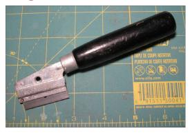
5. The hefty handle on a wallpaper knife makes a single edge razor blade easier to control and saves wear and tear on the fingers. *Dennis Snyder photo*  To make sharp, thin cuts, I prefer using single-edge razor blades. The only problem with them is that prolonged cutting and pressing down on that thin metal back tends to hurt your forefinger.
