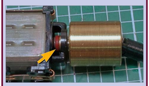
**35a, 35b. Lube motor bearings:** Lubricate the metal motor bearings on both ends with a drop of oil.
