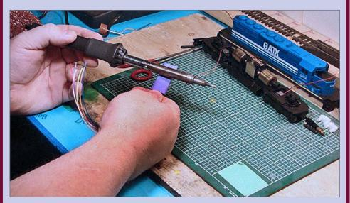
**42. Shrink tubing (soldering iron):** Alternatively, you can shrink the tubing by gently whipping it against the barrel of a hot soldering iron.
