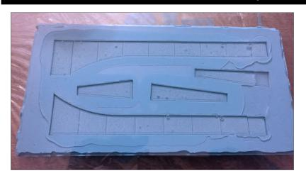
18. After over-filling the mold with resin, cover it with acetate or sheet styrene to keep the backs of the castings flat. As you can see, a few bubbles formed. I'm not sure yet how to avoid that, but decided they didn't matter since they'd be on the back of the castings.
