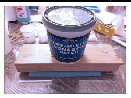
19. Lastly, weigh it all down to compress and flatten the resin. The instructions on the resin say it takes about 15-20 minutes to cure (you know it's cured when it turns from clear to white), but to be certain the casting was as hard as possible, I left it overnight.
