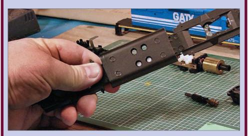
**14b. Access the mount from below:** Holes in the bottom of the fuel tank give access to the other motor mount.
