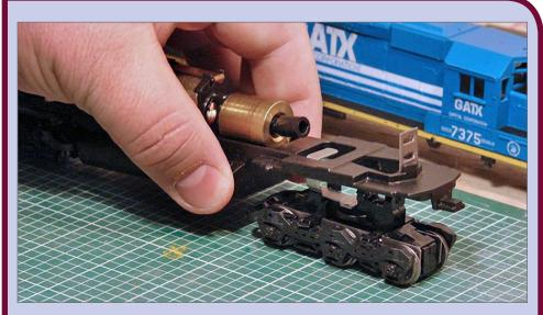
**12a. Remove trucks:** To remove a truck, lift the frame.
