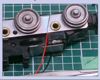
23. Tinned power lead placement: Place the tinned wire on the truck's metal plate as shown.
