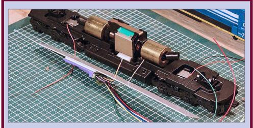
51. Reinstall motor: Install the motor back into the loco frame.
