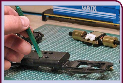
**14c. Poke other mount free:** Use a pencil or pen to press on the motor mount through the holes until the mount pops free.
