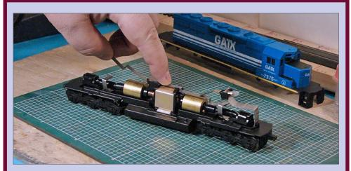
**9a. Removing the metal strap:** Slide the conductivity strap to one side to free it, then unclip it from the top of the motor.
