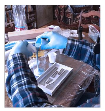
5. Then mix the two cups of material together in a third, clear cup. Be sure to scrape out all the material from each cup.
