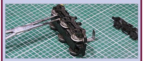
**18a. Remove truck sideframes:** Using a locking hobby clamp (hemostat), gently pry up with even pressure while pulling the side frame away from the truck.
