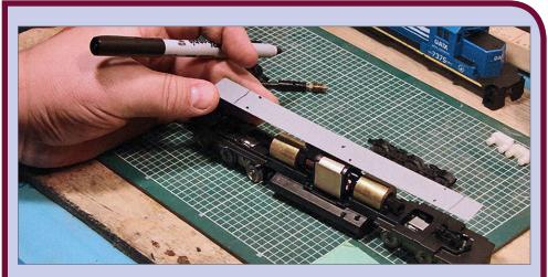
**31. Verify marks are correct:** Hold the piece up against the power chassis to verify correct positioning of the marks for the wires.
