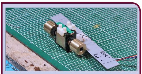
**50. Replace mounts:** Put the motor mounts back on the motor.
