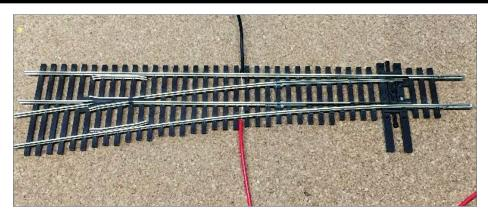
10. I solder feeders to the stock rails of my Insulfrog turnouts, and I also extend the feeders under the closure rails as well. This makes sure all parts of the turnout get power regardless of how well the points may contact the stock rails.
