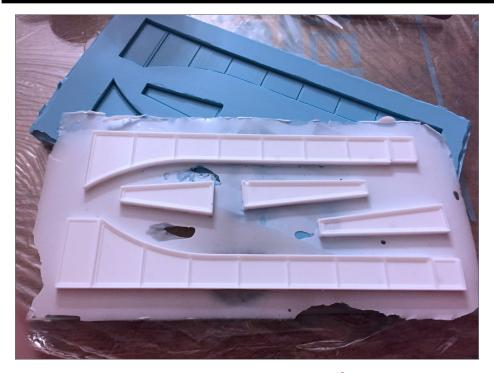
20. Once cured, remove the weight, peel off the acetate, peel the rubber mold off of the casting, and you should end up with something like this.
