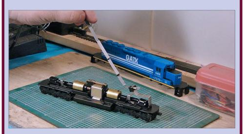
**9b. Set metal strap aside:** Once the conductivity strap has been removed, set it aside.
