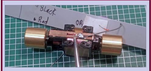
**48. Solder gray wire:** Solder the gray wire to the bottom retainer clip on the motor.
