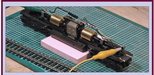
**8a. Motor contact cleaning set-up:** To clean the motor contacts, put the loco fuel tank up on something so the wheels can spin freely, and clip on test leads from a DC power pack.
