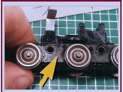
**22. If painted, sand off paint:** You may encounter a painted truck. You need to sand off the paint where the arrow is pointing, so the solder will stick to bare metal.
