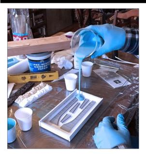
8. Pouring the rubber is both the most fun – it's cool to see it coming out of the cup and into the mold box – but also the most scary, since you're covering up, in this case, over \$40 worth of parts with liquid rubber. Start in one corner.
