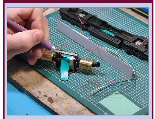
**36. Insulate motor top:** Apply some insulating electrical tape on each side of the top motor clip.
