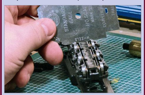
**16. Check wheel gauge:** While the loco is on the workbench, check the wheel gauge and correct any out-of-gauge issues.
