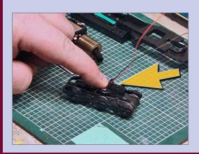
26. Lubricate truck gears: Lubricate the top gear (arrow) and then roll the truck back and forth to distribute to all gears.
