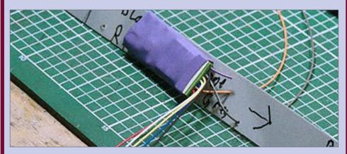
**45. Fix decoder in place:** Once you know the best location for the decoder, fix it in place to the shield with some double-stick foam tape.
