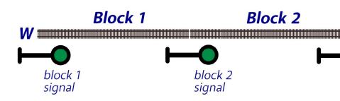
1. Four automatic block signaling blocks with eastbound signals and no trains. (For simplicity, the westbound signals on the other side of the tracks are not shown.)
