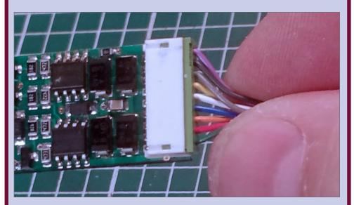
**39. Press in plug:** Press the wiring harness in place until it's firmly seated.
