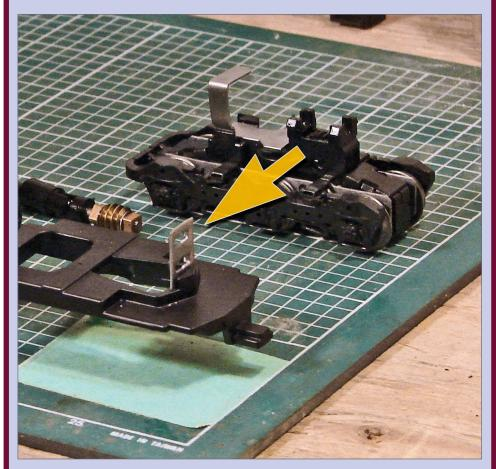
**15a. Light bracket:** The light bracket on the end of the frame needs to be removed.
