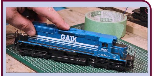
**62. Apply the shell:** Once you're sure no wires are caught or pinched, go ahead and slide the shell down onto the frame until the latches catch.
