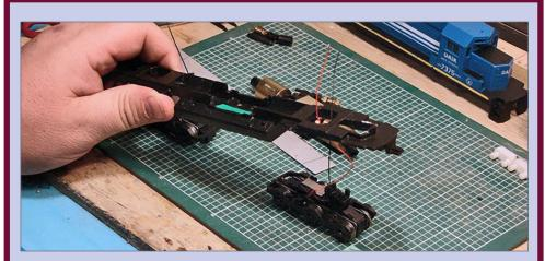
**27. Thread leads through frame:** Starting with the front truck, thread the new feeder wires into the hole closest to the fuel tank. Repeat for the rear truck.
