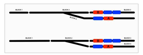
9. Here is an example of how breaking up junctions and turnouts into their own blocks helps streamline traffic flow. On the top diagram, train B is blocked by train A because the turnout is part of block 2. In the lower diagram, putting the turnout into its own block allows train B to move.
