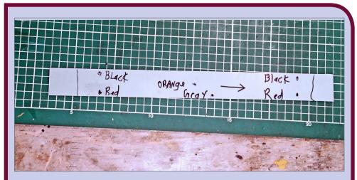
**33. Label the holes:** Label all the wire holes, and mark the front of the shield with an arrow.
