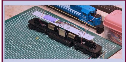
**56. Thread feeds through shield:** Thread the red and black truck wire feeds through the holes in the shield.
