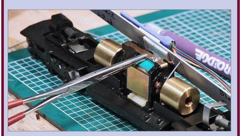
**52. Solder orange wire:** Solder the orange wire to the top motor clip. Note the double-stick foam tape applied to the underside of the shield.
