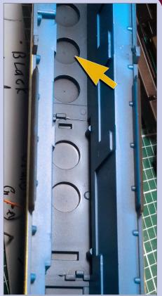
44b. Under rear fans: Another good decoder location is to the rear under the radiator fans (see arrow).
