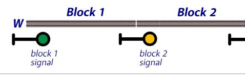
4. The eastbound train enters block 3, causing the block 3 signal to go red, block 2 to go yellow, and block 1 to go back to green.
