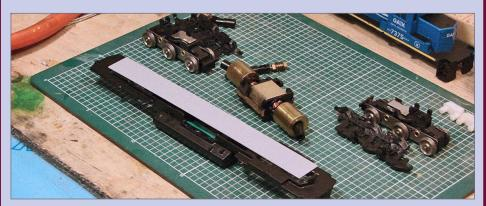
**29. Wire shield:** Make a wire shield out of 0.020" styrene. Measure it to fit the frame. Make it the width of the decoder and no more so it will fit easily inside the shell.
