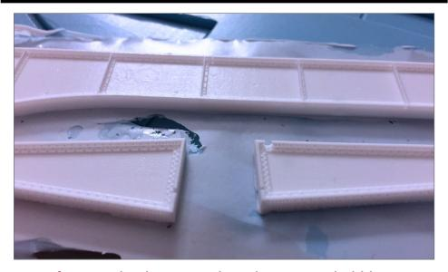
21. Unfortunately, there must have been some bubbling along a few of the girder edges. You can see above what look like "chips" that broke off. Nope – that's how the casting came out. This should be a relatively simple matter of filling them in with either putty or strip styrene, but I might not even bother, since these castings will be painted black and put under a bridge next to the backdrop.
