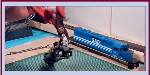
**10a. Remove light bracket:** Lift and rock the light bracket to pry it loose from its mount.
