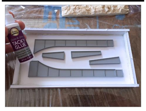
3. Next, I used Aleene's Quick Dry Tacky Glue to attach the masters to the base of the box. To (try and) ensure that no rubber would seep underneath the masters, I ran a bead of glue around the entire perimeter of each part to, I hoped, form a nice seal/barrier. I wasn't too concerned about messing up the nice masters, since the Aleene's would just soak off with water. Make sure your box is absolutely level so your mold will come out level as well.
