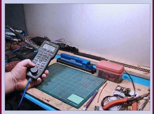
**60. Test run loco:** Once the loco address has been set, put the loco on some normal running trackage and give it a try. Make sure it runs freely with no binds or abnormal sounds.
