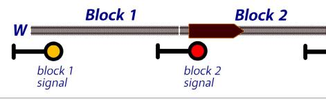
3. The eastbound train enters block 2, causing the block 2 signal to go red and the block 1 signal to go from red to yellow.
