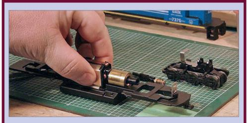
**13a. Remove motor:** To remove the motor, gently rock it from side to side, working the motor mount free.
