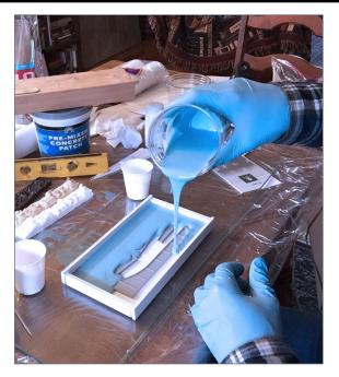
10. Pour throughout the mold box, covering everything with hopefully enough material – at least 1/8" above the tallest part of the master. I had extra cups waiting in case I had to mix up more rubber quickly. To reduce bubbles, pour from high up so you have a thin, steady stream.
