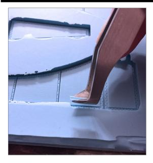
15. But that's next time. For now, I had some trimming to do. After trying a sharp X-Acto blade, I came up with the perfect solution – sprue nippers! As you can see above, they're straight and flush-cutting. Just what I needed to go around and trim off the extra rubber "flash."
