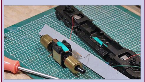
**49. Insulate bottom motor clip:** Cover the soldered area on the bottom of the motor with electrical tape to keep the motor isolated from the frame.
