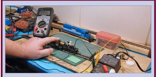
**7a. Current-draw test set-up:** Here is my set-up for testing current draw, with a power source and a multimeter.
