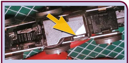
**20. Cut level with top plate:** Cut the bracket level with the top plate of the truck, and make sure there is still a gap.
