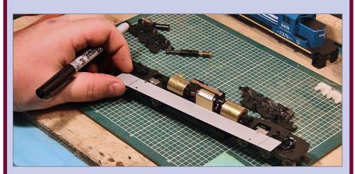
**30. Mark wire locations:** Mark the spots for the wires – two on each end for the truck wires and two over the motor for the motor wire feeds.
