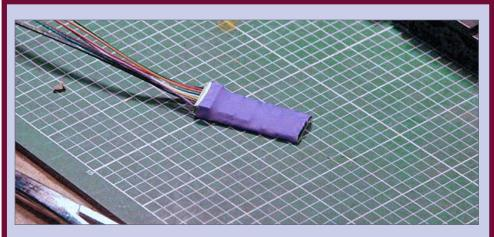
**41. Shrink tubing (heat gun):** Heat the shrink tubing carefully with a heat gun to shrink it up.
