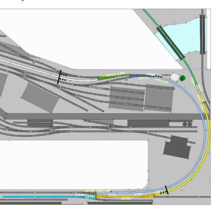
My first question was "How big does a block need to be?" Many sources recommend blocks longer than the length of your average train, or the maximum-length train you ever expect to operate. This way the signal system will function like the prototype, even on our condensed model railroads.
