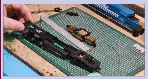
**28. Drop frame onto trucks:** Lower the frame fully down onto the trucks – first the front truck, then the rear truck.
