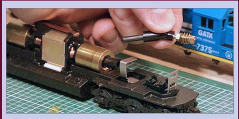
**11c. Set aside worm gear and shaft:** Pull the shaft out of the coupler on the flywheel and carefully set the worm gear assembly aside. Be careful not to lose any of these parts!
