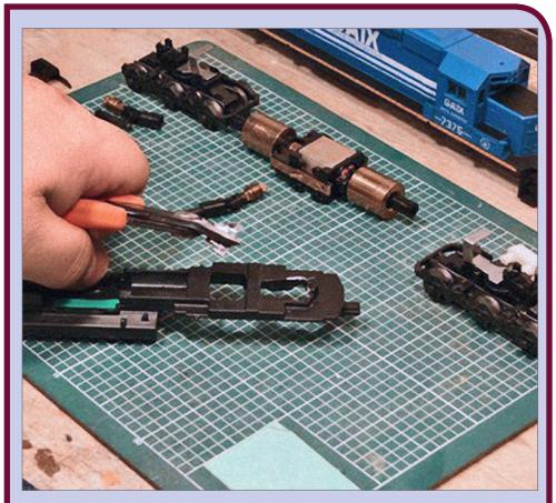
**15b. Bend until snaps free:** Bend it back and forth with pliers until it breaks loose.
