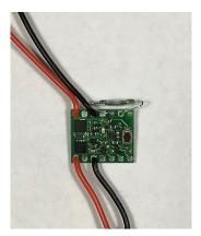
**Dead Rail Installs** is selling an on/off switch actuated by a magnetic reed. The device will control any electronic circuit and can be installed inside a locomotive, tender, or car. It can also be installed under scenery or inside a structure. The switch is turned on or off by waving a magnet near the hidden device. The unit is .6 x .6-inches square, by .7-inches high. For more information visit deadrailinstalls.com.
