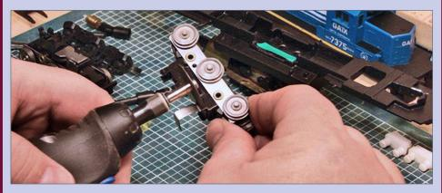
**19. Cut off L bracket:** Use a motor tool with a cutoff disk to cut the metal L bracket off the truck.
