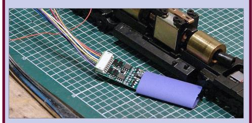
**40. Insulate decoder:** Slip the shrink tubing over the decoder.
