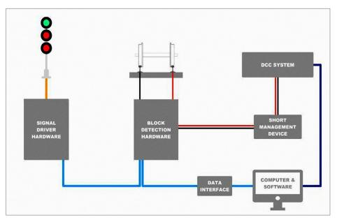
2. This diagram shows how the different parts of my signaling system relate to one another, and how they interconnect. Specific systems may vary.
