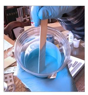
7. When the materials are thoroughly mixed together, you're ready to pour. Well, almost. Set the cup down and tap on the sides for a minute or so to encourage any bubbles to surface so they'll pop. This material has a 10-minute working time from mix to pour, so you have some time for this step.
