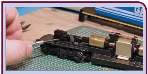
**11a. Remove worm gear clip:** Pry up on the middle of the worm gear cover clip to remove it.
