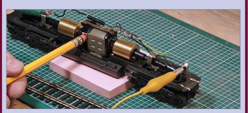
**8b. Clean motor contacts with pencil eraser:** Turn up the DC power to a good speed, then take a pencil with a soft pink eraser and hold it against the motor contacts (commutator) as it spins to clean off built-up carbon.
