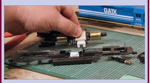
**13b. Lift motor free:** Once the motor is free, lift it from its mount. The other mount will typically stay in the frame.
