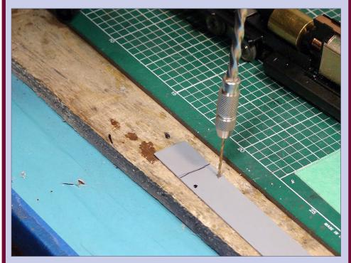
32. Drill holes: Using a #56 bit, drill out the marked wire holes.
