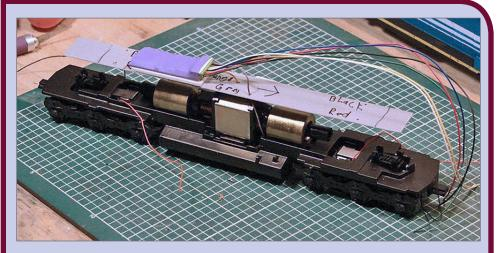
**53. Test fit shield:** Without taking the backing paper off the foam tape, check the fit by temporarily positioning the shield on top of the motor.
