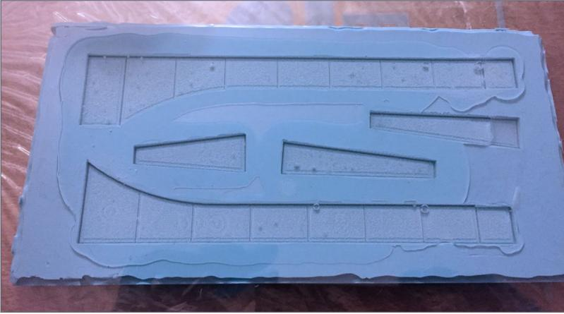
18. After over-filling the mold with resin, cover it with acetate or sheet styrene to keep the backs of the castings flat. As you can see, a few bubbles formed. I'm not sure yet how to avoid that, but decided they didn't matter since they'd be on the back of the castings.
