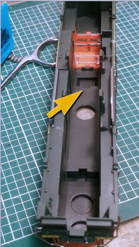
**44a. Behind cab:** One good location for a decoder is just behind the cab area but in front of the dynamic brake (see arrow).
