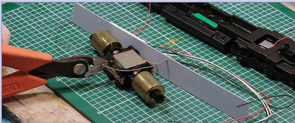
**47. Trim gray wire:** Cut the gray wire so it is long enough to reach the bottom of the motor.
