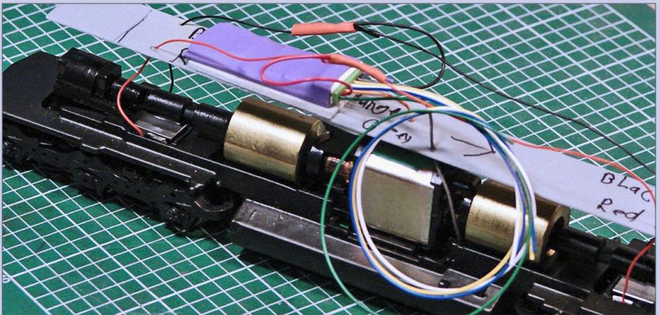
**57. Solder to decoder leads:** Thread some shrink tubing on the black and red decoder leads, and then solder the corresponding truck feeds to the same color decoder wire. Shrink the tubing over the bare solder joints to insulate them.
