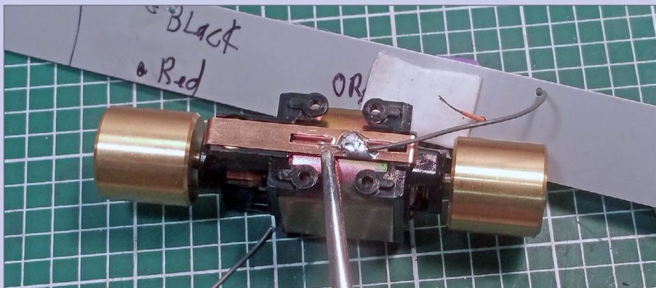
**48. Solder gray wire:** Solder the gray wire to the bottom retainer clip on the motor.
