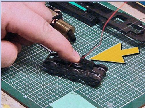
**26. Lubricate truck gears:** Lubricate the top gear (arrow) and then roll the truck back and forth to distribute to all gears.
