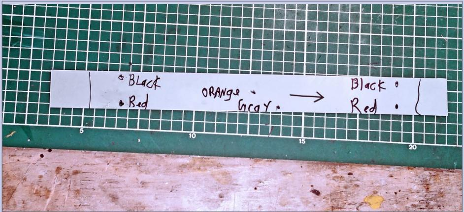
**33. Label the holes:** Label all the wire holes, and mark the front of the shield with an arrow.
