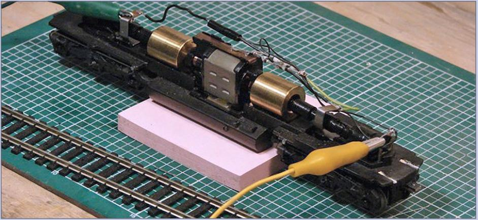
**8a. Motor contact cleaning set-up:** To clean the motor contacts, put the loco fuel tank up on something so the wheels can spin freely, and clip on test leads from a DC power pack.
