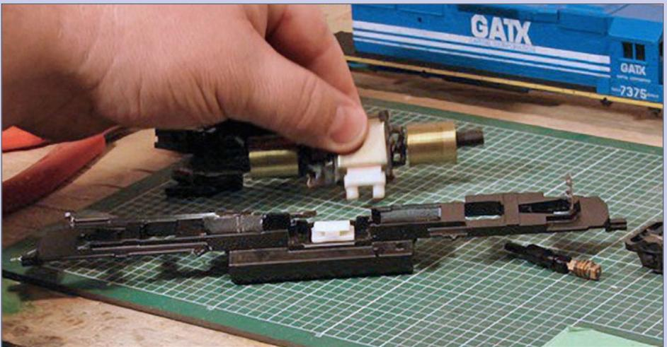
**13b. Lift motor free:** Once the motor is free, lift it from its mount. The other mount will typically stay in the frame.
