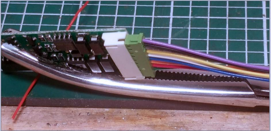
**38. Align plug:** Line up the wiring harness key.
