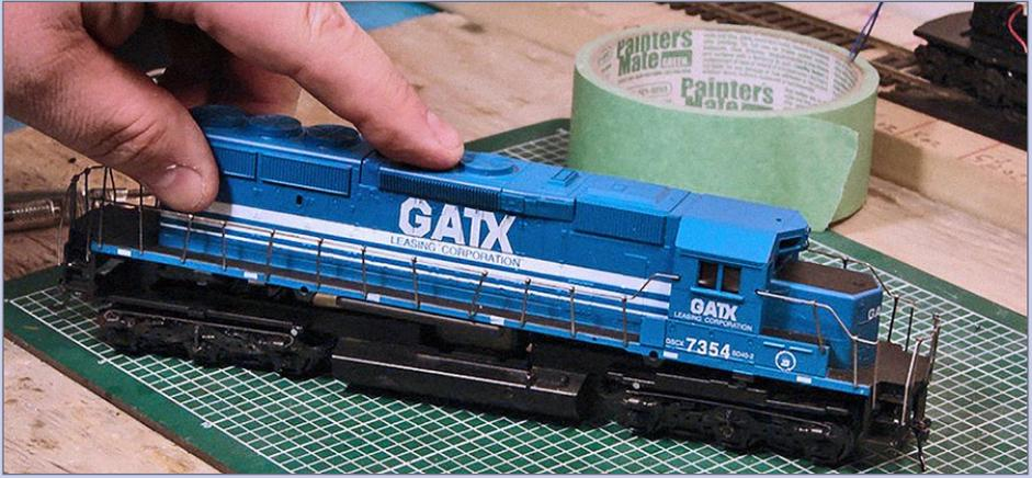
**62. Apply the shell:** Once you're sure no wires are caught or pinched, go ahead and slide the shell down onto the frame until the latches catch.
