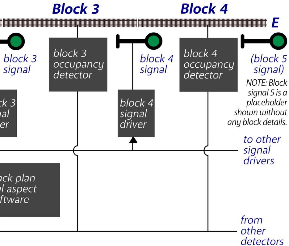
side of the tracks, along with signal drivers for them. As you can see, the total number of parts for this simple four-block ABS signaling system is significant.
