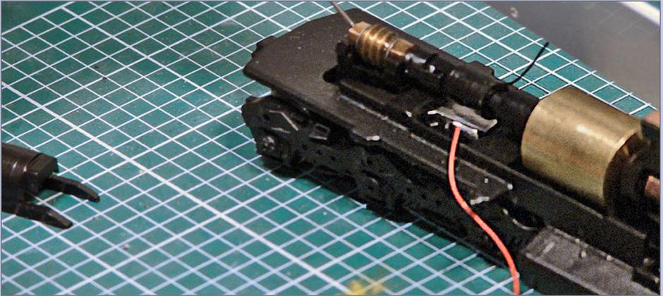
**54. Reinstall worm gears:** Install the worm gear on the truck and apply a drop of oil to the worm gear and each of the square worm gear bearings. Repeat for the other truck.
