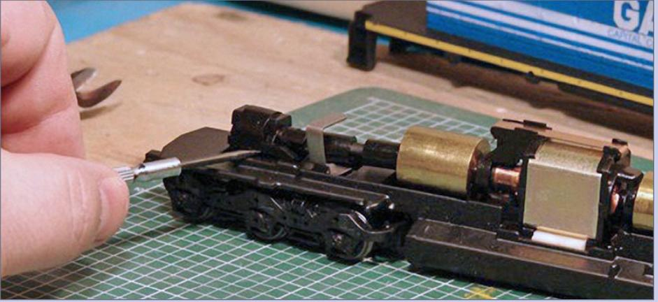
**11a. Remove worm gear clip:** Pry up on the middle of the worm gear cover clip to remove it.
