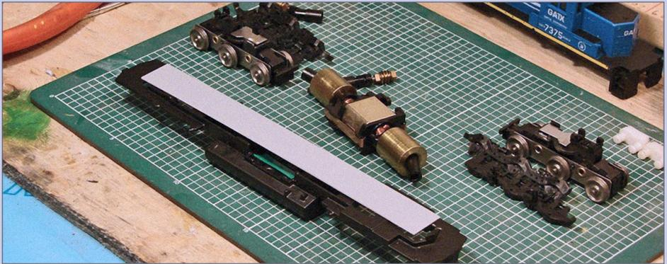
**29. Wire shield:** Make a wire shield out of 0.020" styrene. Measure it to fit the frame. Make it the width of the decoder and no more so it will fit easily inside the shell.
