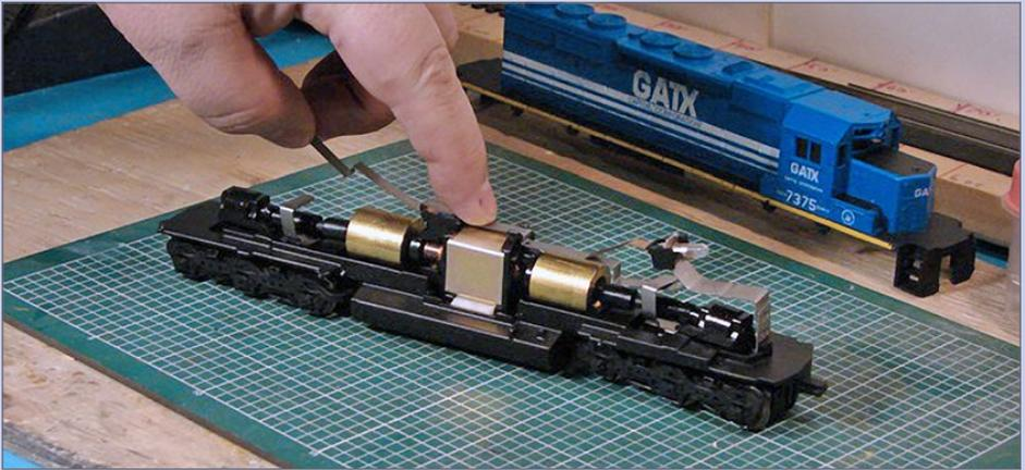
**9a. Removing the metal strap:** Slide the conductivity strap to one side to free it, then unclip it from the top of the motor.
