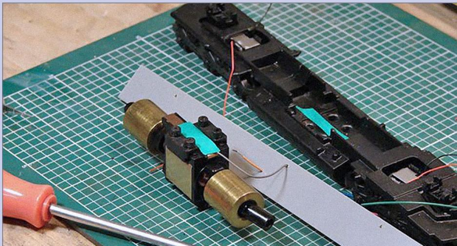
**49. Insulate bottom motor clip:** Cover the soldered area on the bottom of the motor with electrical tape to keep the motor isolated from the frame.
