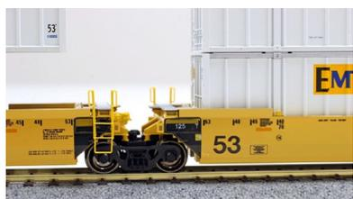
Like the prototype, the three-unit articulated model has two different sized wheels. The end trucks have 33-inch wheels while the two middle trucks, which carry more weight, have 38-inch wheels.
