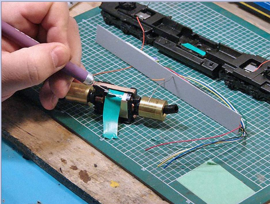
**36. Insulate motor top:** Apply some insulating electrical tape on each side of the top motor clip.
