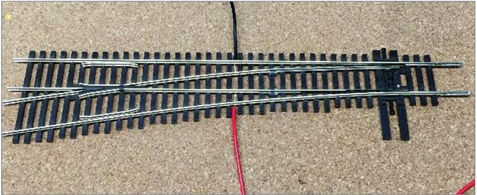
10. I solder feeders to the stock rails of my Insulfrog turnouts, and I also extend the feeders under the closure rails as well. This makes sure all parts of the turnout get power regardless of how well the points may contact the stock rails.
