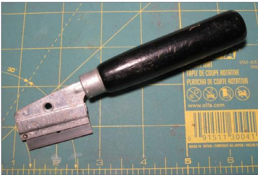
**5. The hefty handle on a wall-paper knife makes a single edge razor blade easier to control and saves wear and tear on the fingers. *Dennis Snyder photo***
