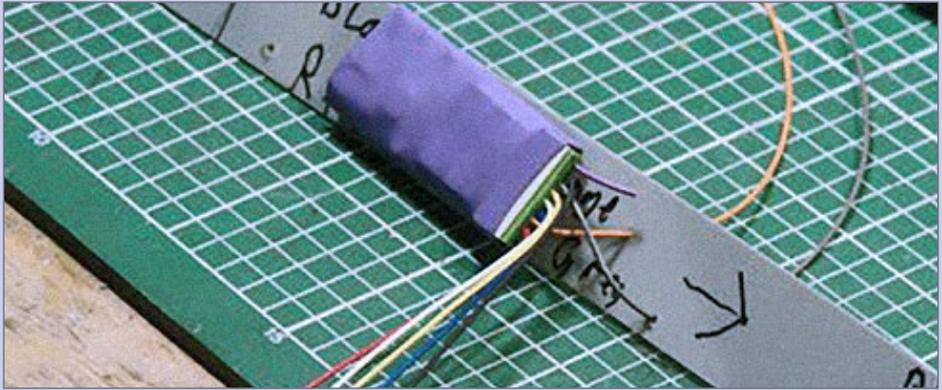
**45. Fix decoder in place:** Once you know the best location for the decoder, fix it in place to the shield with some double-stick foam tape.
