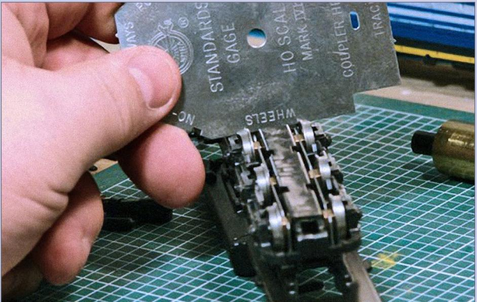
**16. Check wheel gauge:** While the loco is on the workbench, check the wheel gauge and correct any out-of-gauge issues.
