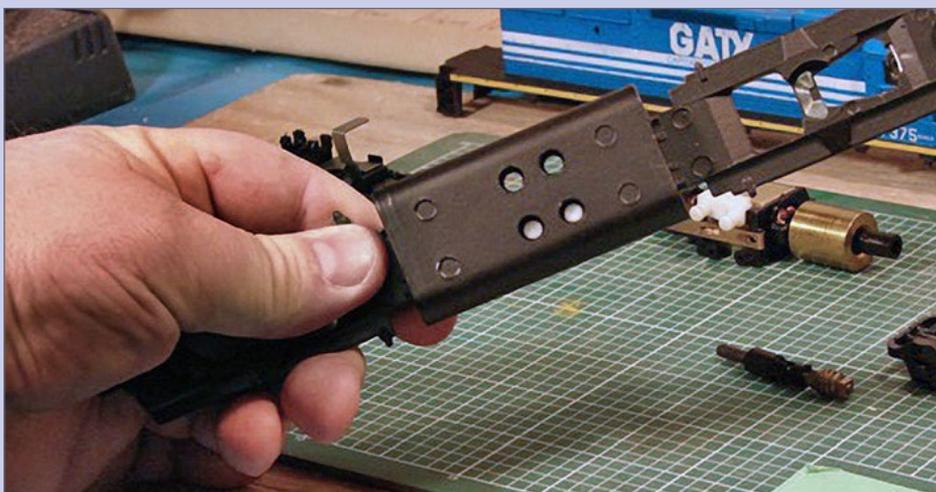
**14b. Access the mount from below:** Holes in the bottom of the fuel tank give access to the other motor mount.
