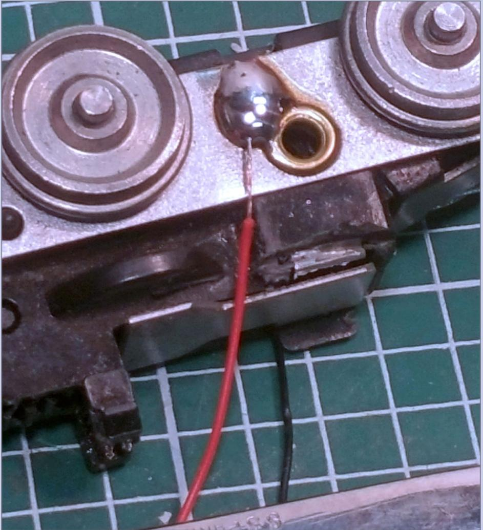
**24. Apply the solder:** Work quickly with the iron to avoid melting the plastic assembly behind the metal plate. (*Less solder works just as well. – ed.*)
