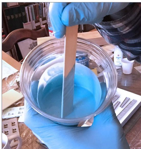
7. When the materials are thoroughly mixed together, you're ready to pour. Well, almost. Set the cup down and tap on the sides for a minute or so to encourage any bubbles to surface so they'll pop. This material has a 10-minute working time from mix to pour, so you have some time for this step.
