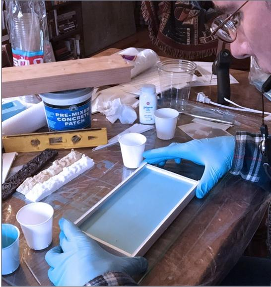
12. The final step, as with the rubber in the cup, is to tap on either side of the mold box to encourage the bubbles to surface and pop. Tapping releases the bubbles, and blowing across the surface helps them pop faster.
