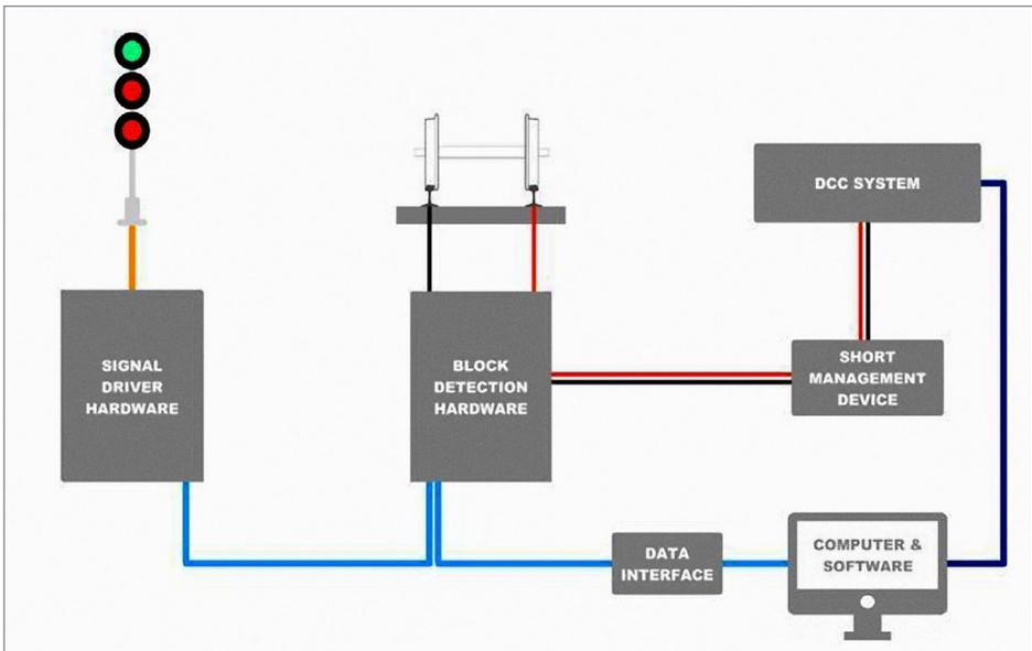
2. This diagram shows how the different parts of my signaling system relate to one another, and how they interconnect. Specific systems may vary.
