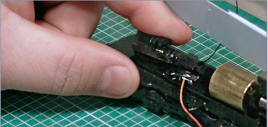
**55. Replace worm gear covers:** Snap the worm gear cover clip on. Repeat for the other truck.
