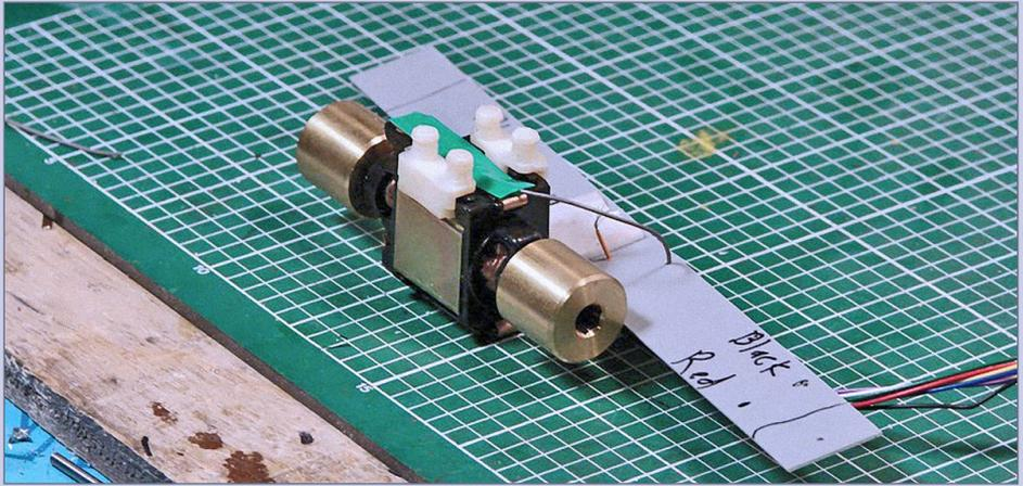
**50. Replace mounts:** Put the motor mounts back on the motor.
