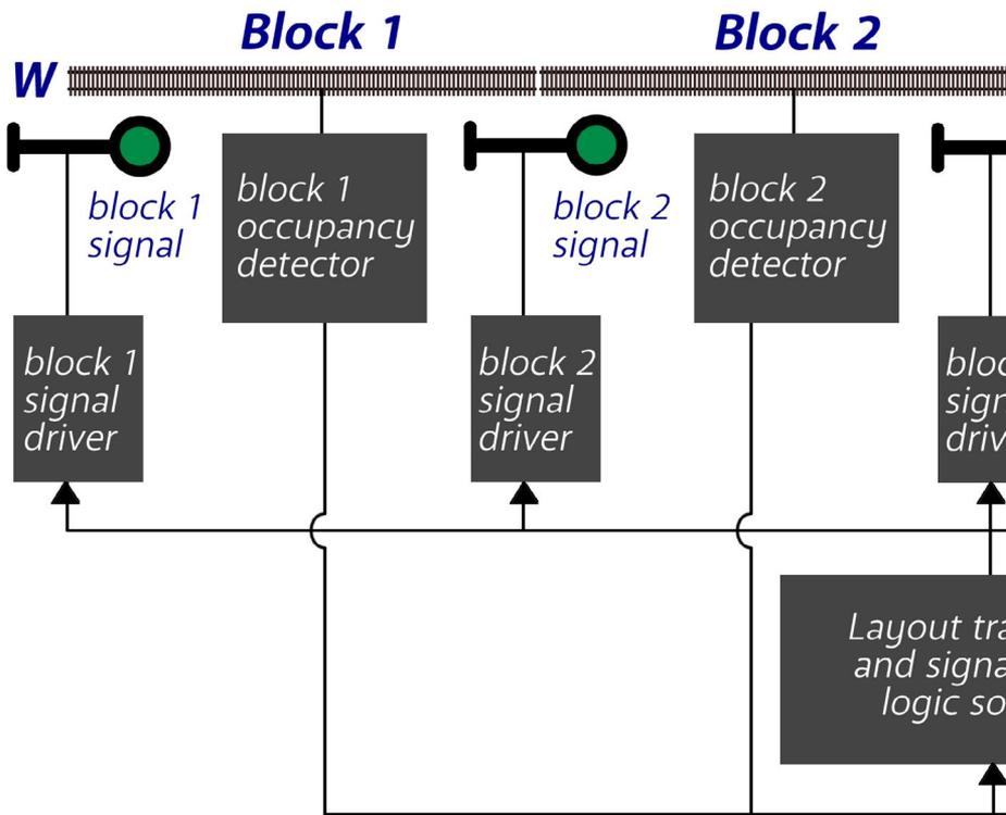
6. To make this simple four-block ABS system work for east-bound trains, these components are needed. If we also want signals for westbound trains, we will need another complete set of signals facing the opposite direction along the other
