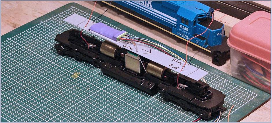
**56. Thread feeds through shield:** Thread the red and black truck wire feeds through the holes in the shield.
