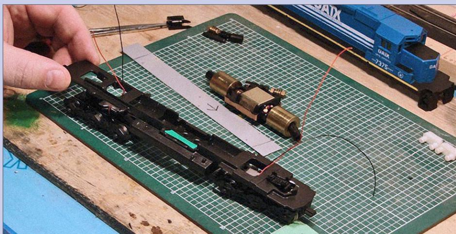
**28. Drop frame onto trucks:** Lower the frame fully down onto the trucks – first the front truck, then the rear truck.
