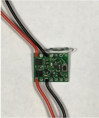
**Dead Rail Installs** is selling an on/off switch actuated by a magnetic reed. The device will control any electronic circuit and can be installed inside a locomotive, tender, or car. It can also be installed under scenery or inside a structure. The switch is turned on or off by waving a magnet near the hidden device. The unit is .6 x .6-inches square, by .7-inches high. For more information visit [deadrailinstalls.com](http://deadrailinstalls.com).
