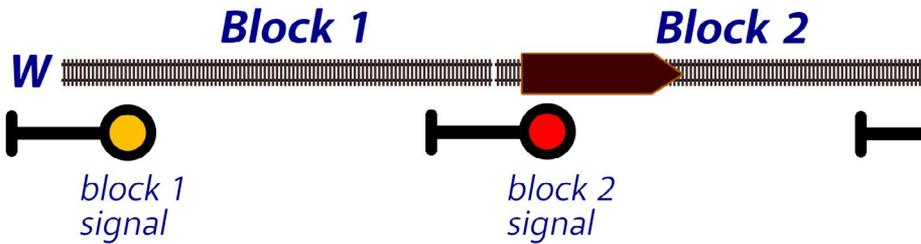
3. The eastbound train enters block 2, causing the block 2 signal to go red and the block 1 signal to go from red to yellow.
