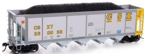
The Evolution series model is a faithful reproduction of the lightweight aluminum cars Johnstown America introduced in the 1980s to replace aging 100-ton heavy steel cars. The release was produced from corrected tooling that resulted in a more
