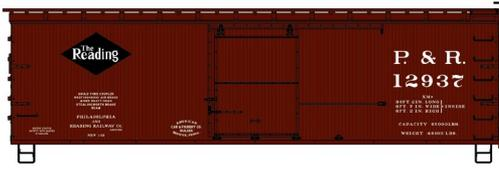
American Car & Foundry built in its Berwick, PA plant in 1913. The car features double-sheathed wood sides, wood ends,
