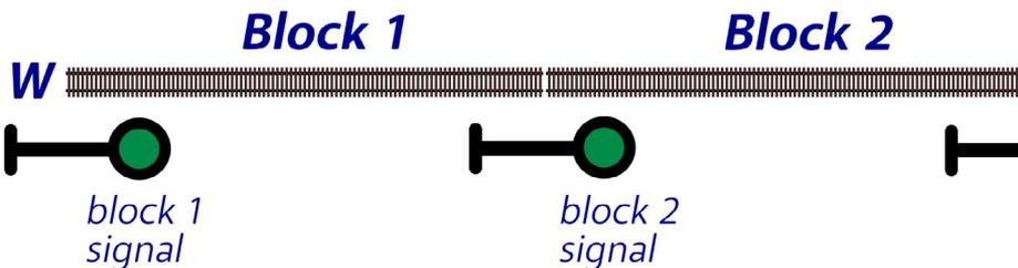
1. Four automatic block signaling blocks with eastbound signals and no trains. (For simplicity, the westbound signals on the other side of the tracks are not shown.)
