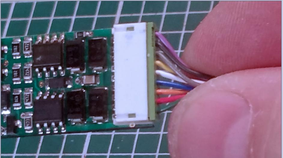
**39. Press in plug:** Press the wiring harness in place until it's firmly seated.
