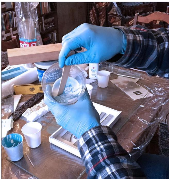
6. Then mix the two parts by *slowly and gently* stirring them together. The clear cup helps you see how thoroughly you're mixing, and the gentle stirring helps prevent bubbles from forming.
