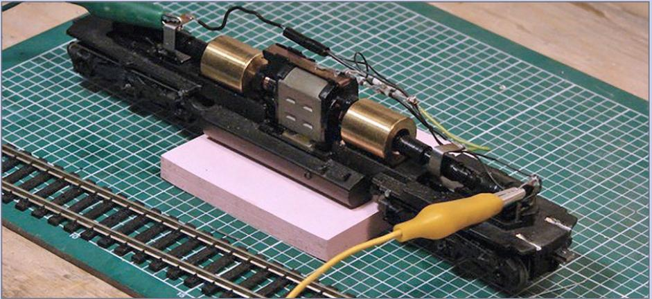
**8a. Motor contact cleaning set-up:** To clean the motor contacts, put the loco fuel tank up on something so the wheels can spin freely, and clip on test leads from a DC power pack.
