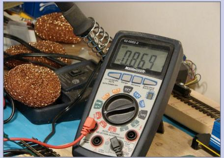
**7c. Reverse reading:** Stall current reading in reverse.
