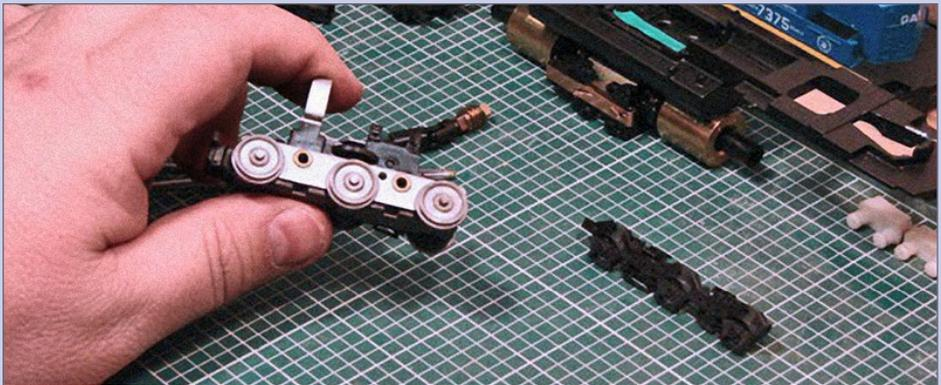
**18b. Success!** The side frame has been removed and the plastic pins are intact.
