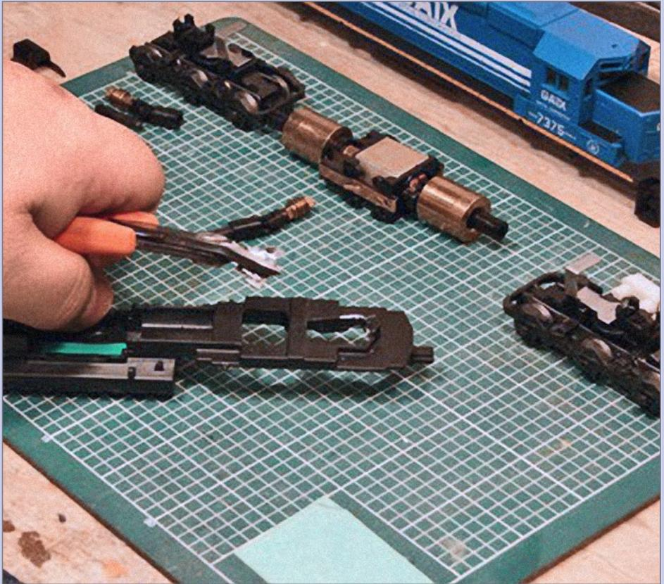
**15b. Bend until snaps free:** Bend it back and forth with pliers until it breaks loose.
