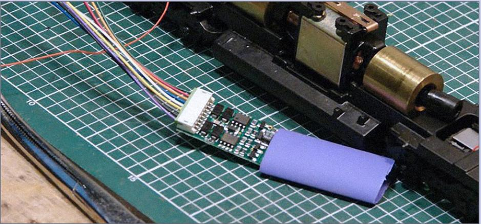
**40. Insulate decoder:** Slip the shrink tubing over the decoder.
