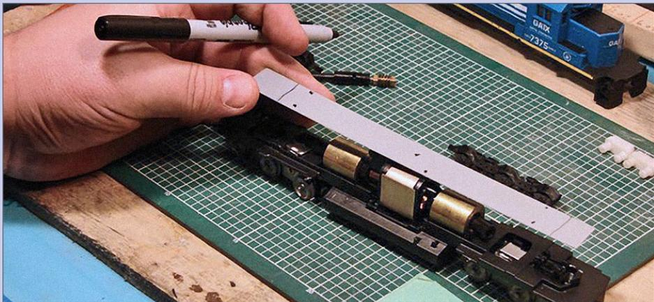
**31. Verify marks are correct:** Hold the piece up against the power chassis to verify correct positioning of the marks for the wires.
