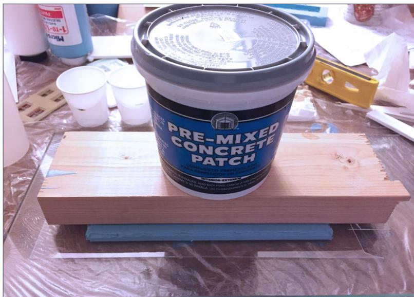
19. Lastly, weigh it all down to compress and flatten the resin. The instructions on the resin say it takes about 15-20 minutes to cure (you know it's cured when it turns from clear to white), but to be certain the casting was as hard as possible, I left it overnight.
