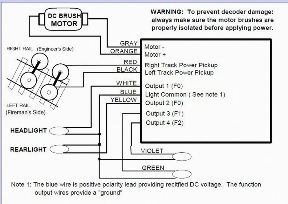
**43. Decoder wiring diagram:** Wiring instructions from the NCE D13J decoder manual.
