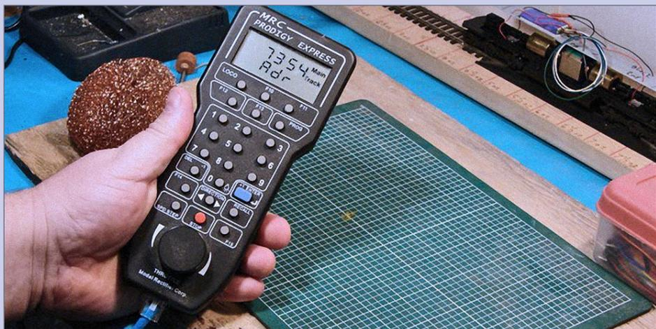
**59. Set loco address:** Having verified there are no shorts, put the loco on the programming track and set its address.
