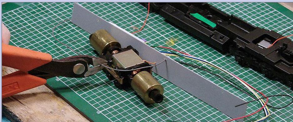
**47. Trim gray wire:** Cut the gray wire so it is long enough to reach the bottom of the motor.
