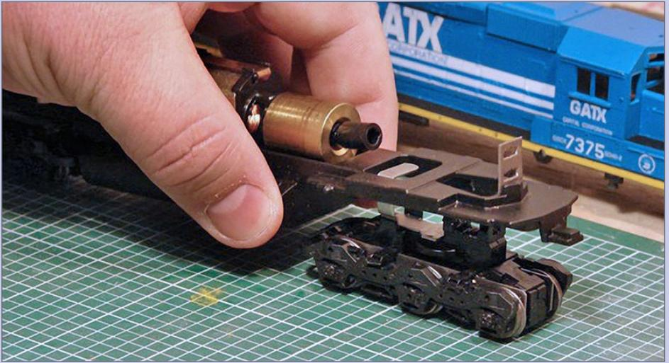
**12a. Remove trucks:** To remove a truck, lift the frame.
