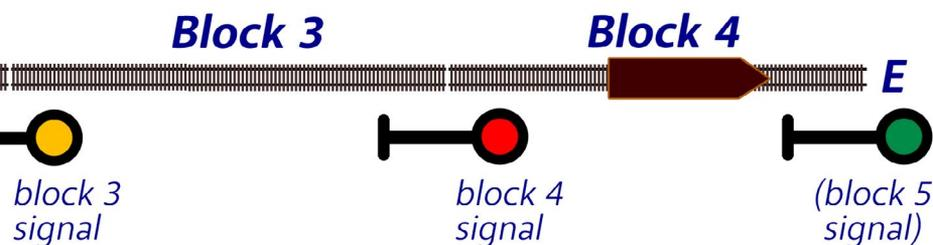
Since most model railroad track is already powered, detection of a locomotive is easy: we can just add a current sensing circuit to determine if current is flowing across the rails.
