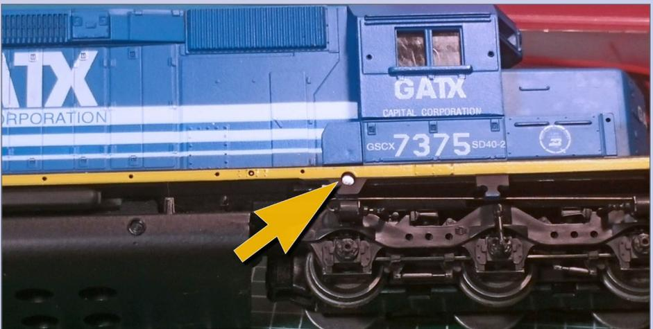
**3a, 3b. Finding shell retainer pins:** Shell side retainers are used on many Blue Box locos.
