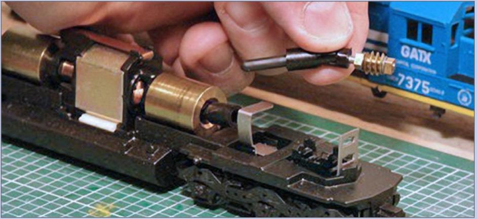
**11c. Set aside worm gear and shaft:** Pull the shaft out of the coupler on the flywheel and carefully set the worm gear assembly aside. Be careful not to lose any of these parts!
