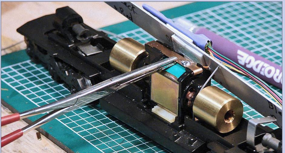
**52. Solder orange wire:** Solder the orange wire to the top motor clip. Note the double-stick foam tape applied to the underside of the shield.
