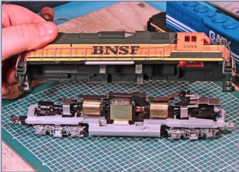
**5a, b, c. Removing shell with bottom pins:** To remove a shell which has the bottom internal retainers, grip the fuel tank, and gently squeeze and rock the body until it comes off.
