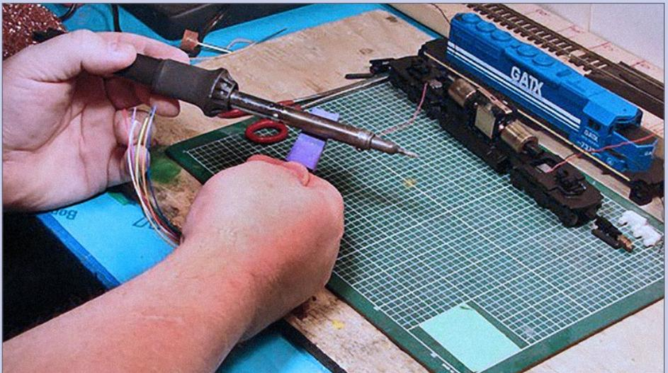
**42. Shrink tubing (soldering iron):** Alternatively, you can shrink the tubing by gently whipping it against the barrel of a hot soldering iron.
