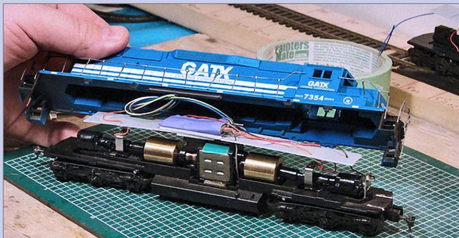
**61. Tidy up:** Tidy up any loose wires and gently place the shell onto the body, making sure to keep any wires from getting pinched between the shell, shield, and the frame.
