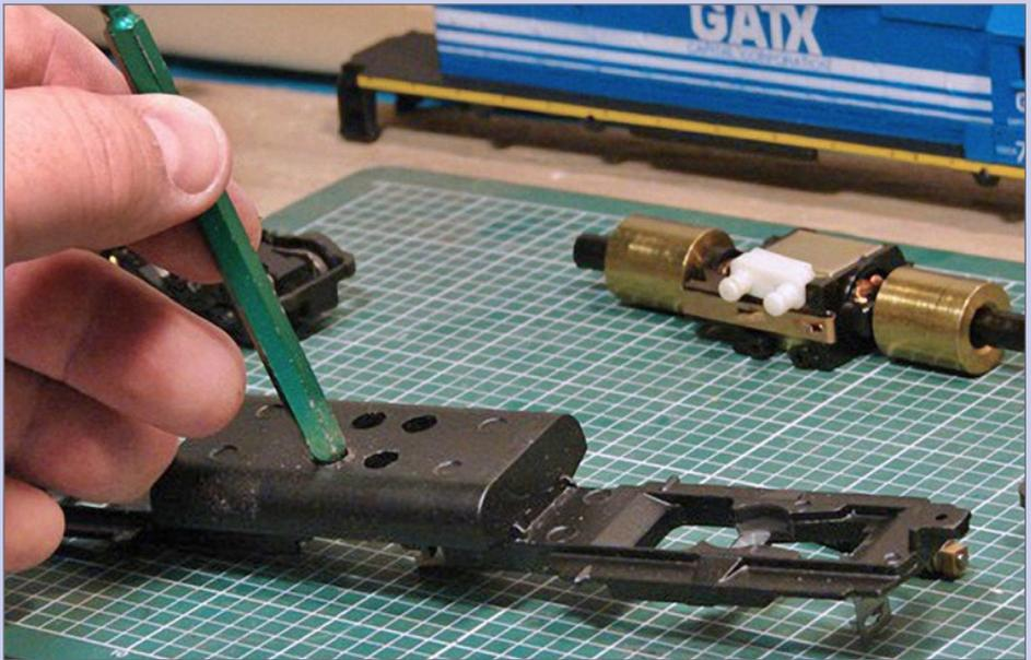
**14c. Poke other mount free:** Use a pencil or pen to press on the motor mount through the holes until the mount pops free.
