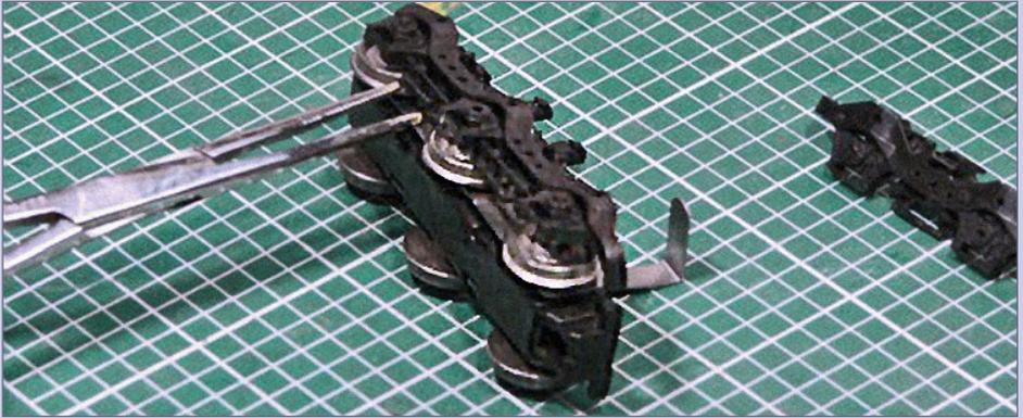
**18a. Remove truck sideframes:** Using a locking hobby clamp (hemostat), gently pry up with even pressure while pulling the side frame away from the truck.
