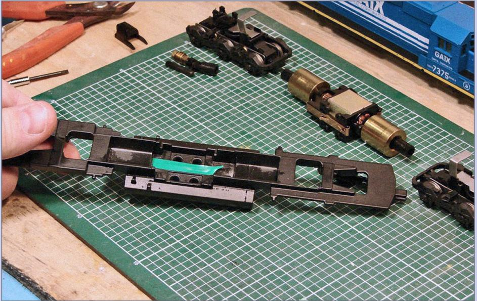
**17. Tape the frame:** Apply insulating tape to the frame at the shiny motor contact area to isolate the frame electrically.
