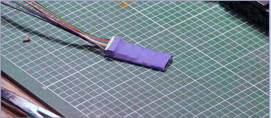
**41. Shrink tubing (heat gun):** Heat the shrink tubing carefully with a heat gun to shrink it up.
