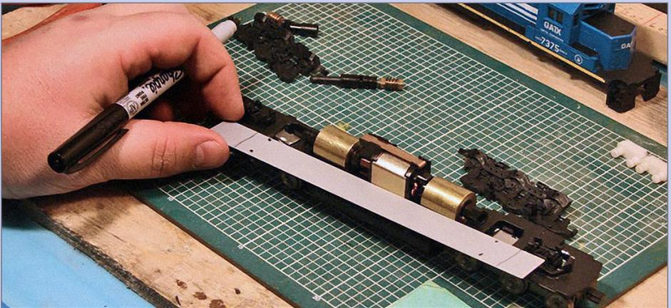
**30. Mark wire locations:** Mark the spots for the wires – two on each end for the truck wires and two over the motor for the motor wire feeds.
