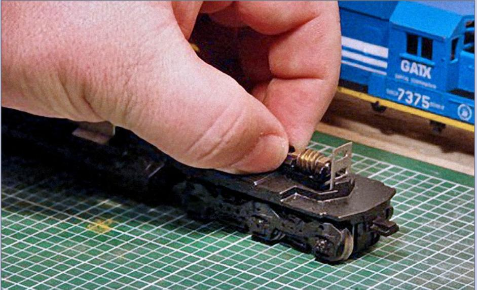
**11b. Remove worm gear:** Once the worm gear cover clips are removed, lift out the worm gear and its block mounts.
