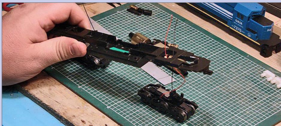
**27. Thread leads through frame:** Starting with the front truck, thread the new feeder wires into the hole closest to the fuel tank. Repeat for the rear truck.
