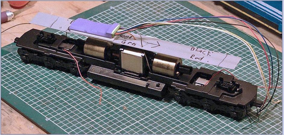
**53. Test fit shield:** Without taking the backing paper off the foam tape, check the fit by temporarily positioning the shield on top of the motor.
