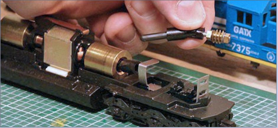
**11c. Set aside worm gear and shaft:** Pull the shaft out of the coupler on the flywheel and carefully set the worm gear assembly aside. Be careful not to lose any of these parts!
