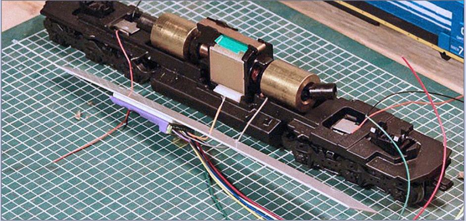
**51. Reinstall motor:** Install the motor back into the loco frame.
