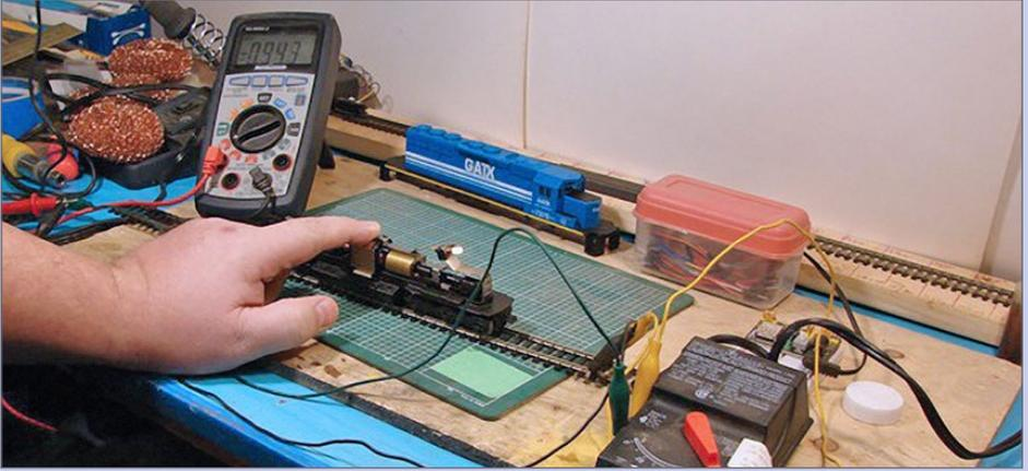
**7a. Current-draw test set-up:** Here is my set-up for testing current draw, with a power source and a multimeter.
