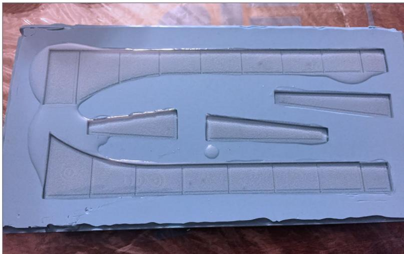
17. As before, I mixed equal parts of A and B together in a clear cup, then slowly poured the resin into the mold, doing my best to avoid bubbles. And – important (as I discovered later) – be sure to “overfill” the mold slightly. This is where making sure your foamcore box and mold are perfectly level pays off. And be sure you’ve put down some plastic to protect your workbench and catch any resin overflow.
