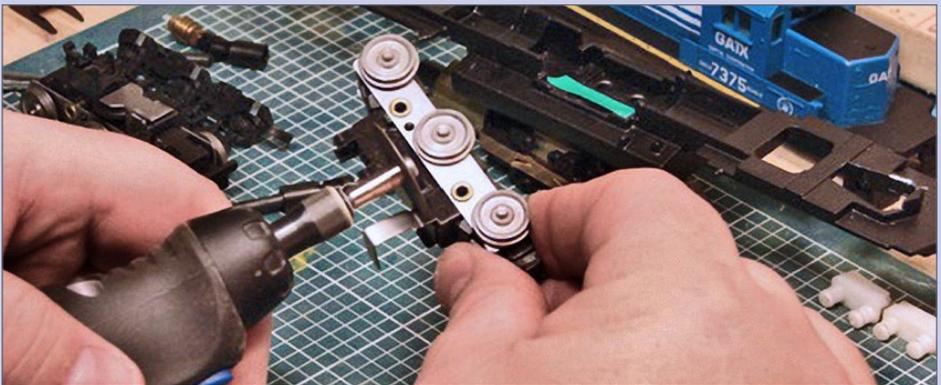
**19. Cut off L bracket:** Use a motor tool with a cutoff disk to cut the metal L bracket off the truck.
