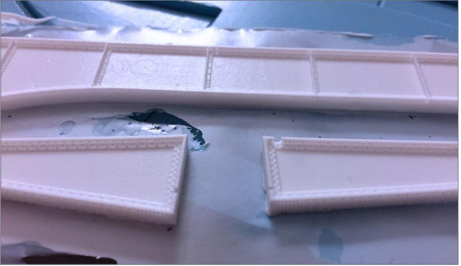
21. Unfortunately, there must have been some bubbling along a few of the girder edges. You can see above what look like “chips” that broke off. Nope – that’s how the casting came out. This should be a relatively simple matter of filling them in with either putty or strip styrene, but I might not even bother, since these castings will be painted black and put under a bridge next to the backdrop.
