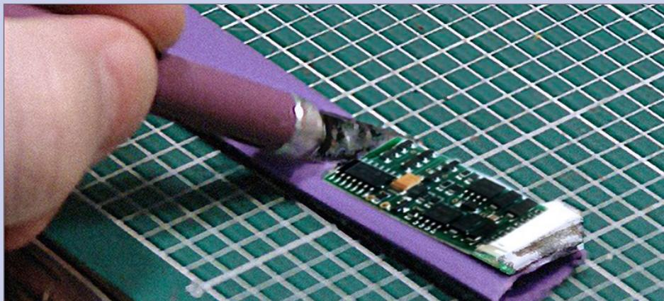
**37. Cut 1/2" shrink tubing:** Using the decoder as a guide, cut some 1/2" shrink tubing to length.
