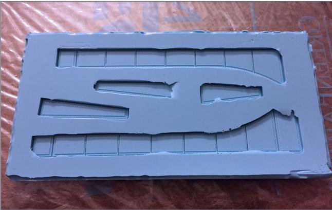
14. The box broke away fairly easily, and I was able to peel the mold away. Not too bad – but I still got some seepage of rubber underneath the masters, despite running a bead of glue around the perimeter of each part. Next time, I'll make sure that the glue seeps out just a little around the edges – that should seal things nicely.
