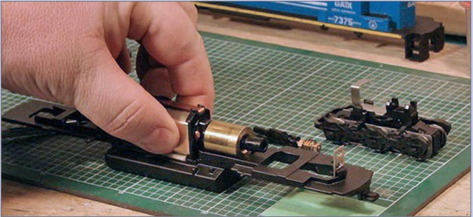
**13a. Remove motor:** To remove the motor, gently rock it from side to side, working the motor mount free.
