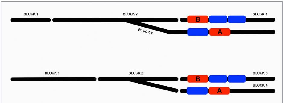
9. Here is an example of how breaking up junctions and turnouts into their own blocks helps streamline traffic flow. On the top diagram, train B is blocked by train A because the turnout is part of block 2. In the lower diagram, putting the turnout into its own block allows train B to move.
