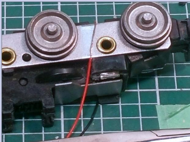
**23. Tinned power lead placement:** Place the tinned wire on the truck's metal plate as shown.
