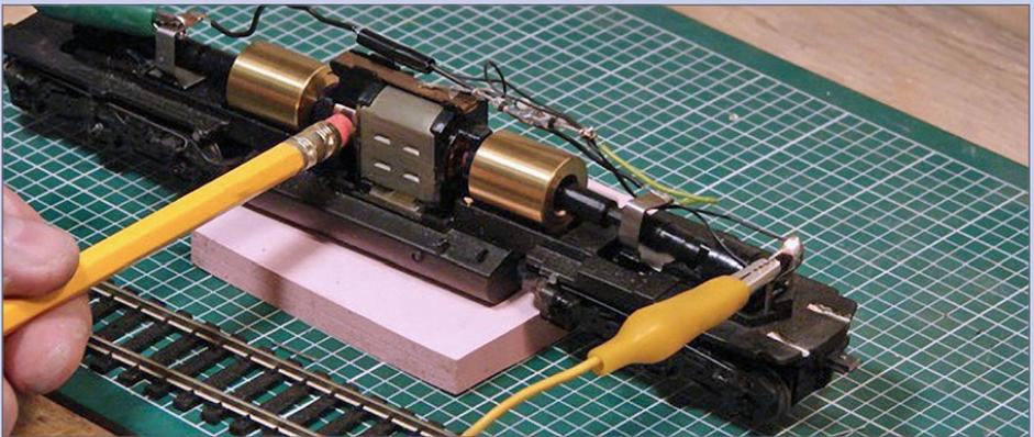
**8b. Clean motor contacts with pencil eraser:** Turn up the DC power to a good speed, then take a pencil with a soft pink eraser and hold it against the motor contacts (commutator) as it spins to clean off built-up carbon.
