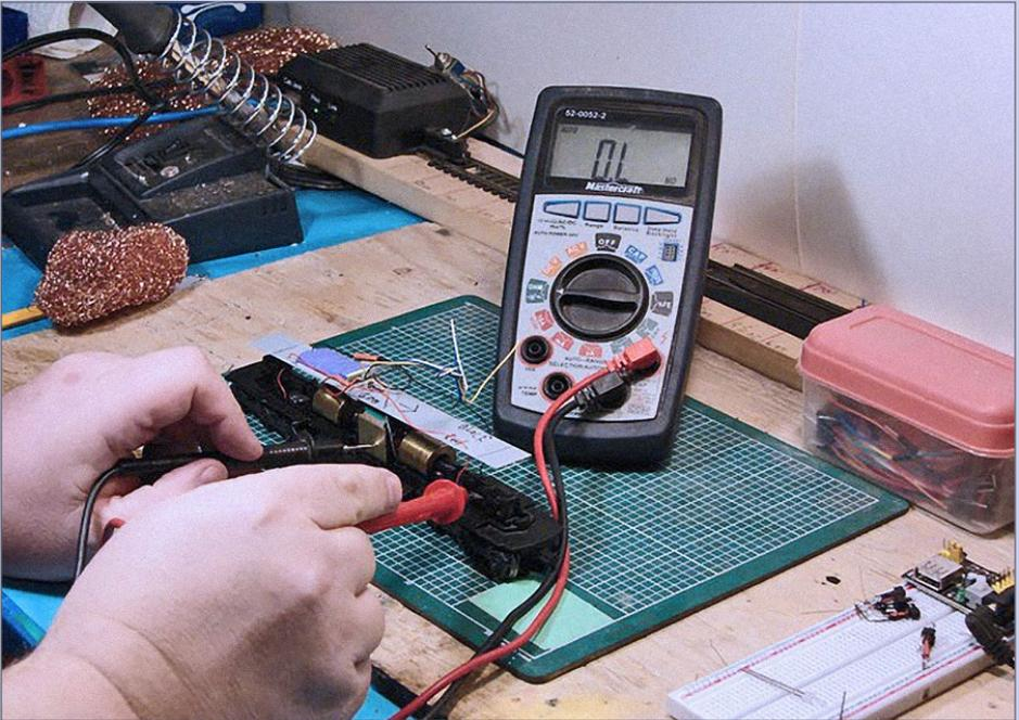
**58. Test for shorts:** Using the connectivity setting on a multimeter, check for shorts between the wheels and the motor housing, as well as between the wheels on the left and right sides.
