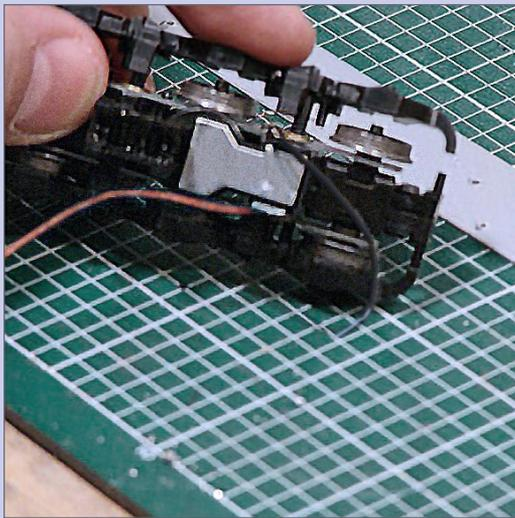
**25. Reinstall side-frames:** Put the side frames back onto the truck by pressing the pins down into their respective holes. Avoid pinching the feed wires with the side frame.
