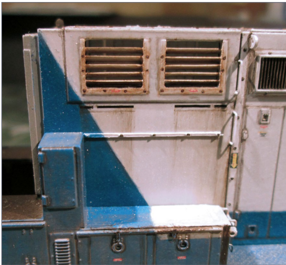
57. Location of the batten-and-bolts strip above the A/C unit (A/C unit temporarily removed).
