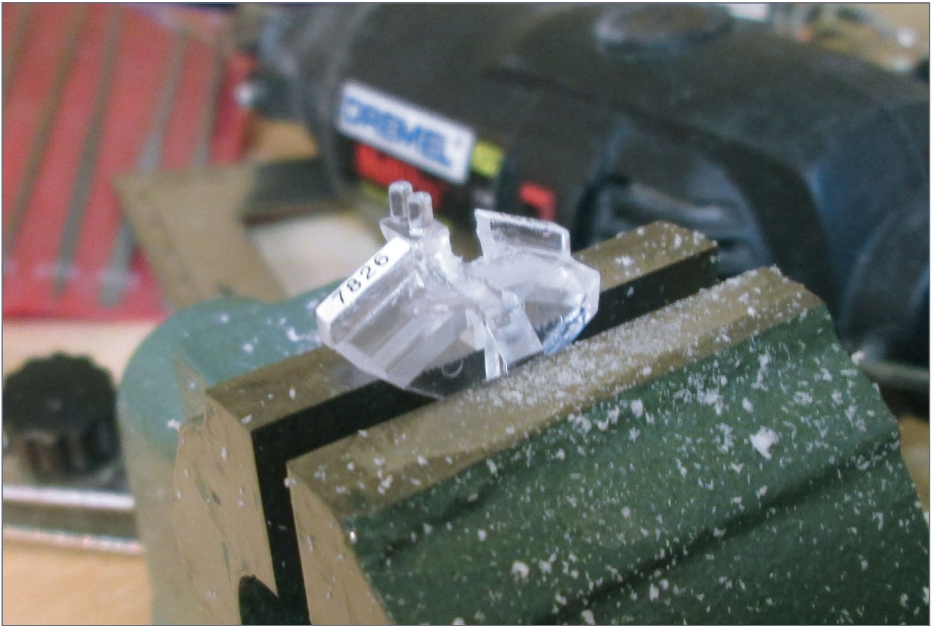
56. Filing the light casting to get it to fit.
