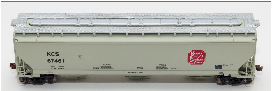
15. KCS 67461 from overhead, showing off the metal-style roof hatches and plastic roof walk.
