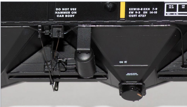
21. DCBX 2065, closeup of brake piping, air tank, and discharge hatch.
