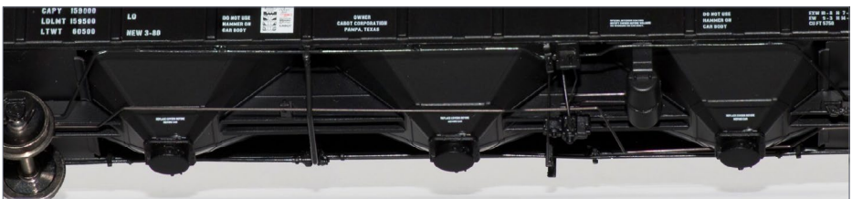
29. CABX 580772, Hopper and brake piping details.
