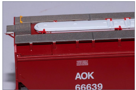
6. AOK 66639, Detail view of fiberglass roof hatches.
