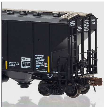
38. DCBX 2065 N scale Thrall 4727 cu. ft. carbon black covered hopper, B end detail.
