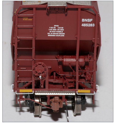
4. BNSF 485283, Detail view of B end with brake equipment details.
