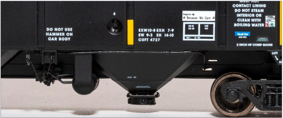
25. DCBX 2065, detail of hopper bin and COTS stencil.
