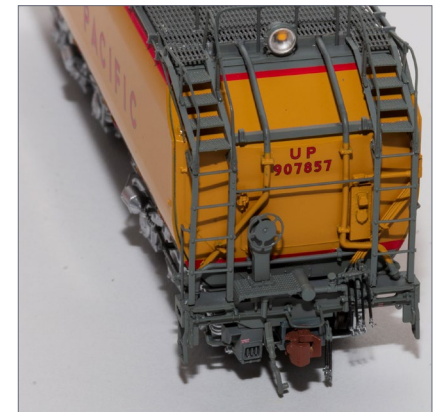
51. UP water car 907857, B end detail view.
