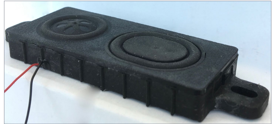
10. Tang Band TO-2008S speaker module will provide amazing sound in places where it will fit. If you have more space, larger versions are available. The speaker is the round item on the left in this photo. The oval is the passive radiator, which has more cone area than the speaker.
