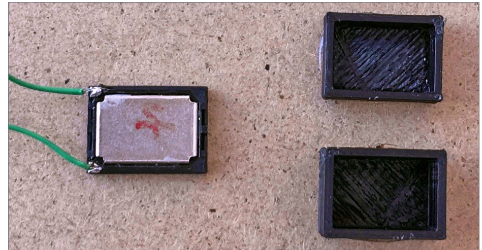
2. Litchfield Station SP-13x18-04 speaker with 12mm and 6mm high enclosures.
