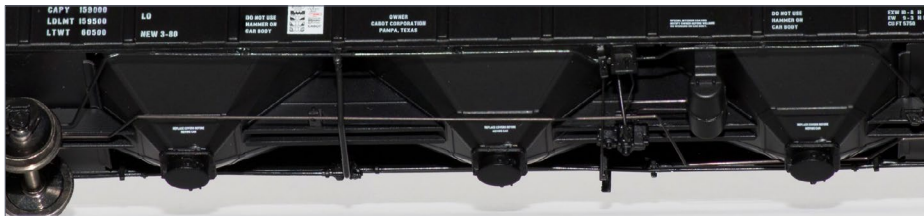
29. CABX 580772, Hopper and brake piping details.
