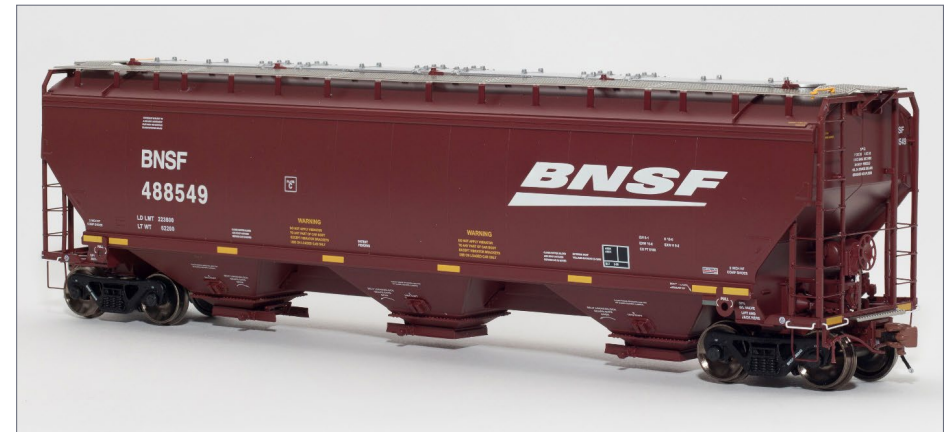
9. BNSF 488549, Version 3 body, equal-width intermediate panels, roping eyes mounted to the side sills of the car body.
