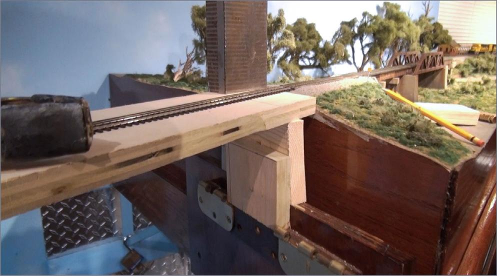
4. I test-fit the wood section into place and used 1x4 pine as a riser, placing it atop my existing woodwork. This made the track line up perfectly with regards to rail height. I used another piece of 1x4 lumber, centered between the door hinges, to make a lap joint to prevent the section moving. I did this to each end of the lift-out, gluing and clamping the unfinished wood together.
