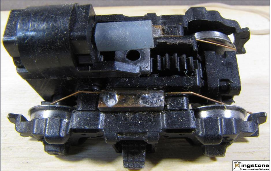
5. Adding wheel wipers to a loco such as those shown here adds an alternate electrical path directly from the wheels and bypasses the sometimes weak wheel-to-axle-to-metal-plate path. Adding a wire from the wiper PC board to the loco motor PC board or decoder also improves reliability by providing a second path for the electrical current. *Photo by Bernd Fanghanel*
