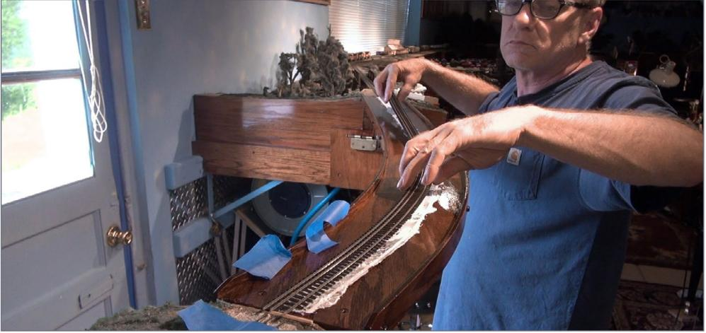
10. I soldered together two 3-foot pieces of flex track. I carefully bent this to match the flow through the scene, then glued the track in place with DAP Quick Seal flexible adhesive applied with a painter's knife. I pressed the track into this glue, carefully matching the ends to the existing track and let this dry for about 2 hours.
