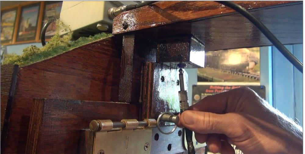
13. The wood box was glued up under the lift-out section. The male microphone jack simply plugs in, providing track power to the section.
