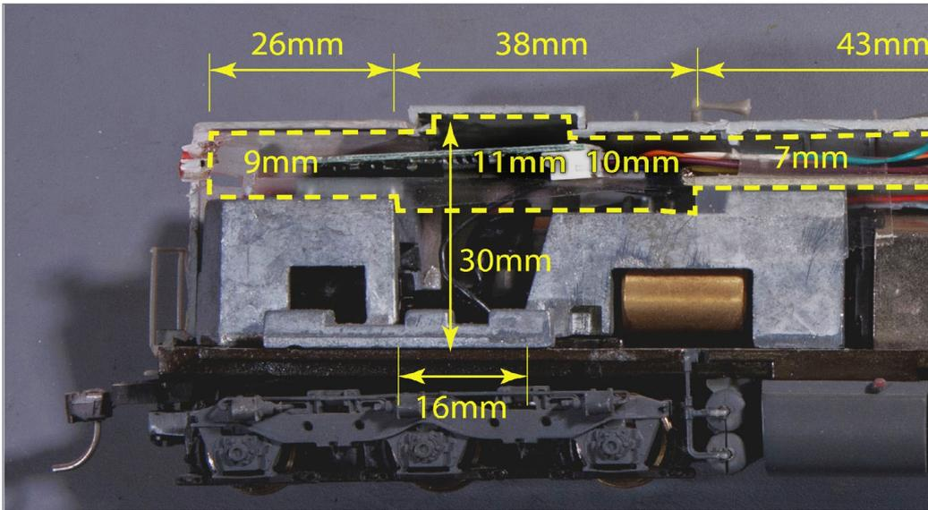
9. To give you an idea of the space typically available inside an HO diesel loco, here is a cross-section of a Proto-2000 SD9. This loco is actually fairly roomy above the motor and weights. Some locos
