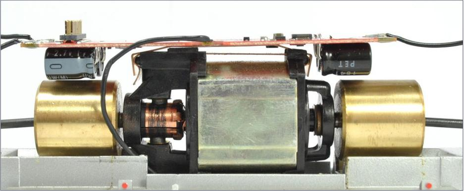
13. Example of how a TCS Keep-Alive® motherboard replacement locates the capacitors in otherwise dead space over the flywheels. This clever trick allows fitting stay-alive into locos more easily. *Photo by Train Control Systems*
