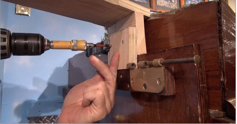
5. I used wood screws to join the lap joint and attach the  $\frac{3}{4}$ -inch plywood to the 1x4 riser. I then drilled two  $\frac{3}{8}$ -inch diameter holes in the 1x4 and the existing stained plywood, about 3 inches apart.
