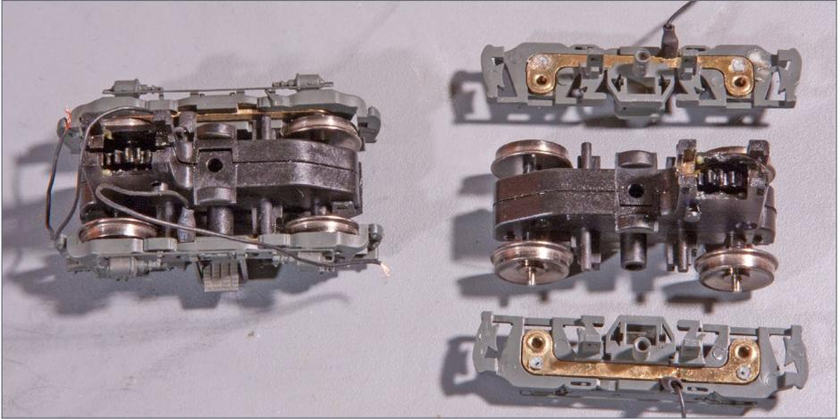
6. Many modern HO diesel trucks have metal plates in the side frames like you see here. The electrical contact point becomes the wheel axle tip through a hole in the metal plate. The reliability of the electrical path depends on how much slop exists between the axle tip and the hole.
