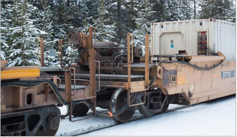
3. Connections between cars and the generator-set container. While the containers are on the train they are powered by the genset. Once they are off, other power sources are used. *Andrew Hall photo*
