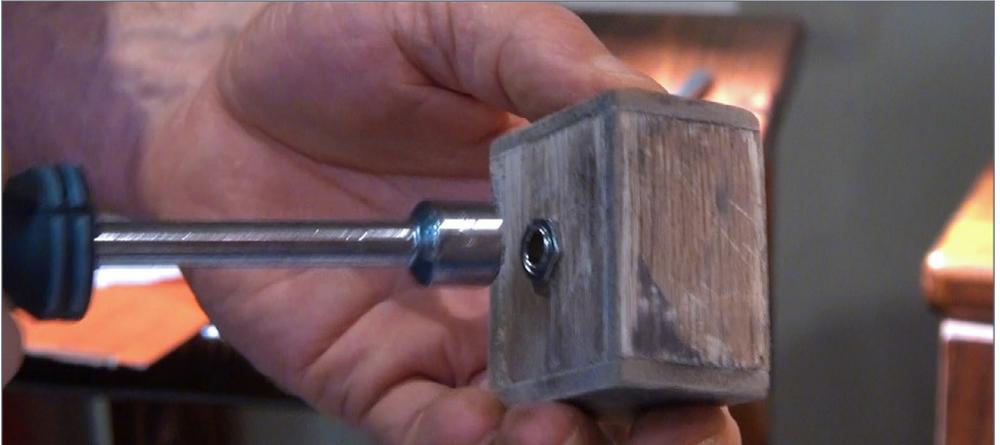
11. While the track glue cured, I built a small wood box from scrap pieces of  $\frac{1}{4}$ -inch oak. I then drilled a hole in the box to accept a 2-conductor microphone female jack.
