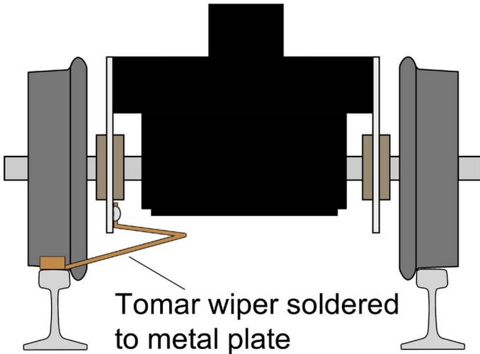
4. I added the Tomar wiper to the blue-box Athearn loco by folding it and soldering it to a truck's metal plate as shown. By adjusting the V-bend angle, I can control how much tension the wiper puts on the rail.
