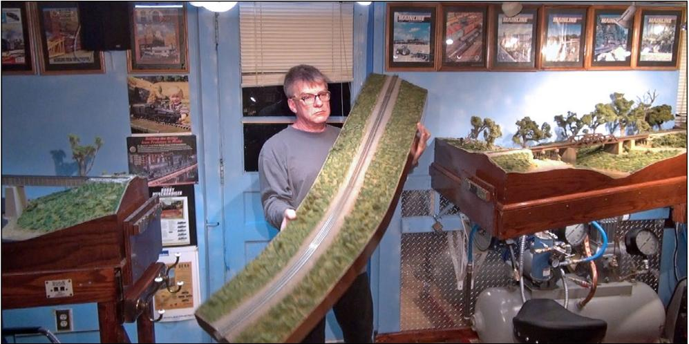
1. (Above) I wanted to replace this foam lift-out section on my layout with a simpler design that would be 5 inches wide rather than 13 inches, and have a 3-inch higher clearance, making it easier to duck under. I figured it could be made from simple plywood. I started by removing the old lift-out section. It was held in place by door hinges and pins, so I pulled out the hinge pins and removed the section by lifting it up and unplugging the 2-conductor microphone jack.
