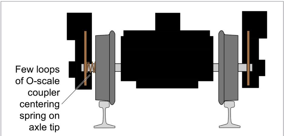
7. To improve power pickup on locos that rely on axle-tip-to-side frame contact, put a few loops of an O-scale coupler centering spring on each axle tip. Don't overdo it, though, or you'll start to create extra drag and limit your loco's pulling power. Just a few loops with minimal pressure guarantee a current path between the wheels and the side frames.
