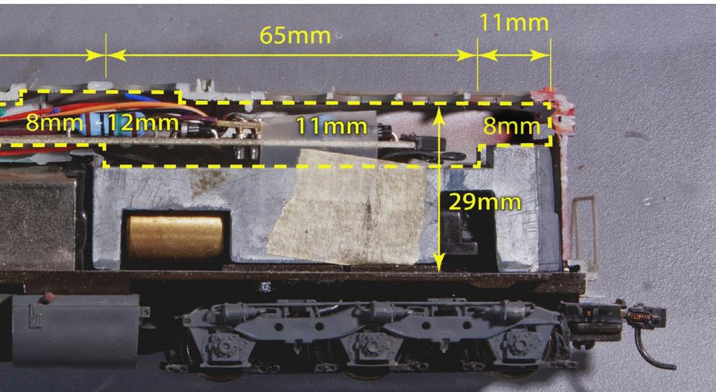
average closer to 6mm above the motor and weights. Older Bachmann diesels have even less space, with the weight taking all but a few millimeters of the space inside the top of the shell.
