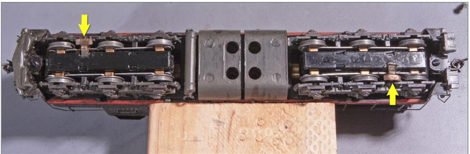
2. Adding Tomar phosphor-bronze railhead sliders (yellow arrows) to this blue-box Athearn loco makes it extremely sure-footed when it comes to electrical pickup. Note the old-style sintered metal wheels are not particularly clean, yet the loco still runs without stalling!
