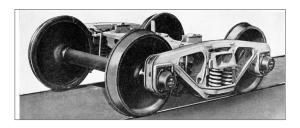
ted with Hyatt roller bearing assemblies. Note the plankless spring base.
