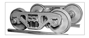
ing journal allows a controlled amount of lateral movement of the axle. The three axle bolts are surrounded by a round end cap.
