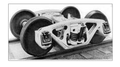
tive shock absorber. Although the Chrysler FR-5 truck rode well, its high initial cost and heavier-than-normal maintenance limited its acceptance.
