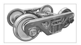
61. Also popular is the ASF100-ton Ride Control truck. This photo clearly shows the inverted U-shaped jaws on the cast side frame that the hold
