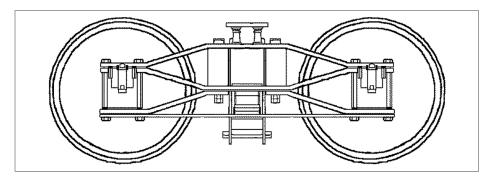
4. Some early trucks were fabricated with four bars. MCB named it the auxiliary arch bar (third from the top).
