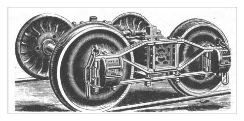
1. Thielsen arch bar trucks were popular from 1875 to the early 1900s. It featured a cast iron transom. This one is equipped with safety chains, indicating it was for a tender. In 1884 the Master Car Builders (MCB) standardized the wheelbase of arch bar trucks at five feet.
