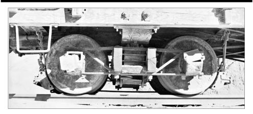
2. The principal drawback with arch bar trucks was that over time the rivets and bolts that held the side frames together tended to loosen, often with disastrous results. This well-traveled arch bar truck has a straight upper chord and swing hangers between parallel wood transoms.
