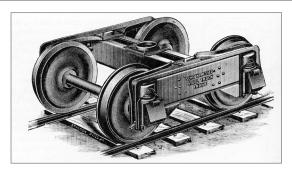
dropped the Schoen design but continued producing the Fox truck. As trains grew in size, weight and speed, the lack of flexibility in stamped metal trucks and the tendency for the journal to jam in the spring pedestal spelled their demise.
