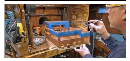
6. I painted the building's cement cap stones with an airbrush and Floquil Cement paint. The air pressure was set at 10 psi to spray a very tight and fine pattern with no overspray. This will accent the outside lines of the building for a realistic appearance.
