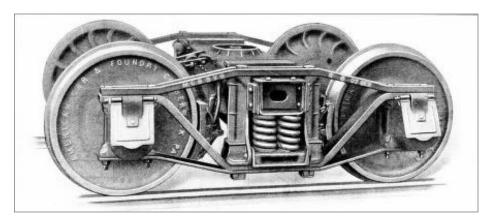
3. From the late 1800s through the 1920s, the American Car & Foundry Company (ACF) produced arch bar trucks for 30- to 50-ton capacity cars. This one is for a 40-ton car. The MCB defined the bars of the frame as the arch bar (top), the inverted arch bar (middle), and the pedestal tie bar (bottom).
