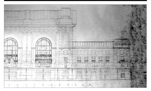
2. Here is a photograph of the right side of the drawing. The entire drawing is over 8 feet long. In the left-hand window in the middle of the decorative masonry at the bottom of the window is a lion head. I faithfully re-created this in my CAD drawing. Later I learned the important difference between "as drawn" and "as built." There was no lion head on the prototype!
