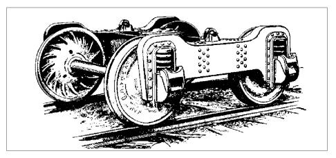
8. Trucks with stamped metal side frames were introduced in an attempt to overcome the inherent problems of the arch bar concept. Several designs were offered, with the most successful being the Fox truck with stamped side frames riveted together to form a rigid truck. Fox was an established British company that sold its products throughout Europe. It met considerable resistance to its products in the U.S.
