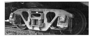
include the arched upper corners and deep section below the spring plank.
