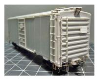
RSW's mini-kit consists of a pair of cast resin ends, a sheet of Chicago Great Western decals, and a pair of Tahoe truck side frames. The master for the proprietary P-S ends was created by Jason Kliewer and printed as a 3D solid model. They were cleaned up and used to make molds to cast these
