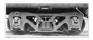
47. Symington-Gould's XL series of high-speed trucks featured pedestal style journal boxes with unique bottom retainers that allowed lateral axle movement
