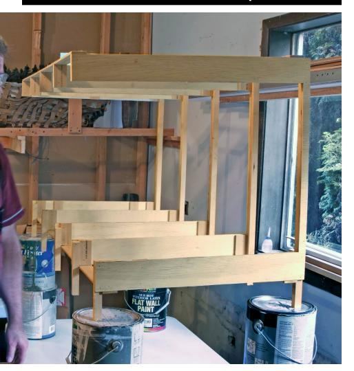
16. I built a 44" long prototype module section out of ¼" plywood and some ¾" square stock cut on my table saw to test my module construction ideas. The module shown here has the base track level at 50" off the floor (I stacked paint cans on the work table to get it up to the right height) and it weighs a mere 5 pounds. Compare this to the 3D digital render I did in SketchUp [11]. This section still needs the fascia, valance and backdrop added, but so far the results are very promising.
