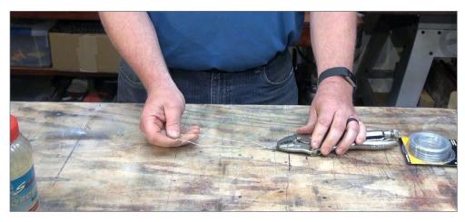
21. He starts with a picture frame wire bent in an 8-inch-long 'U' pattern.
