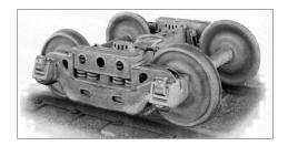
52. The Commonwealth equalized, high-speed, swingmotion, pedestal-type trucks, produced by General Steel Casting Co., employed both coil and full-elliptical springs.
