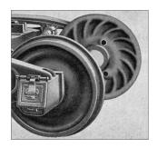
83. Wrought steel wheels, which had a much better safety record than cast iron, were specified for new passenger equipment in the 1920s. Although more expensive, wrought steel wheels were considered far safer. The application of wrought steel wheels on freight trucks started selectively in the early 1930s and became widespread after World War II.
