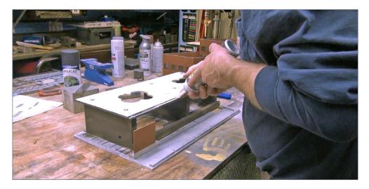
9. The interior frame of the building is made from wood and painted to seal it. I am applying a bead of silicone adhesive to the second story lip as well as the entire base around the bottom.
