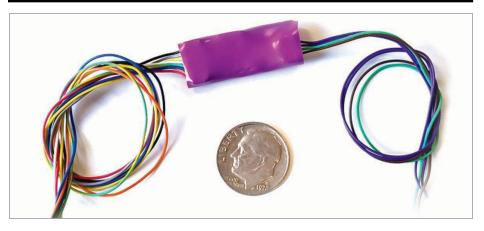
3. The TSU-1100 replaces the TSU-750 and provides 1-amp motor current and four functions.
