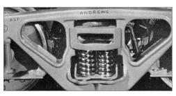
spring planks were made of wood [2]. Metal spring planks (above) were made of a wide U-shaped channel.
