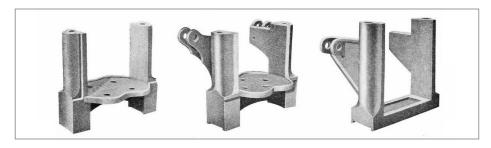
6. Cast spring seats and bolster column guides for arch bar trucks were offered by several companies. These are from American Steel Foundry (ASF).
