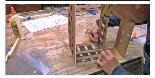
8. For the glass in the building I used 1/32" clear plastic sheets cut to the size of the entire wall, covering the windows. This was glued in place with clear silicone adhesive. I did this for all the windows as it was fast and added strength to the walls.
