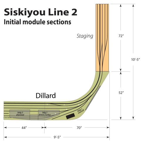
8. I'm planning to start construction of SL2 with these two module sections and follow TOMA practice by getting them finished before moving on to other sections. I'm adding some minimal staging on one end for use with these two sections as I'm hoping to take what you see here to the Kansas City NMRA National train show in August.
