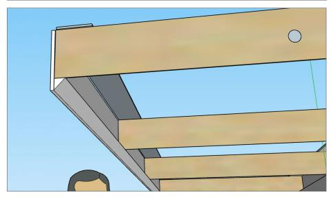
14. Adding a triangular strip to the valance makes it easy to add LED strip lighting to the module.
