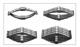
weight of the car single, dual, triple, and quadruple elliptic groups were used.
