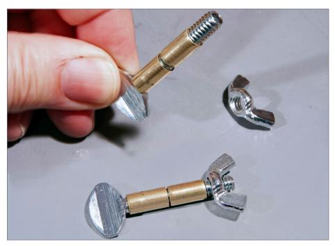
12. To connect the module sections, I'm using  $\frac{1}{4}$ " x 1- $\frac{1}{2}$ " thumb screw bolts with wing nuts. I'm also lining the holes in the wood module ends with 9/32" brass tubing that has a tight sliding fit over the  $\frac{1}{4}$ " bolts.
