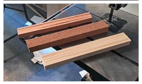
13. I tested different materials for making spline (from top to bottom):  $\frac{5}{16}$ " pine,  $\frac{1}{4}$ " Masonite, and  $\frac{1}{4}$ " poplar. I was looking for which material weighed the least – and pine was the hands down winner, being only 36% the weight of Masonite.
