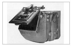
5. Cast journal boxes surrounded the end of the axle, held the bearing in place, and provided a small reservoir for lubricant. The spring-loaded lids could be flipped up to view the bearing and add oil if needed.
