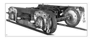
tals bolted to a cast steel frame. This truck was produced by General Steel Casting Company.
