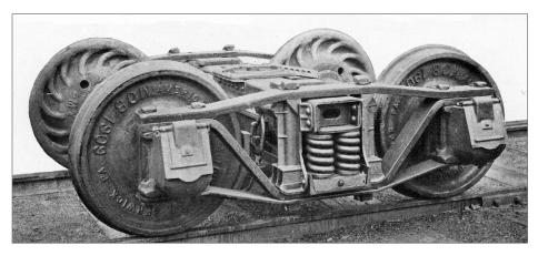
7a. This arch bar truck with large journal boxes is rated for a 50-ton capacity car. Upper and lower arch bars are 1.5 inches thick by 5 inches wide; the tie bar at bottom is 0.625 inches thick.
