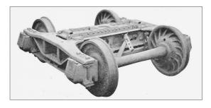
stamped bolster that was riveted to the stamped upper arch bars. It garnered little interest. Freight car trucks take a beating, and with the myriad of parts in a pressed metal truck, too many things could go wrong. A better idea was needed.
