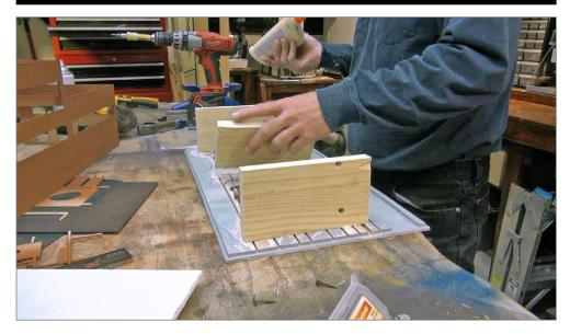
5. The first-floor plywood base warped, with a 1/8th-inch bow as the primer dried in the sun. I scored the base with a saw to bend it straight and replaced the half-inch wood columns with 5-inch-high half-inch stock. This will prevent further warping and support the second floor in the right position to fit the building's window arrangement.
