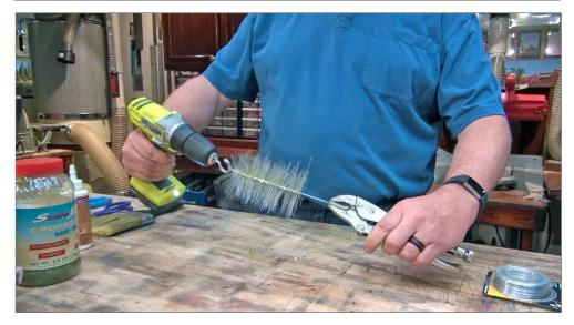
24. When the drill is turned on, the wire twists the brush fibers into instant tree branches. It happens very fast and is cool to watch in the video.
