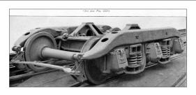
favored bolted-on journals, since a broken one could be easily replaced without junking the expensive main frame. This truck was built in the early 1930s.
