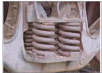
As freight train speeds increased in the 1920s and '30s, it was found that trucks with springs that cushioned loaded cars rode extremely hard when empty, sometimes setting up oscillating harmonics that caused the trucks to bounce dangerously. Various types of snubbers were developed to help mitigate the oscillations.
