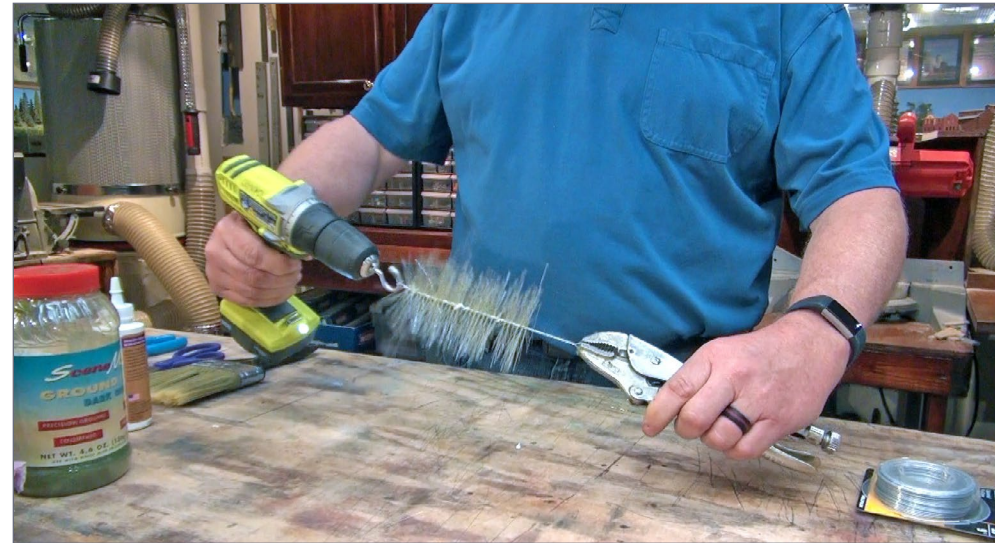
24. When the drill is turned on, the wire twists the brush fibers into instant tree branches. It happens very fast and is cool to watch in the video.
