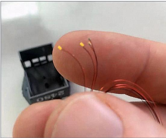
6. Note how tiny these micro LEDs are.
