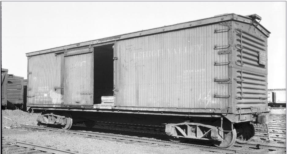
29. Note that the car, although rebuilt with many new all-steel body elements, retains its original arch bar trucks. *DL&W company photo, Steamtown NPS collection*
