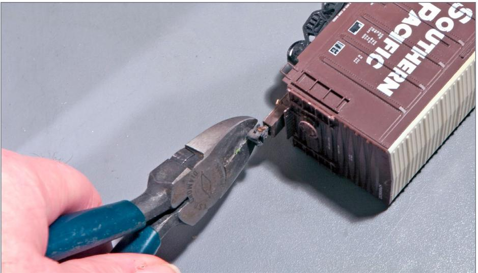
2. Don't use wire cutters to cut off Kadee coupler trip pins. The hard metal Kadee uses will damage the tool's cutting faces. Use a motor tool and cutoff disc instead.
