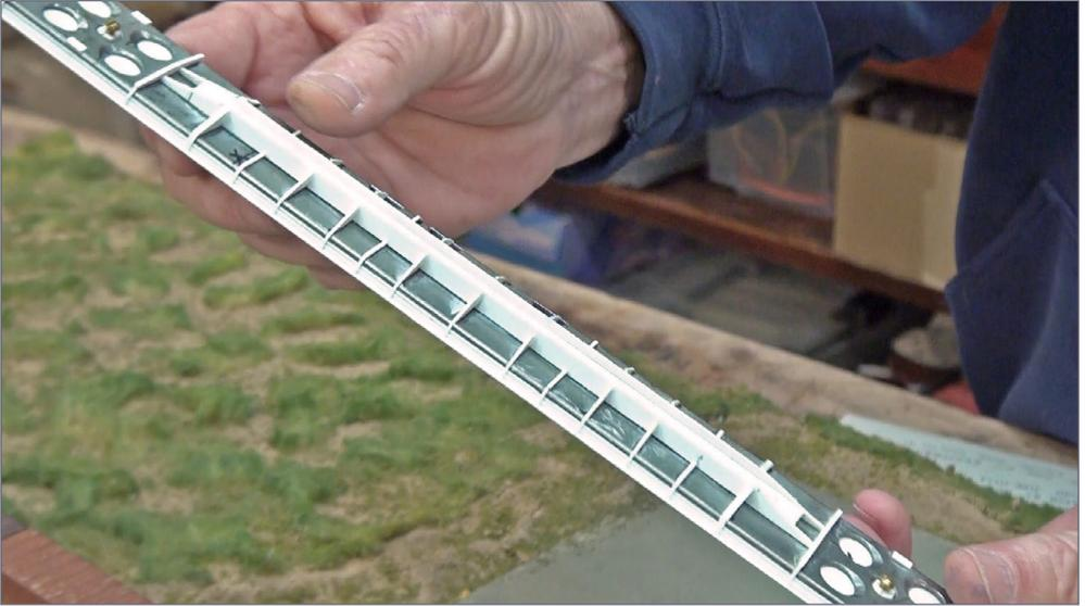
17. Mike built each car from scratch, starting with an Accurail flat car weight and building styrene shapes and ribs until he had a close resemblance to the prototype cars.
