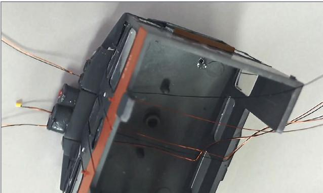
**7. Thread the LED leads through the light housing holes. Leave the LEDs sticking out by at least 5mm (1/4 inch).**
