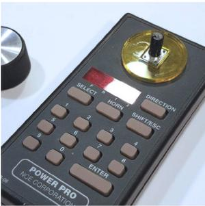
**The Cab Saver** has introduced Cab Savers, plastic disks with square holes in them sized to eliminate free play and rocking in the knob of potentiometer equipped NCE Cab06P and Cab04P throttles. Available in 16 different colors, the Cab Savers fit against the throttle underneath the knob, filling the space between the
