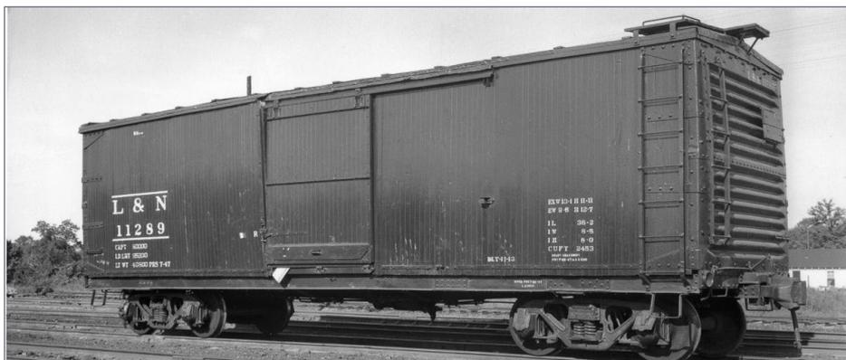
17. L&N 11289 poses for a photo in late 1947, soon after being repainted. This photo was probably taken as an insurance photo; the light splotch to the upper left corner of the door shows that the car body has broken in two!
