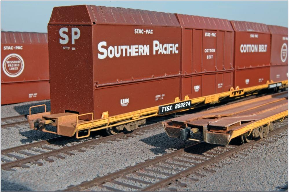
18. The coupler sat on the deck the PLH10 flat cars, which have 28-inch wheelsets. Risers were scratchbuilt on the ends of the low-riding flats so any cars or trucks could clear the topside coupler boxes.
