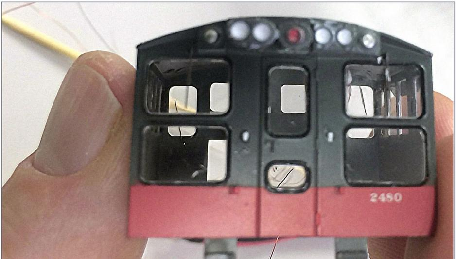
8. Lights with Micro Kristal Klear applied. Allow it to cure completely.
