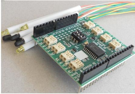
Many modelers use Arduino or compatible microcontrollers to create their own layout automation and animation effects. **Azatrax LLC**, a Colorado firm specializing in model railroad applications, has built four infrared (IR) proximity detectors into
