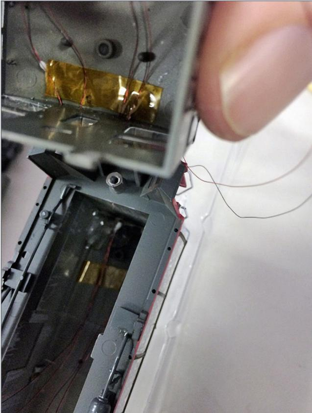
isolate the decoder from the frame and other metal parts, I made a simple styrene spacer which covers the motor and flywheels and keeps the board from shorting metal anywhere. I secured it in place with Kapton tape.
