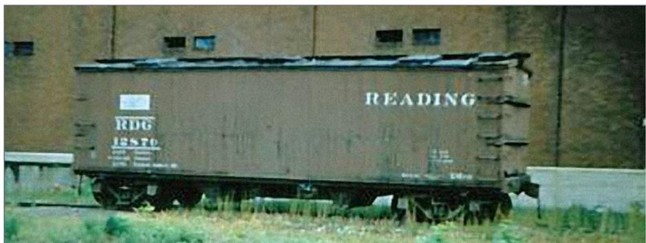
31. This poor photo shows one of the Reading's cars very late in life, having been rebuilt into a sand service covered hopper in the 1960s. This car is still on the revenue roster, since it had to be interchanged for loading. This photo was taken right after the formation of Conrail in 1976.
