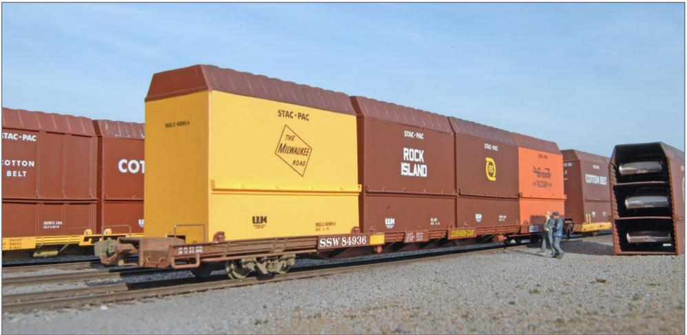
16. The containers were open on one end to accept three Cadillacs, Buicks or other full-size GM cars from 1971 to 1976 until smaller GM cars came out in 1977 and rendered the Stack Packs obsolete. The containers were loaded on the flats with their open ends to the center, with only 4" of clearance, making access by vandals almost impossible.
