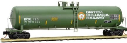
The prototype of this 56-foot general service tank car was built in 1983 to carry diesel fuel for BCR.
