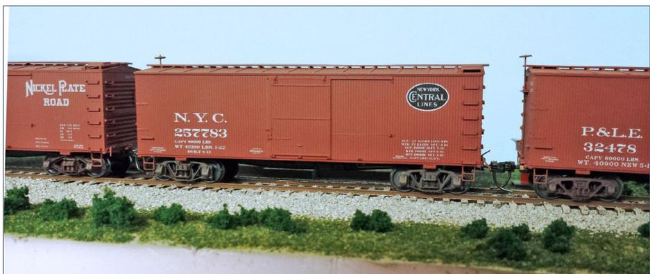
3. Small detail additions like cut levers and prototype-correct trucks have been added to all three of these new Accurail box cars to bring their “basic car” detailing more in line with higher-end kits.
