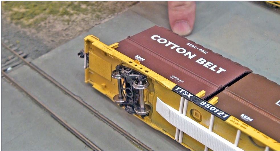
19. Mike used Shapeways printed parts on the sides of the cars to represent the inspection holes for the trucks.
