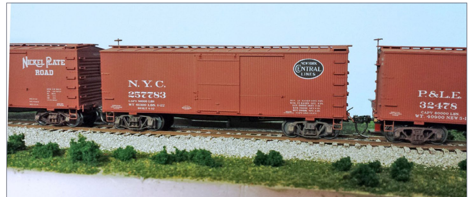
3. Small detail additions like cut levers and prototype-correct trucks have been added to all three of these new Accurail box cars to bring their "basic car" detailing more in line with higher-end kits.
