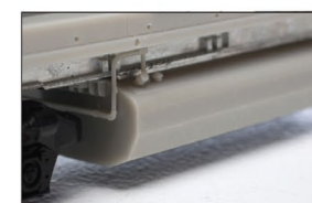
NS specific crash-worthy fuel tank per prototype
