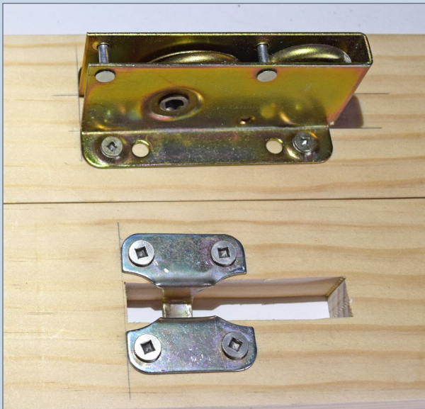
15. The Norse latch and receiver mounted in place.
