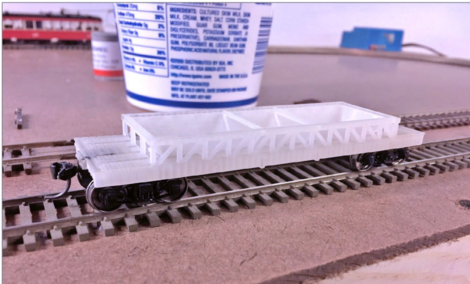
8. I built a module with 10"-radius track curves to test inter-urban equipment on this tight radius. The car performed just fine.
