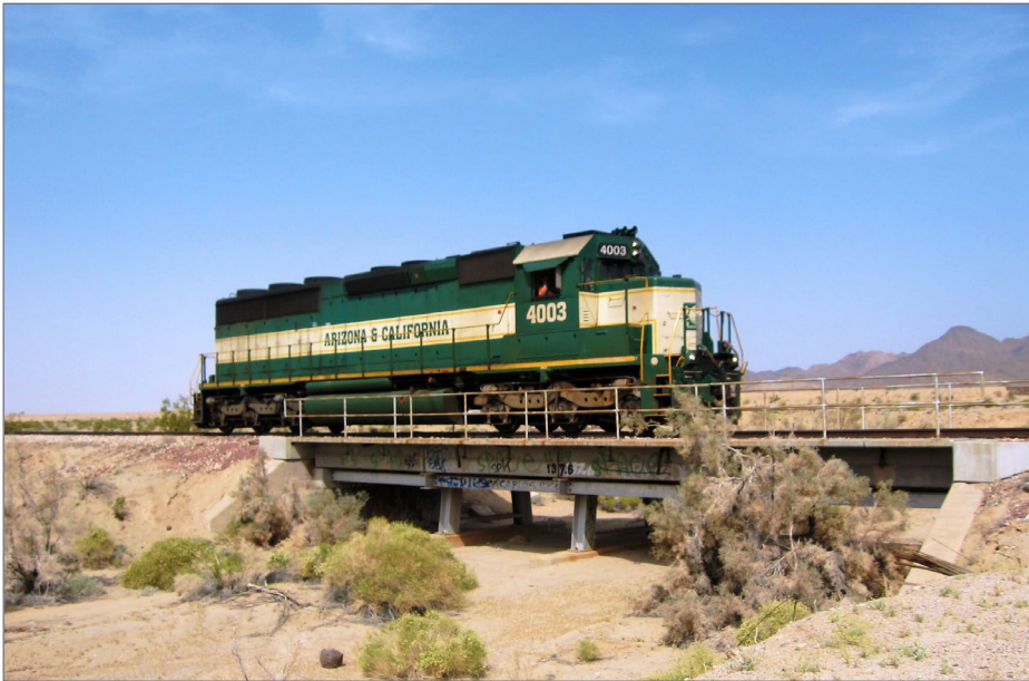
8. ARZC 4003, a rebuilt SCL SD45-2 rebuilt to an SD40M, crosses a dry wash at MP 137 near Rice. KL Smith
