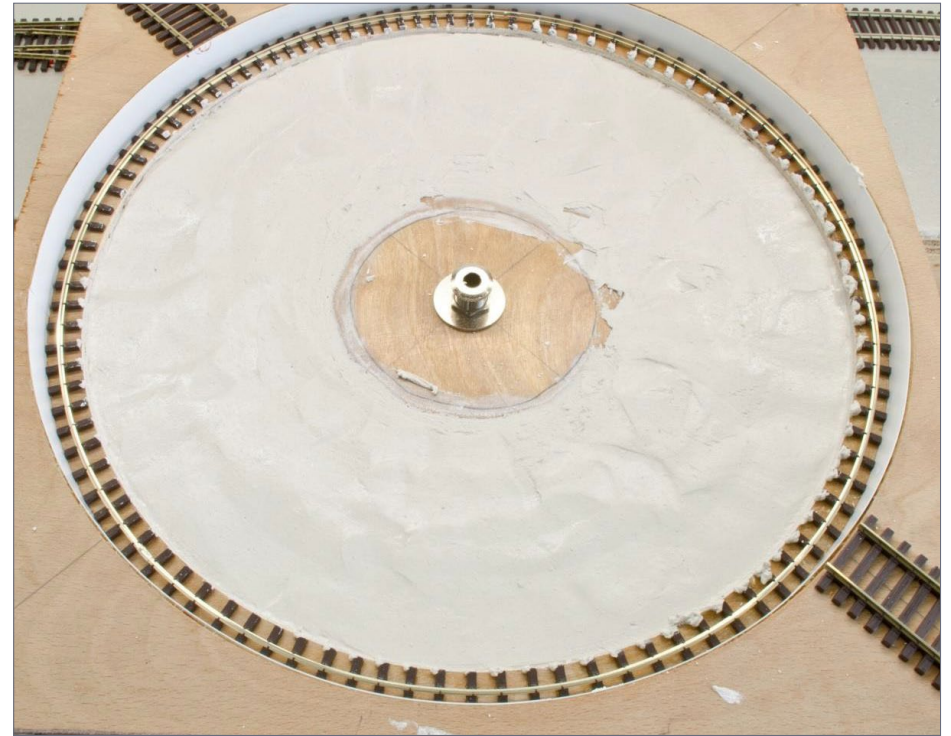
67. Finally, polish the surface with a wet spatula to get a smooth finish. You will need to take more time and care with this than I did if you want to represent finished concrete!
