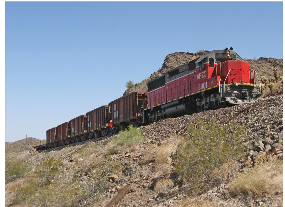
20. An ARZC ballast train moves through Harcuvar Hill. The five ballast hoppers in tow are rebuilt ATSF PS2 hoppers with open tops and ballast unloading doors. KL Smith
