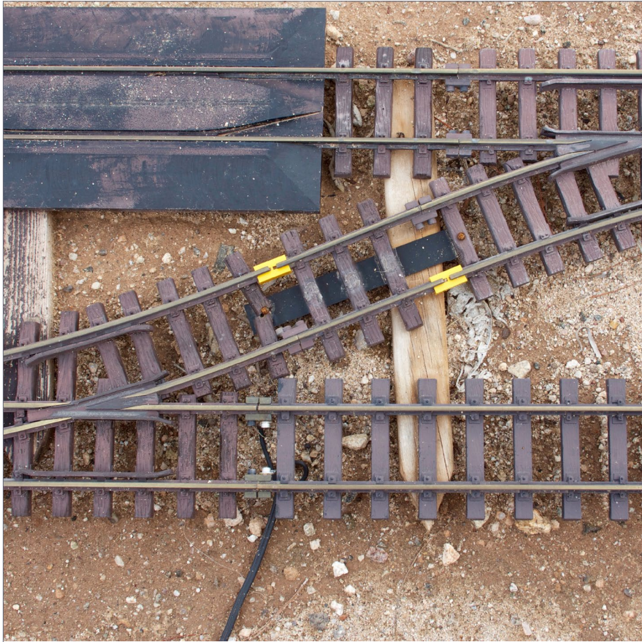
11. Insulating gaps (yellow) on both rails of my garden layout. Note the about four-inch stagger between the two rails.
