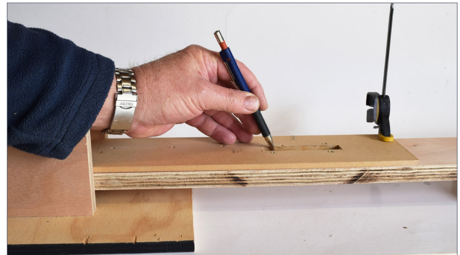
5. Mark the slot position and the drill holes through the story board.
