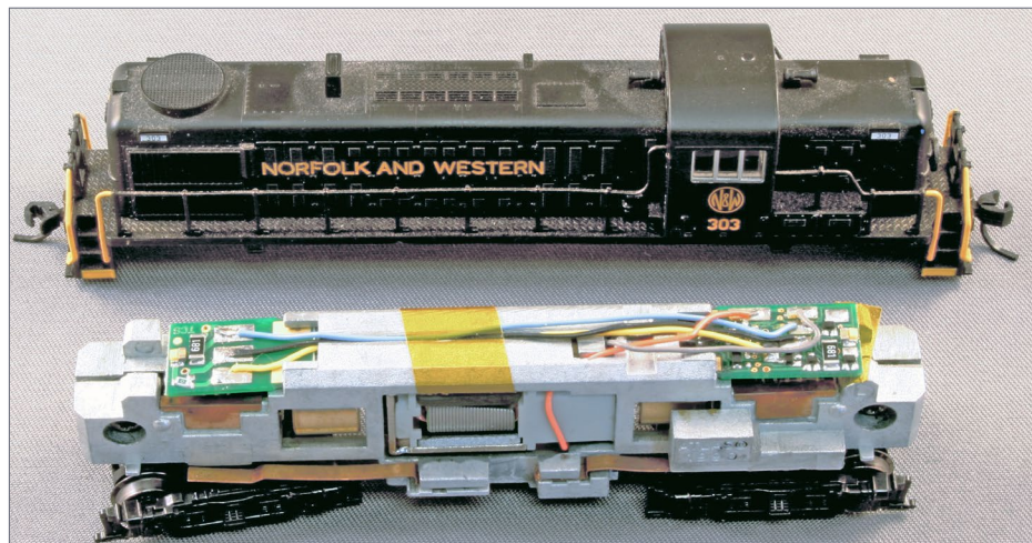
3. A TCS CN decoder in an Atlas RS3, circa 2008. Quite a change from [2] in just over five years.
