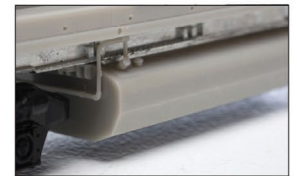
NS specific crash-worthy fuel tank per prototype
