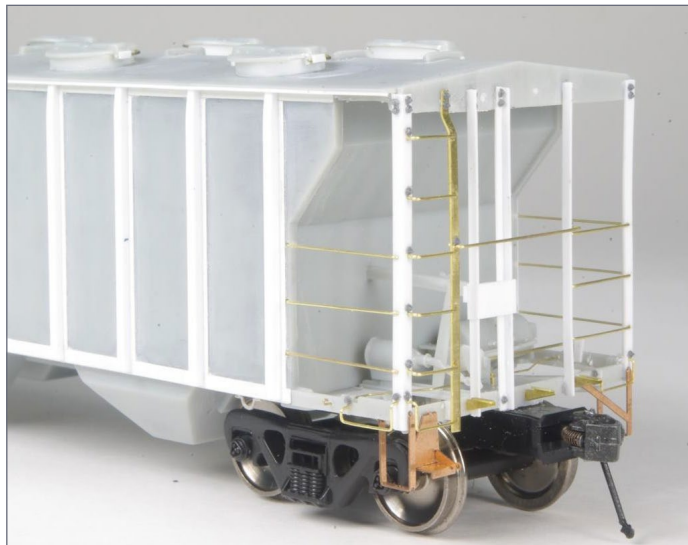
22. B end of car with grab irons, stirrups, and other details in place.
