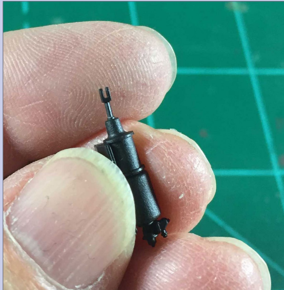
8. Closeup of the brake casting. Here's the K brake casting with the sprue nubs cleanly trimmed off.
