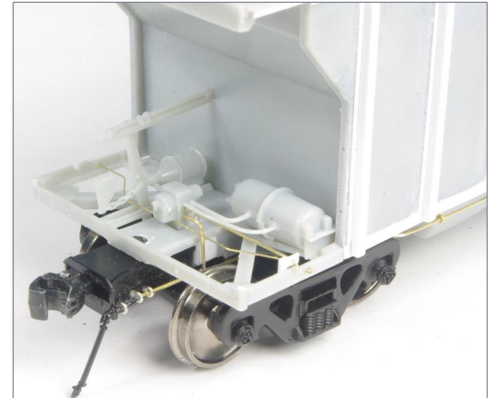
19. Completed brake system detail. Note the piping to the brake valve on the center sill, and the retainer rods out to the side.
