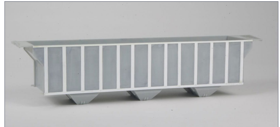
4. .005" styrene strips added to sides of car.
