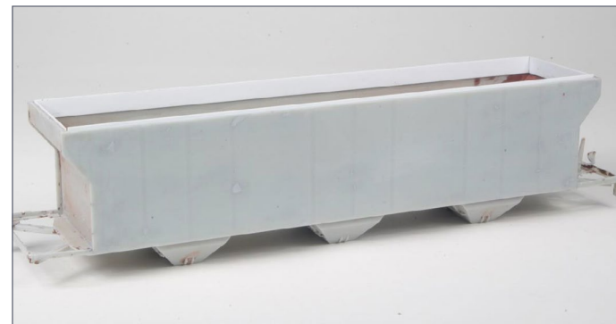
30. Thin styrene lip added to top of hopper body.
