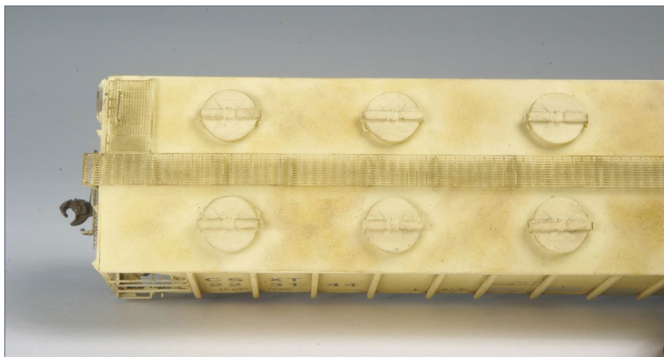
41. Roof weathering on CSXT 223144 with heavier weathering on roof panels, and less weathering around hatches.
