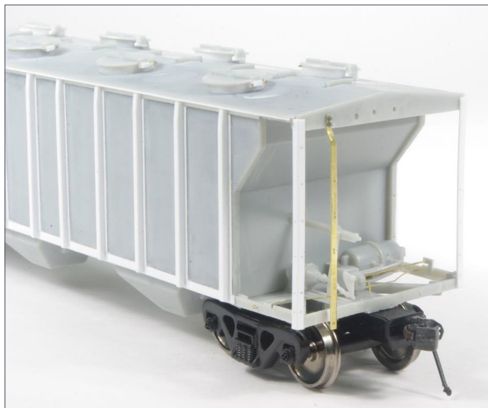
20. New corner posts and ladder post glued in place.
