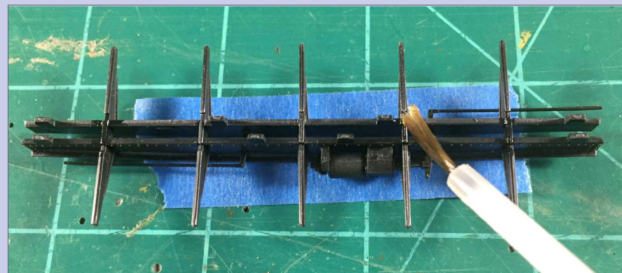
22. Install the remaining cross bearers. Let the cement dry for a moment. Then install the remaining cross bearers. Touch them with the cement to finish this part of the assembly.
