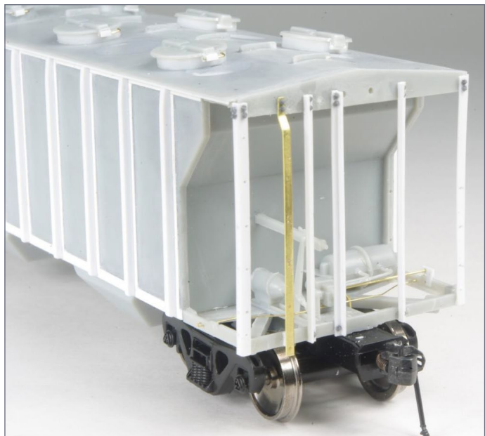
21. All vertical end posts glued in place on the B end, with gray nut-bolt-washer castings attached.
