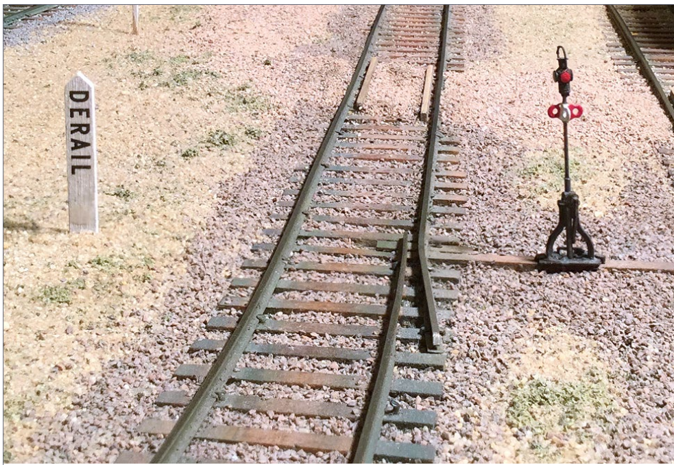
27. One of the two working derails with working switch stands protects the mainline from a runaway freight car.
