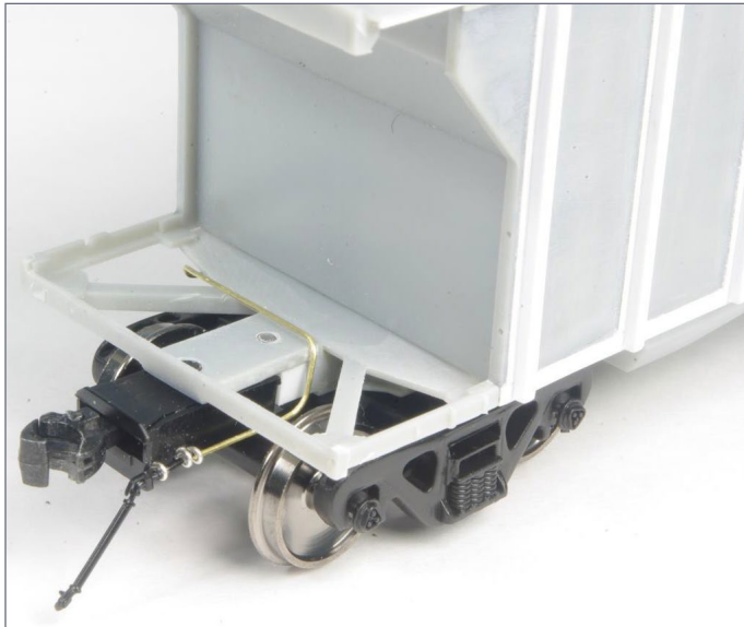
18. Train line on the A end of car.
