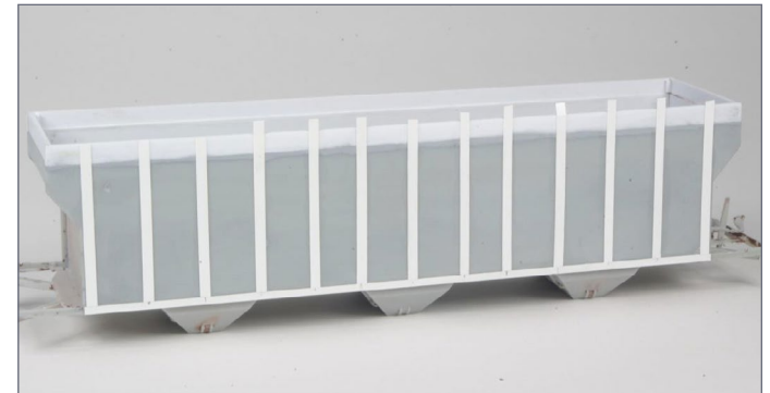
32. Strips of .005" styrene added to hopper sides.
