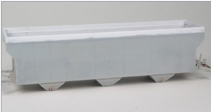
31. Extension added to hopper body.
