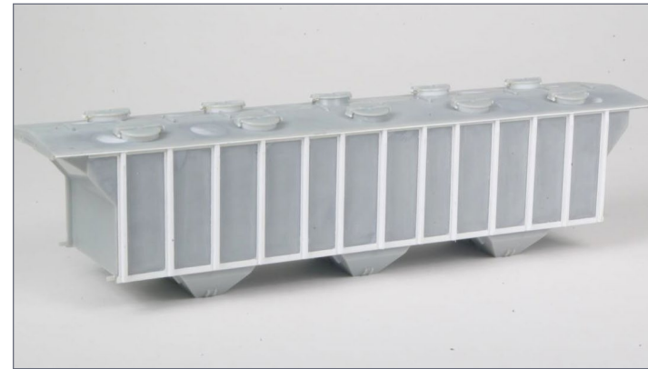
10. Roof glued to the hopper body with the hatches in the correct location.
