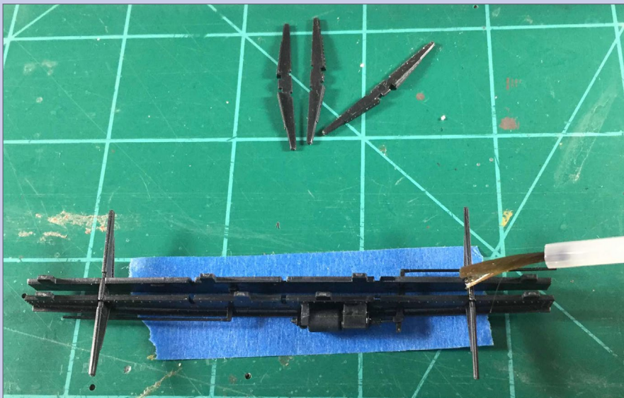
21. Cement two cross bearers in place. A touch of styrene cement fixes the two cross bearers in place.
