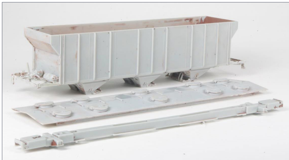
29. Athearn car disassembled and paint stripped using 99% isopropyl alcohol.
