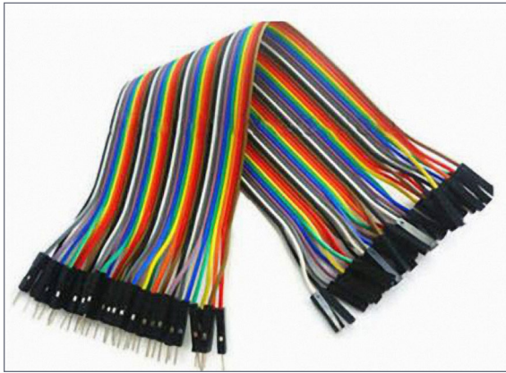
11. Jumper wires with pins on one end (left) and sockets on the other end (right).
