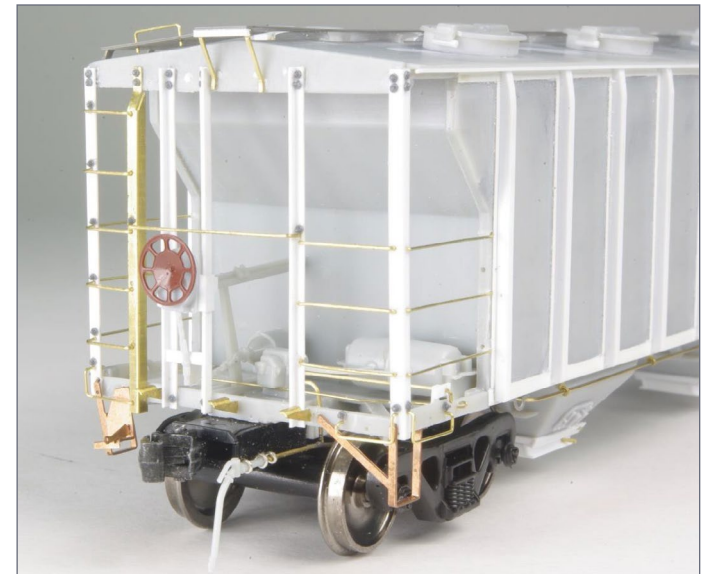
26. Completed end of car with roof walk supports and brake wheel.
