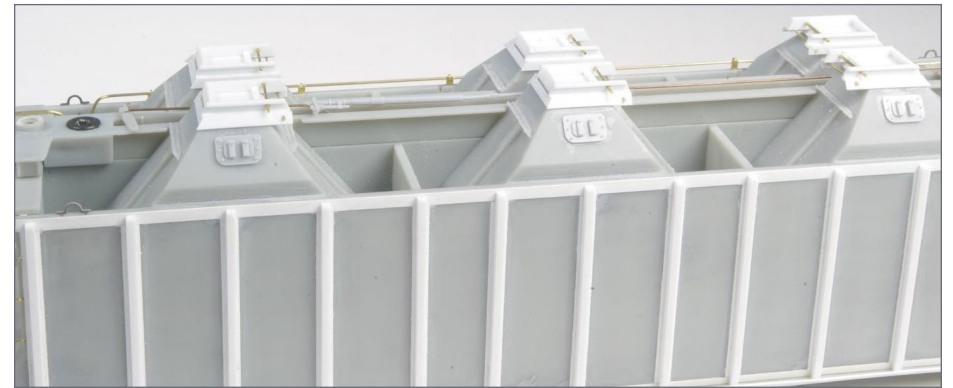
25. Completed hopper outlets and slack adjuster glued in place on center sill.
