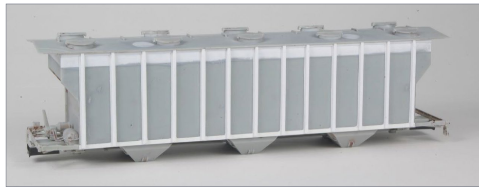
35. Roof glued in place with hatches relocated.
