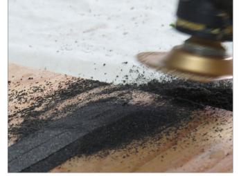
10. The grinding attachment is touted as being for tile grout removal, so you will get a lot of roadbed tapered before it wears out!
