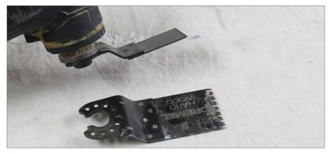
2. Both the wood blade on the tool and the wood & metal offset blade shown below the tool lets you cut flush to a surface.
