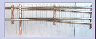
cedure, weighting the rail and checking gauge as I went, except when I reached the throwbar. The points must be able to move, so to accomplish this, I placed a PC board tie as a shim temporarily between the straight stock rail and the curved point rail. I soldered the point rail to the throwbar and then removed the temporary PC tie shim. This left a gap that allows the points to move. I then removed the completely soldered scale track from the template.
