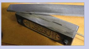
file the bottom of the rail to remove tarnish. Since this is not a switch, the rail will run the entire length of the scale track, and a point must be filed on each end. Like the curved stock rail, you will need to gently curve one point rail with your fingers to match the rail route on the printed plan.
