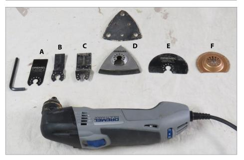
1. Here is the author's Dremel Multi-Max tool with attachments. From left to right: A) Flexible scraper; B) Wood & metal cutting blade; C) Wood cutting blade; D) Sanding attachment and sandpaper; E) Half-moon drywall and wood blade; F) Grinding attachment, purchased separately.
