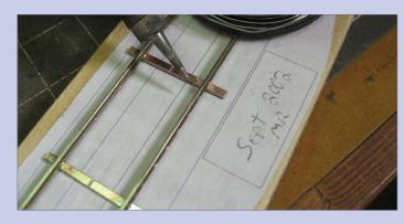
**9. Proper rail and tie prep:** A few light passes of the mill file on the tops of the ties and the bottoms of the rails will remove any tarnish. This way the solder joint will heat quickly and the solder will flow smoothly. Do this file prep now to make the soldering go easier later.
