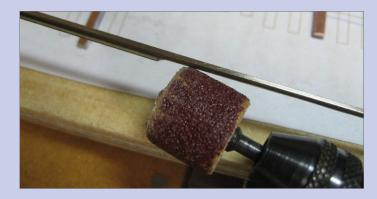
**8. Notch the stock rails:** The two outside rails are the stock rails and need notches filed in them to admit the point rails leading to the scale. Fast Tracks sells a tool called the Stock Aide for doing this (handlaidtrack.com/sa-m) but I did not have one, so I used a sanding drum in a Dremel rotary tool to notch my stock rails. To do this:
