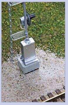
21. Plugging the finished signal mast into the DIP layout socket.
