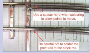
bar to allow the points to move. Be careful not to solder the point rail to the stock rail when soldering to the throwbar. If this happens (experience talking) you can generally loosen it later with your soldering iron and then file away any excess solder. I checked my work with my track gauge at each solder joint. The straight point rail should be in perfect gauge with the straight stock rail.
