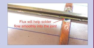
dering iron against the web of the rail. I placed the solder against the PC Board tie at the base of the rail, and kept the hot iron on the joint until the solder flowed. The solder should flow *under* the rail making a solid joint. Excess solder outside the joint is not necessary. The Fast Tracks site has some excellent videos on proper soldering techniques: [handlaidtrack.com/FTV-Turnouts-5].
