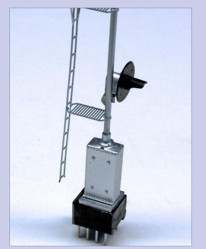
**18. Finished DIP plug base on the signal, snapped together and ready for final testing.**
