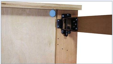
16. (Left bottom) This photograph from Kam Konnect shows how a dropdown module is built with 18mm Baltic Birch (13 plies thick, total 3/4") plywood sides and ends. The base is 1/4" hardboard with 1/2" foam board for scenery. I will add 12mm (1/2") cabinet-grade plywood for the track roadbed.
