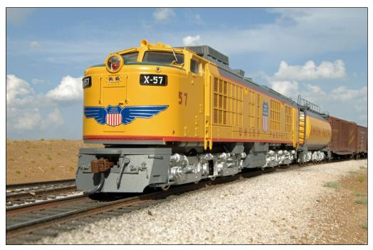
with Farr grilles on the sides of the locomotive – these are etched metal on the model. The screens were used to reduce the dust and dirt pulled into the unit's jet turbine and were removed by 1955.
