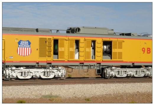
21. The side doors on the turbine unit slide open to expose the inner workings of the modeled turbine engine. Scaletrains.com also offers two types of fuel tenders, a C23 riveted shorter tender and a C24 smooth-side larger insulated fuel tender. UP operated both types and mixed them among units as time went on.
