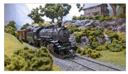
1. Chet Zaiko installed the headlight in this locomotive about 20 years ago. LEDs weren't common then. An MV lens that fit the headlight opening was drilled from the back to make it appear that there is a bulb in the light. An LED could also be used. Holes were drilled through the back of the headlight housing and the smoke box to feed the bulb leads through. *Chet Zaiko photo*
