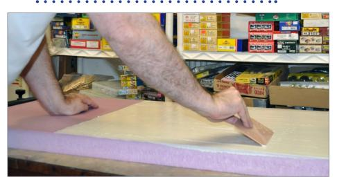
10. I applied Liquid Nails adhesive evenly to one piece of foam in preparation for laminating it to another piece of foam.
