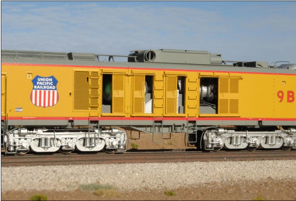
21. The side doors on the turbine unit slide open to expose the inner workings of the modeled turbine engine. Scaletrains.com also offers two types of fuel tenders, a C23 riveted shorter tender and a C24 smooth-side larger insulated fuel tender. UP operated both types and mixed them among units as time went on.
