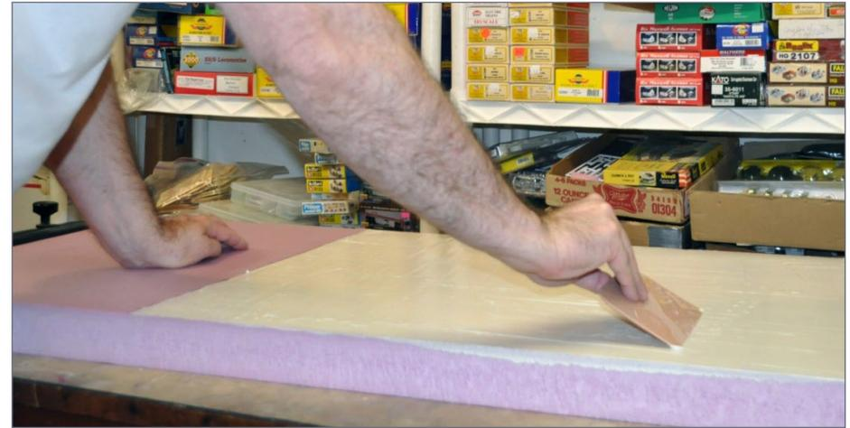
10. I applied Liquid Nails adhesive evenly to one piece of foam in preparation for laminating it to another piece of foam.
