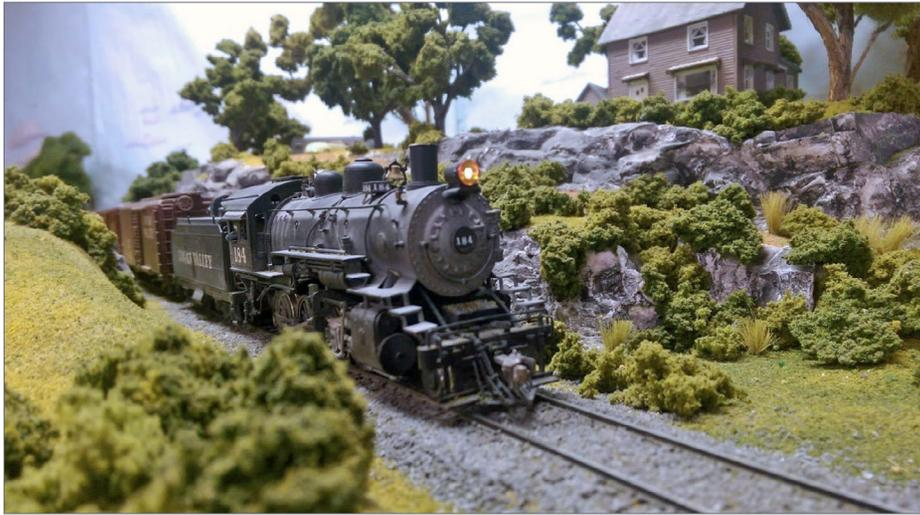
1. Chet Zaiko installed the headlight in this locomotive about 20 years ago. LEDs weren't common then. An MV lens that fit the headlight opening was drilled from the back to make it appear that there is a bulb in the light. An LED could also be used. Holes were drilled through the back of the headlight housing and the smoke box to feed the bulb leads through. *Chet Zaiko photo*
