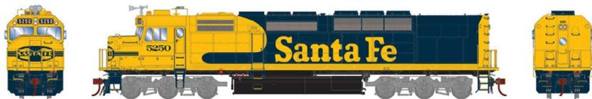
A Genesis EMD SDP40F decorated in Santa Fe's blue and yellow freight scheme is scheduled for release in October 2018. Notable details include a Leslie S3L horn, illuminated Strato-light, two Sinclair antennas, and blank plates at rear where the steam generators were removed.
