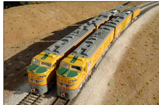
17. The veranda turbines were retired by 1964 and traded in to GE, which used the turbines' trucks when building the U50 series locomotives (above) with two diesel prime movers aboard (below).
