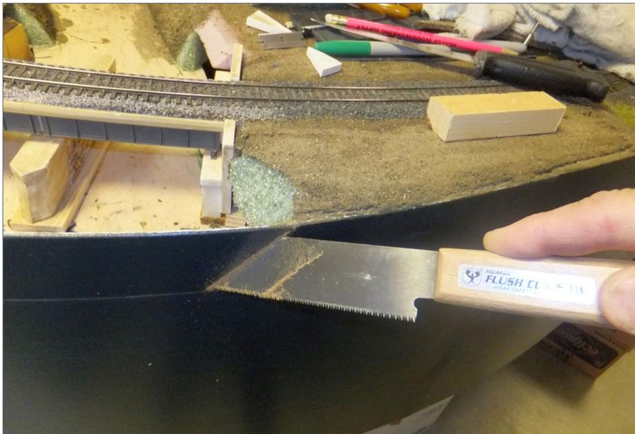
48. Side angle cuts were done by hand with a flush-cut saw.
