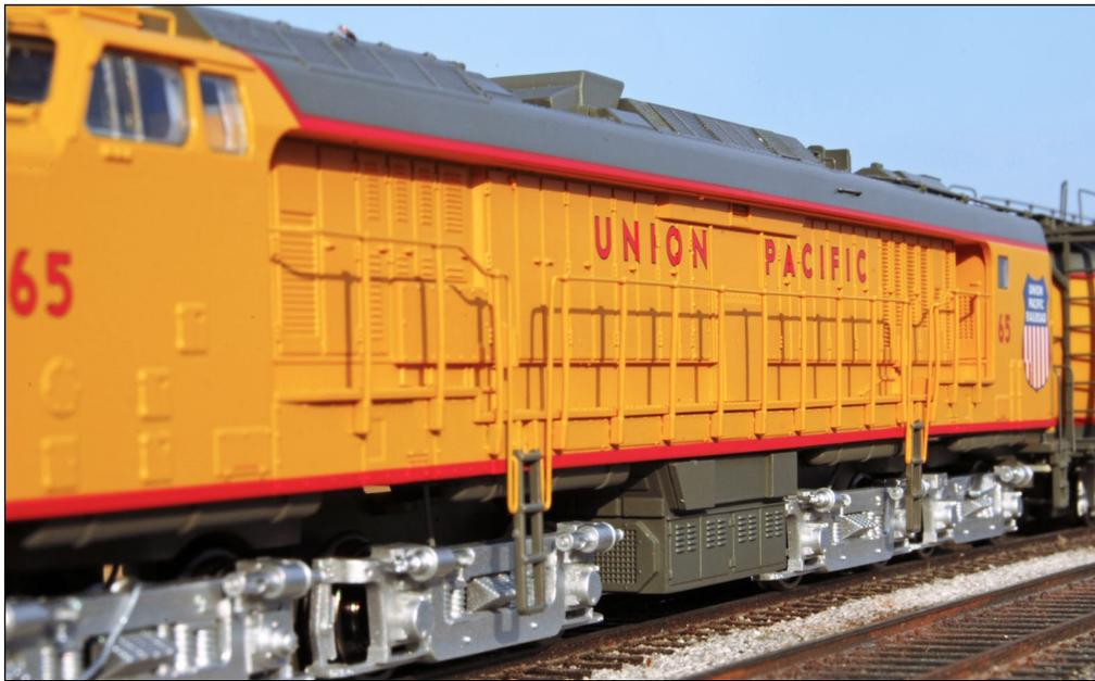
16. The verandas had walkways built along the sides, with doors on the long hood for easier access to the inner workings of the locomotive. Rated at 4500 horsepower, UP had 15 of these units, numbered 61-75. These units also received fuel tenders around 1955, again to increase the range of the units.
