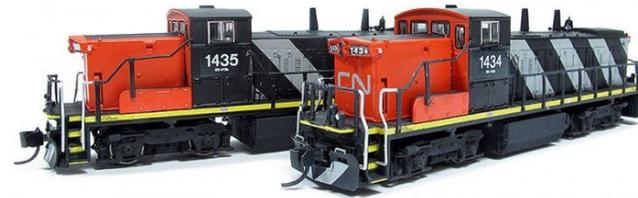
Rapido's 1400 series GMD-1s represent units rebuilt in 1988 with new prime movers and a new paint scheme. They were rebuilt again in the late 1990s with four-wheel trucks replacing the original six-wheel units.
