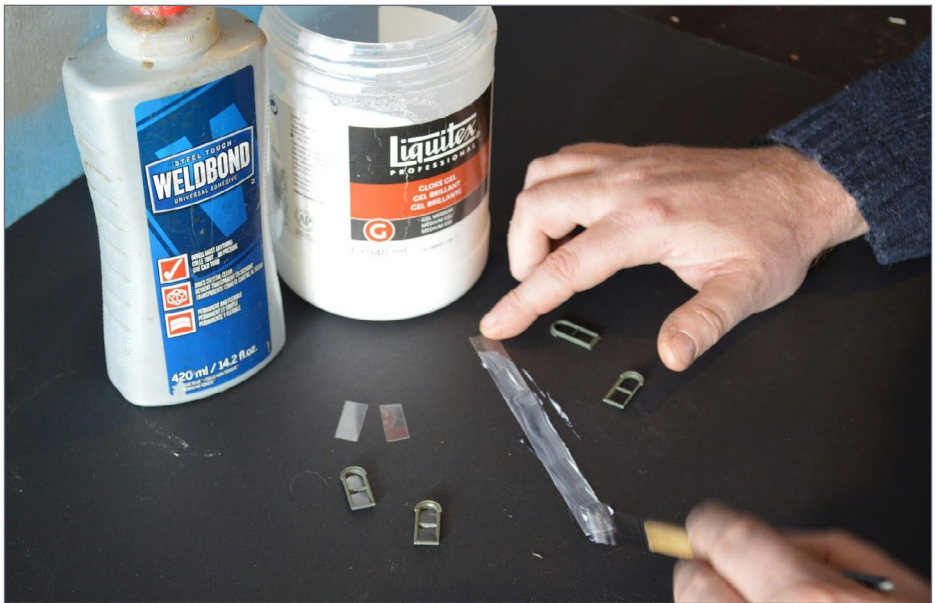
14. Paint a strip of acetate with a layer of gloss medium. Make the coating thin. It will not be enough, but don't fret.
