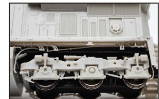
Separately-applied plumbing and traction motor cables.
