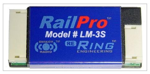
3. Each loco will need a module to control the motor and lights. If the module has a "S" suffix, it also includes sound. Here is the LM-3S sound loco module. *Ring Engineering photo*
