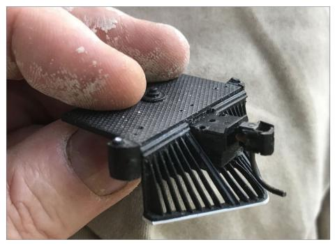
2. Neil Erickson addressed his working-coupler problem: "The pilot comes off the loco easily enough and I could open up the coupler pocket enough to insert a Kadee box but it looked a little strange. Maybe some diamond plate over the top would be OK, or I may cut off the trip pin and push it back as far as possible." *Neil Erickson photo*
