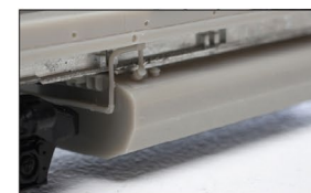
NS specific crash-worthy fuel tank per prototype
