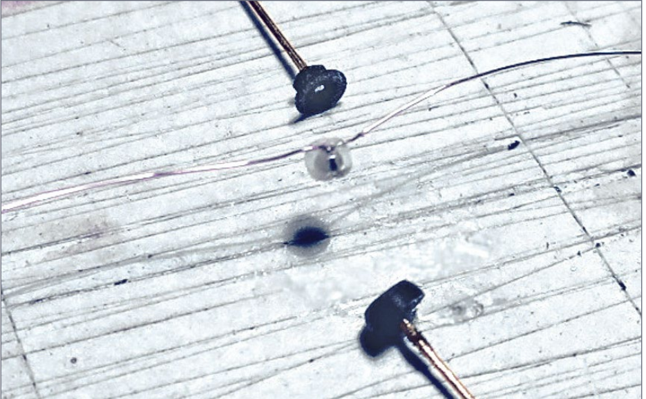
29. Assembling is very difficult if the LED was inserted into the bead previously.
