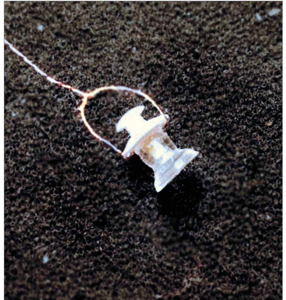
18. The wires are twisted together into a handle.
