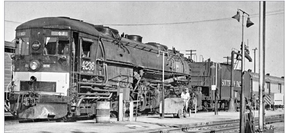
12. The wheeled work cart near the center of this view has a gable top, though flat tops are far more common in SP photographs. The striped barrel is also noteworthy. The scene is at Tucson, AZ where power was changed on many trains, and minor repairs often made. Al Phelps photo, August 1952, Signature Press collection
