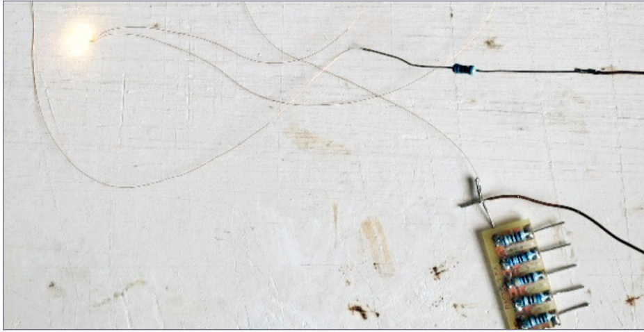
14. Check that the LED lights up.
