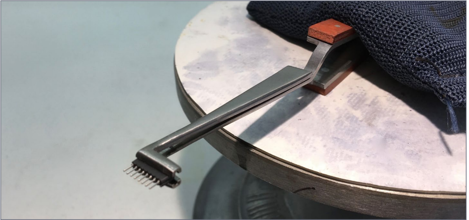
11. Clamping tweezers holding a multi-pin header. The tweezers are positioned on the decorating wheel by a shot bag. Bruce Petrarca photo
