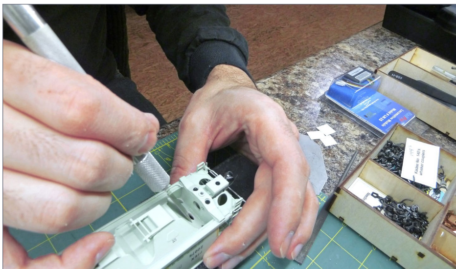
14. Cleaning up the openings with a chisel blade.
