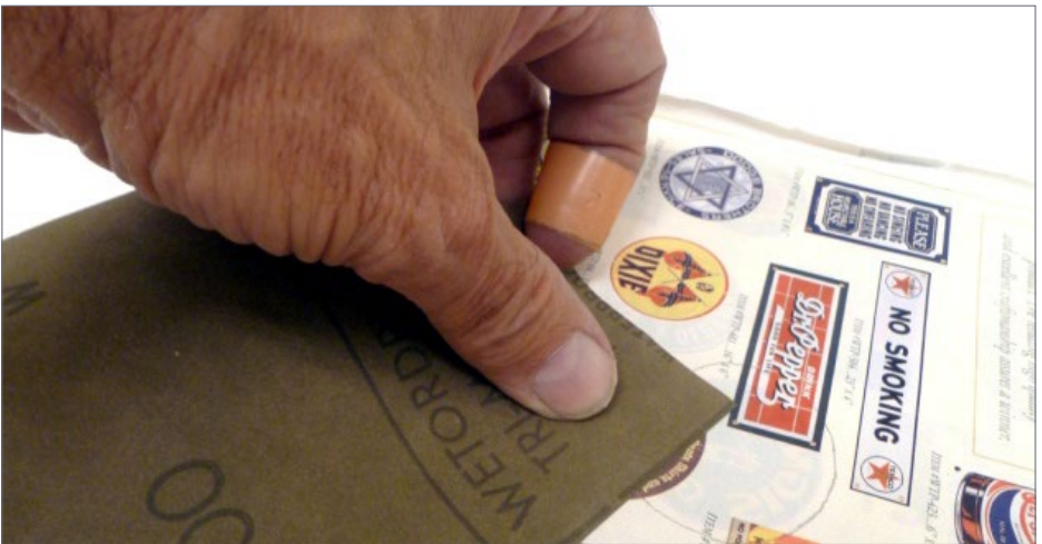
14. Thin the sign by carefully sanding the back. (Make sure to use the sandpaper on the back of the sign, not the front.)
