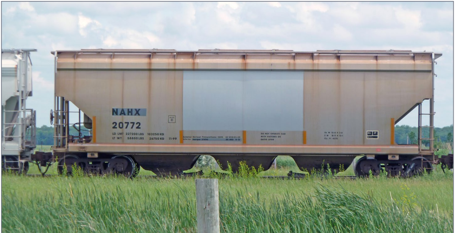
1-2. Typical example of the NSC three-bay potash hopper, in NAHX and Agrium paint, seen in Emerson, Manitoba.
