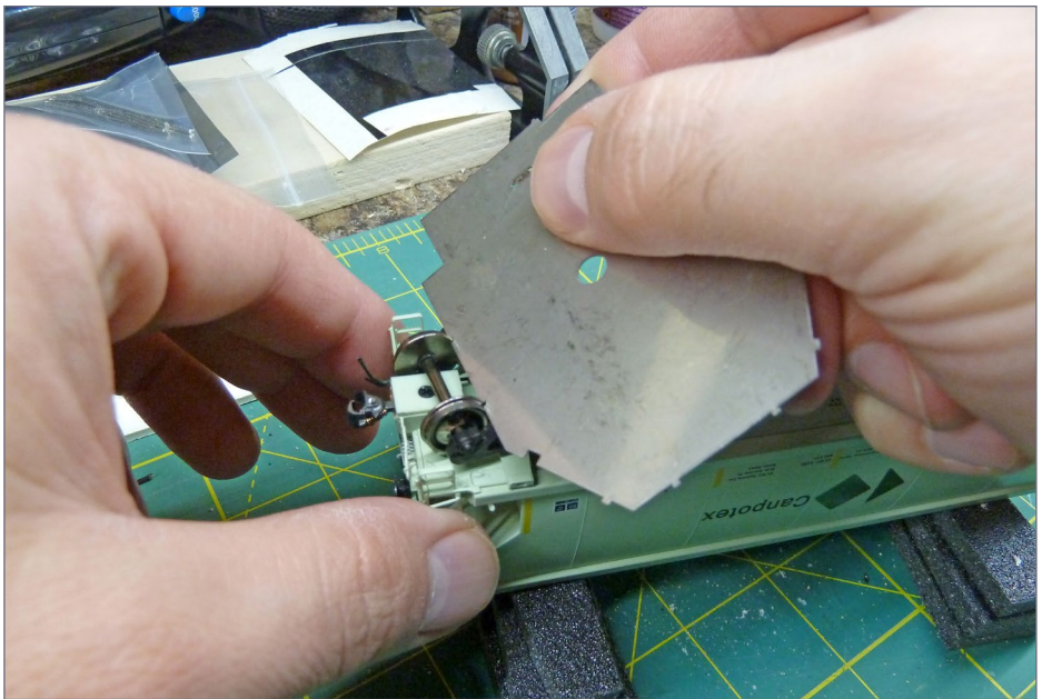
7-8. Checking the wheel gauge.
