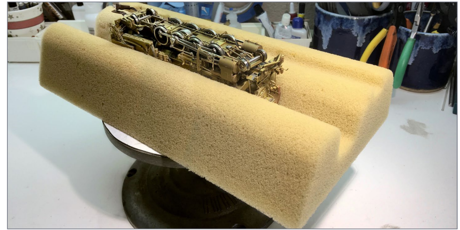
9. Decorating wheel holding up a foam cradle and a loco. Bruce Petrarca photo
