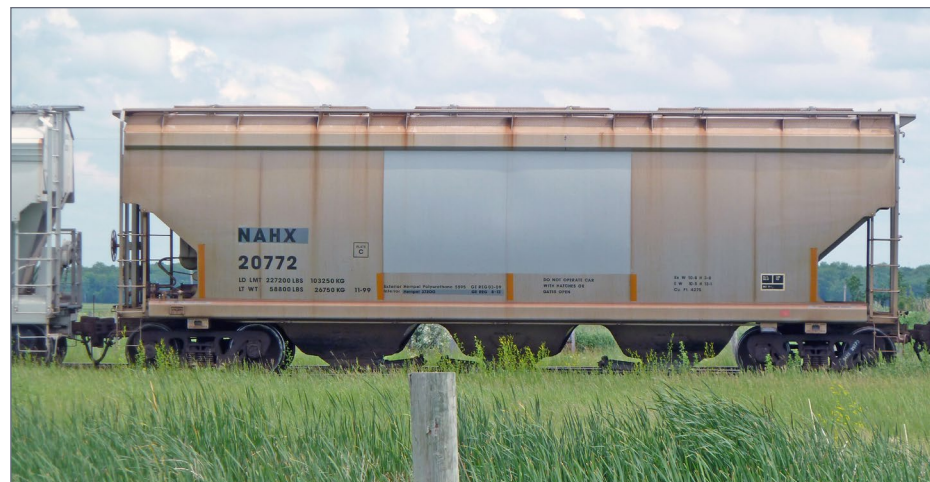
1-2. Typical example of the NSC three-bay potash hopper, in NAHX and Agrium paint, seen in Emerson, Manitoba.
