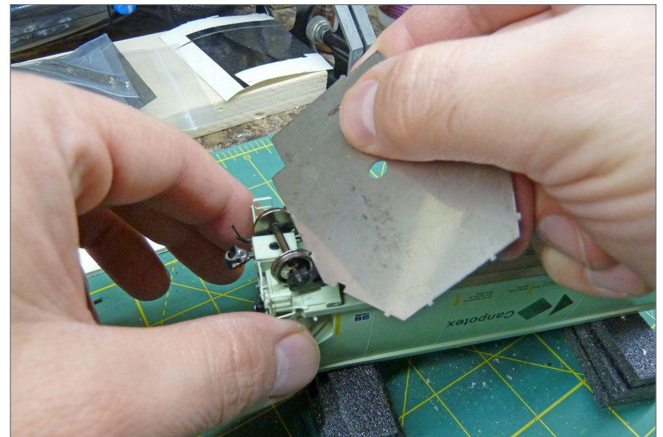
7-8. Checking the wheel gauge.
