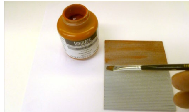
40. Brush the siding with dilute red acrylic paint along the grain of the boards.
