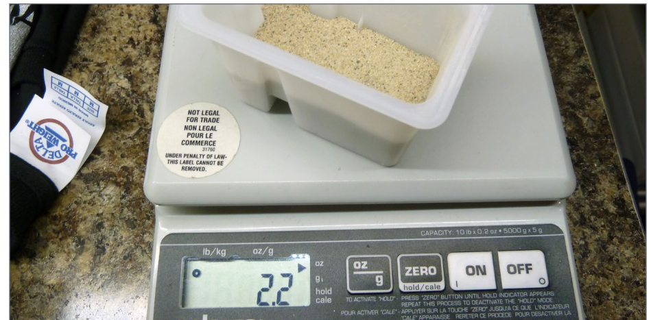
16. Tip: Zero the scale with the container on it and then add the sand to be weighed.
