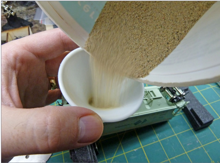
17. Pouring the sand slowly on the slope of the funnel prevents the funnel from clogging.
