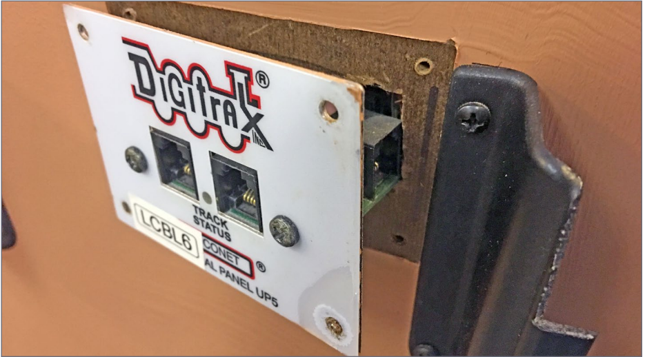
5. Mounting screws have been removed allowing the UP5 panel to slide out of the PCMRC layout. Bruce Petrarca photo
