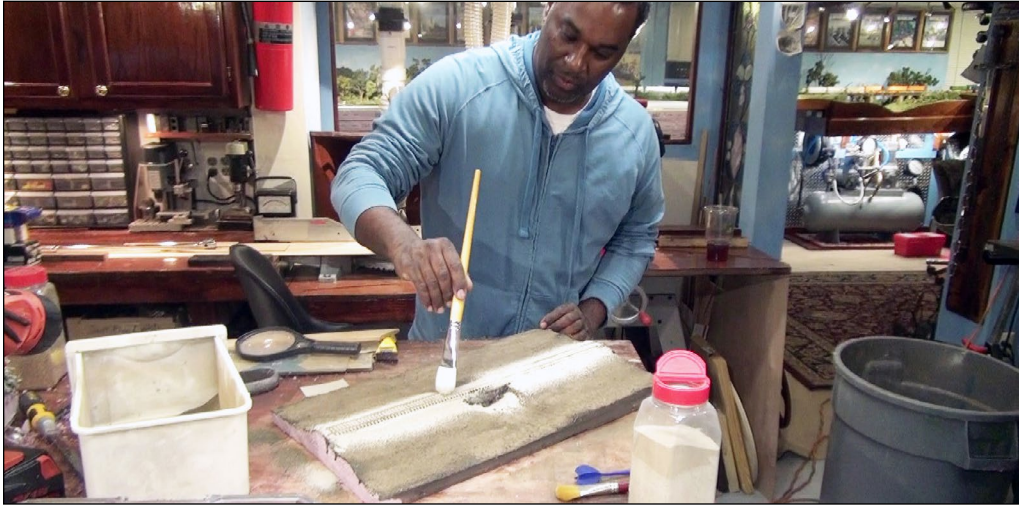
30. We apply ballast to the scene and spread it with a curved artist brush. The curve in this brush allows only the tip to come in contact with the scene, making it very easy to spread the ballast smoothly between the ties. A brush like this retails for $28 but is well worth the price for perfect smooth ballast and time saved.
