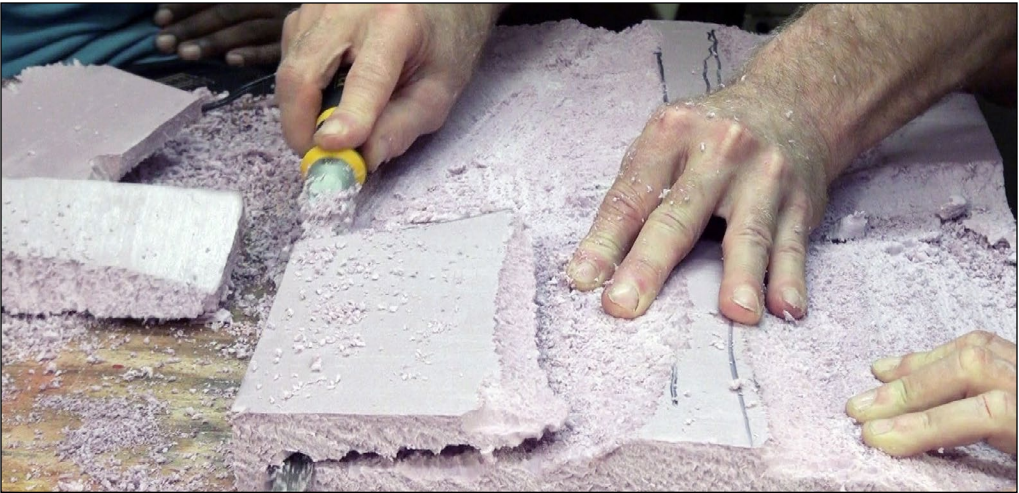
26. To carve surrounding scenery for the creek and tracks we use a pruning saw blade attached to a strong handle. This allows for fast rough cutting of foam, to tear through the topography quickly.
