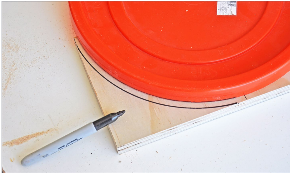
6. I used the lid from a 5-gallon plastic bucket to mark the radius for the cove supports.
