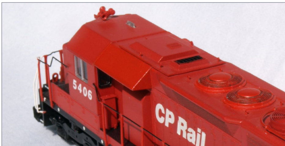
17. The completed awnings over the air intakes.
