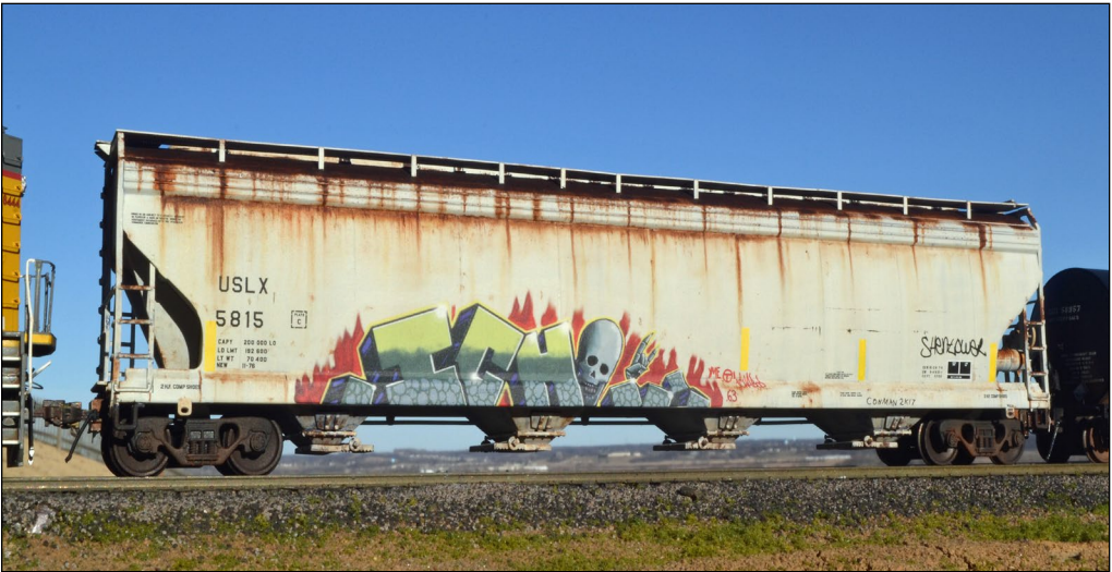
19. The covered hopper is weathered with oil paints. The burnt umber rust streaks were applied with a fine artist's brush. He then applied colorful graffiti decals to make the car stand out.
