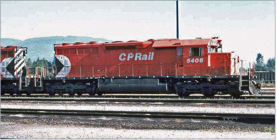
14. CP 5406 in Port Coquitlam, BC on October 11, 1986. Note the rounded dynamic brake fans. Claude Prutton mountainrailway.com
