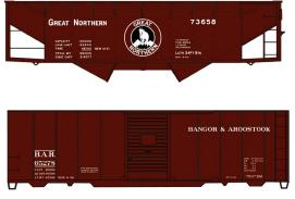
The kit for this 50-ton twin-bay hopper car with offset sides is based on a Great Northern car built in 1934.
