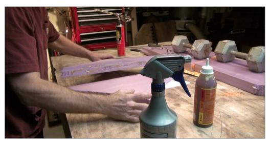
4. I also glued two sections of foam together with Gorilla Glue and water, setting this aside under weights to cure and expand to fill imperfections in the foam to create a tight joint.
