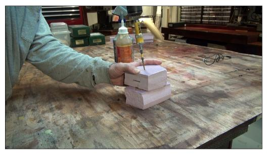
10. I tested a section using one 2.5-inch-long wood screw to hold the Gorilla Glue joint together.
