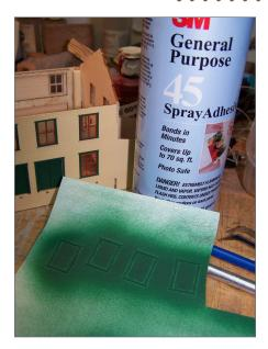
5-6. (Left and below) After applying spray adhesive to the paper, the window frames and the trim parts with their self-stick backing are affixed to the paper and sprayed with paint.
