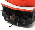
Amtrak style pilot, with steam line access door snow plow.
