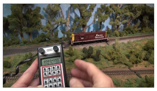
36. First, we set CV 2.503 while the model is running on the layout in speed step 1 on the DCC throttle. While the model is moving, program the CV to around 255.
