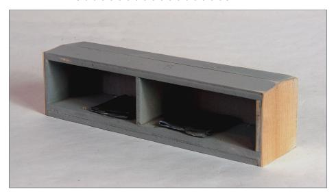
8. Wood car models are very light so they will never track well unless weight is added. Interpolating the NMRA standards between HO & O scales, I arrived at a weight of 5.3 ounces. The car and all of its hardware was placed on an old balance scale from a science kit. Lead chimney flashing (available at lumber yards) was added until the correct weight was reached. Fastening with five-minute epoxy makes sure the weights will never shift.
