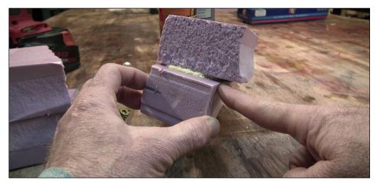
11. After 15 minutes, this joint shows signs of failure as the glue pushes the two foam sections apart.
