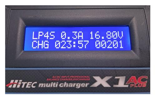
6. HiTEC multi charger X1AC+ topping off the charge in a pack. This display shows: Lithium ion 4 cells (LP4S); charging at 0.3 A; with a battery voltage of 16.80 V; it has been charging (CHG) for 23 minutes and 57 seconds; 201 mAh have been added to the battery. *Bruce Petrarca photo*
