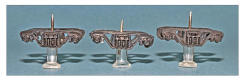
4. Prep plastic trucks for paint and weathering by scrubbing them with a paste of water and cleanser. Left, an untreated truck; center, an alcohol-washed truck; and right, a Bon Ami-prepped truck. *Josef Brugger photo*
