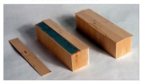
9. Now that the true thickness of the walls is established, the outer, overhanging roof is attached. Allow about 1/16" overhang since half of that will be taken up by the fascia boards. Careful observers will notice that a 1/16" x 1/32" strip has been attached to the sides to accommodate the freight door tracks.
