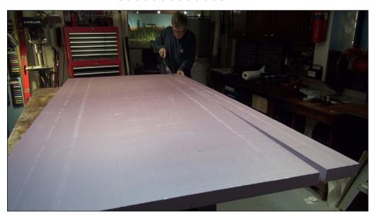
13. Measuring 6 inches wide, I cut a few sections of foam. These will create a 10-foot-long by 4-inch addition for the layout. I cut this with a thin Chinese style pull saw for a clean cut.
