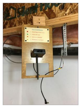
4. Here is the RB02 radio receiver in the spot previously occupied by the UR-92. I read that the best place to put the RB02 is in the center of the room, on the ceiling, and turn it upside down so the radio waves spread out like a mushroom and reach all operators. This placement passed the test of the first op session. The opening at the bottom of the panel housed a fast clock display that was relocated.
