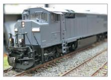
The HO scale model is Rapido's first release in its budget-priced Prime Movers series. Features will include working ditch lights, metal grab irons, and a decoder (decoder plug on DC models) easily accessible in the fuel tank.
