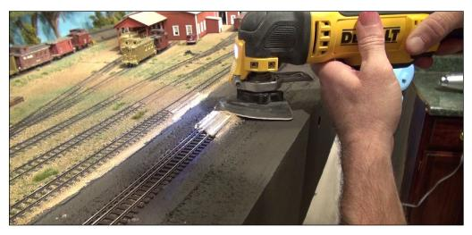
27. I used my oscillating sander to sand flat the tops of the railroad ties that form our crossing, stoppin when I reached the top of the rails. I used to do this by hand with a wood block and sandpaper but the oscillating sander speeds up this process.
