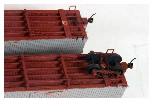
25. The underframe with a second coat of paint and the Bachmann arch bar trucks installed. Painting the wheels and trucks contributes greatly to the appearance. I painted the trucks with Burnt Sienna and the wheels with Delta Ceramcoat Charcoal.
