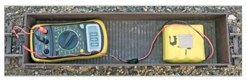
3. Battery pack and multimeter set for 10 amps running in trailing gondola to verify locomotive current draw. *Bruce Petrarca photo*
