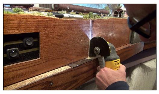
14. I attached a saw blade to my oscillating sander to cut the plywood fascia. The new foam will intersect the plywood at an angle. No other type of saw on the planet, that I am aware of, could make this cut without removing the module or cutting into the table-top benchwork. I am always finding new uses for this oscillating tool. It worked well and I did not have to remove the module. Note, I am using a steel ruler to protect the table's top from the saw blade.
