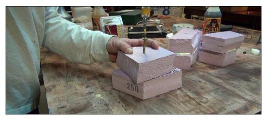
12. After thinking about it overnight, I picked up some 4-inch wood screws with large half-inch round pan heads. Using these larger screws, I repeated the experiment of gluing two sections of foam together using Gorilla Glue. After 30 minutes, the glue was hard with no visible expansion between the foam sections. I now had a good way to clamp/screw the foam in place while the glue cures and expands.
