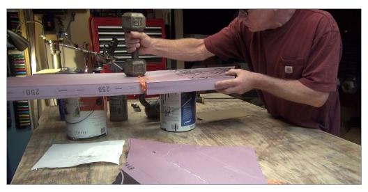
5. Six hours later I came back to test the glued sections of foam. I set up the glued panels between two paint cans and tested each glue joint by dropping a 15-pound dumbbell weight on the foam from a height of about two inches. Both glues held up to this abuse.
