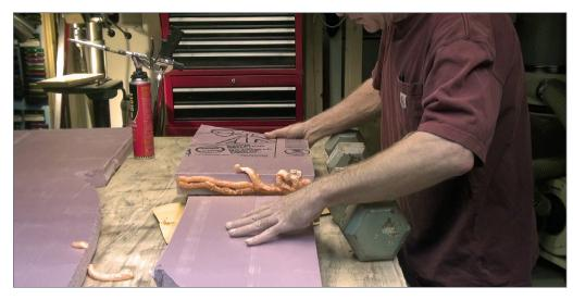
3. To test the idea, I glued two sections of 2-inch pink foam together with the Great Stuff Foam Pro we always use on the show, and weighted the assembly down to cure.
