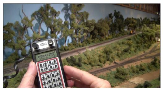
37. The next step is to set CV 2.504 while the model is moving in speed step 30. This process lets the decoder draw a graph in its internal memory, understanding the gear drag and pull weight of the locomotive when running light. This will allow the decoder to differentiate and understand when it is running light or heavily loaded, changing the tone and performance of the sound effects to match what the locomotive is doing.
