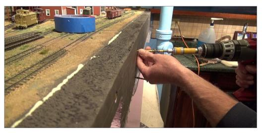
18. You can see how the glue squeezed up through the foam joint. This expansion fills any gaps between the foam panels, ensuring a solid, hard, strong bond. It is simply amazing glue. With the glue set, I removed the screws to use them on the next section.
