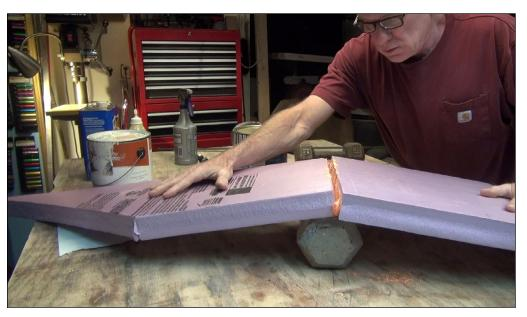
7. I wanted to break the glue joints to understand the strength and pressure required. so I placed the Foam Pro section on top of a dumbbell and pushed the sides down, breaking the glued joint fairly easily.
