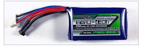
2. RC style battery pack. This is a 3S 350 mAh pack designed to be discharged as quickly as 130C. Note the two connectors, one for the model and one for the balancing charger. The (two-wire) model wires are very large gauge. The (four-wire) balancing charger wires are a bit smaller. Since this pack is rated at 130C discharge, it will supply over 40 amps for about 2 minutes. Not recommended for model railroading. *Pete Steinmetz photo*
