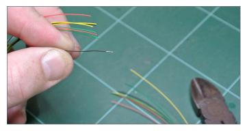
13. Wire with sheath removed and tinned.
