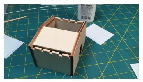
13. My third model of the oil house under construction. The basic "box" is 1/8" birch plywood. The laser-cut sides produced by Monster Modelworks include cut-outs for the I-beam roof supports.
