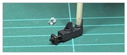
19. Light pipe being pushed into the housing opening.
