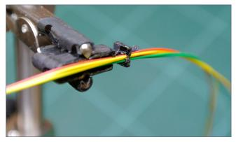
8. Test fitting all eight wires through the housing base hole.
