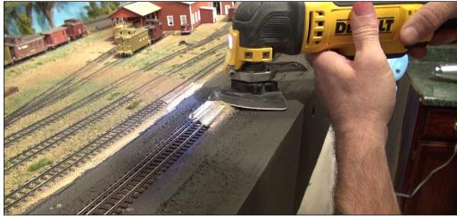
27. I used my oscillating sander to sand flat the tops of the railroad ties that form our crossing, stoppin when I reached the top of the rails. I used to do this by hand with a wood block and sandpaper but the oscillating sander speeds up this process.
