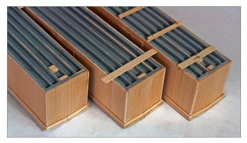
16. The prototype photos provide no information on the underside, so my plans are based on the details of a Bachmann gondola car. This is probably typical of wood car construction. A wood block was placed under the coupler pockets and the truck centers to provide material to hold the screws. A 1/32"x 1/4" bolster came next. The queen post beams are 3/32" x 1/8". It is much easier to drill locating holes before detail is added to the sides.
