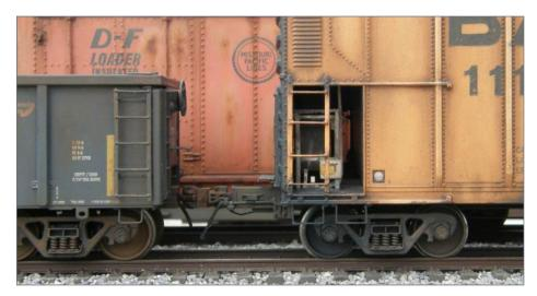
2. An alcohol wash cleans grease and other residues from slippery engineering plastics, leaving a clean surface for painting and weathering. On the left is an Atlas Master Thrall 2743 gondola with ExactRail trucks and ExactRail 33" .088 wheels. On the right is a superdetailed Athearn blue box 57-foot reefer with the same type of trucks and wheels. *Terence Boardman models and photo*
