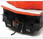
Amtrak style pilot, with steam line access door snow plow
