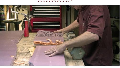
3. To test the idea, I glued two sections of 2-inch pink foam together with the Great Stuff Foam Pro we always use on the show, and weighted the assembly down to cure.
