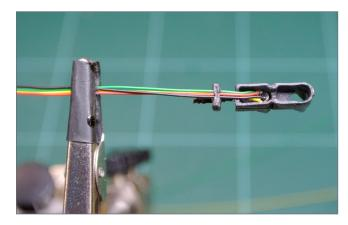
23. Wires threaded through the base hole.
