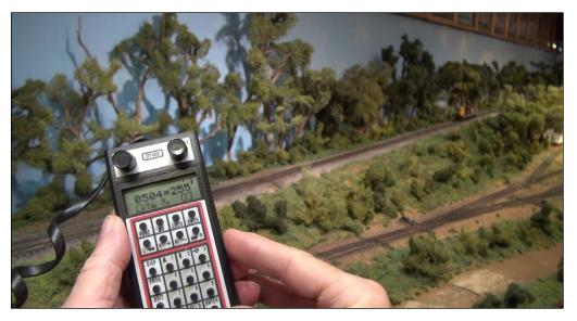
37. The next step is to set CV 2.504 while the model is moving in speed step 30. This process lets the decoder draw a graph in its internal memory, understanding the gear drag and pull weight of the locomotive when running light. This will allow the decoder to differentiate and understand when it is running light or heavily loaded, changing the tone and performance of the sound effects to match what the locomotive is doing.
