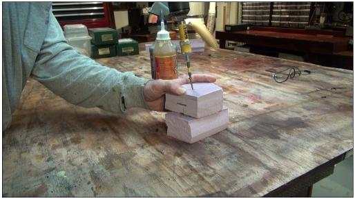
10. I tested a section using one 2.5-inch-long wood screw to hold the Gorilla Glue joint together.
