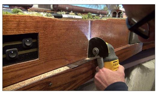
14. I attached a saw blade to my oscillating sander to cut the plywood fascia. The new foam will intersect the plywood at an angle. No other type of saw on the planet, that I am aware of, could make this cut without removing the module or cutting into the table-top benchwork. I am always finding new uses for this oscillating tool. It worked well and I did not have to remove the module. Note, I am using a steel ruler to protect the table's top from the saw blade.
