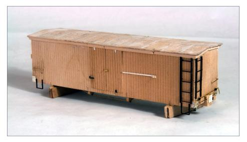
20. Details around the door area included a Grandt door latch, some paper and wood bits, and a track spike for the lower retainer. Prototype photos showed ornate metal parts for these. I had considered laser cutting or 3D printing to make these. When I saw how tiny they were on the scale drawing, I decided bits of card stock were more than adequate.
