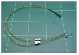
29. Completed dwarf signal with wires and resistors.
