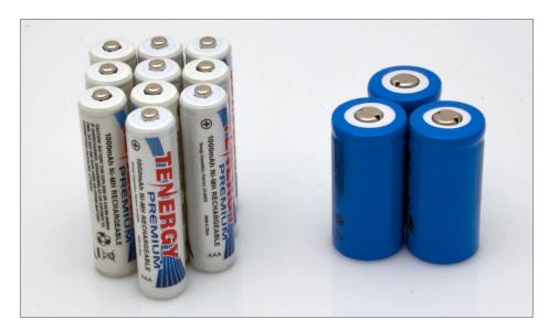
1. About 12 volts and 1000 mAh of storage: ten AAA NiMh cells or three (shorter) lithium ion cells. *Bruce Petrarca photo*
