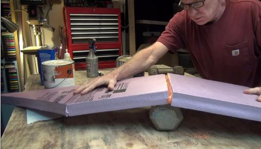
7. I wanted to break the glue joints to understand the strength and pressure required. so I placed the Foam Pro section on top of a dumbbell and pushed the sides down, breaking the glued joint fairly easily.
