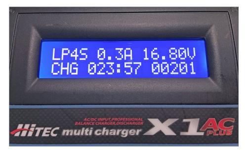
6. HiTEC multi charger X1AC+ topping off the charge in a pack. This display shows: Lithium ion 4 cells (LP4S); charging at 0.3 A; with a battery voltage of 16.80 V; it has been charging (CHG) for 23 minutes and 57 seconds; 201 mAh have been added to the battery. *Bruce Petrarca photo*
