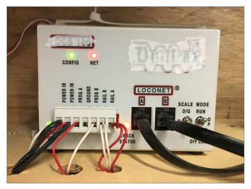
2. This is the Digitrax DCS 100 command station right before I replaced it with the NCE Power Pro command station. I took this photo so I could remember how the wires had been connected. I also compared the wiring layout with the PH-PRO-R to make sure the same connections would work.
