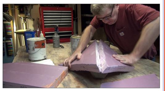
8. The Gorilla Glue joint was much harder to break. I am sure it took more load to break than a modular layout would ever see, making this Gorilla Glue a sure bet to allow me to move forward with this project.
