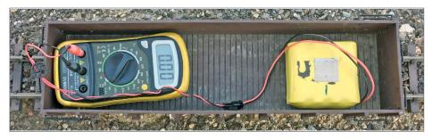
3. Battery pack and multimeter set for 10 amps running in trailing gondola to verify locomotive current draw. *Bruce Petrarca photo*
