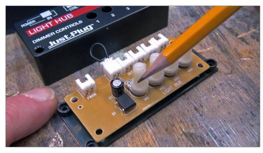
3. Looking inside the light hub I found a capacitor and a rectifier along with other well-thought out electronics which filter the current to the lights along with converting the AC power to a smooth DC current of 16.3 volts.
