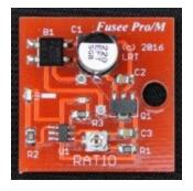
**Logic Rail Technologies** has released the Fusee Pro/M, a track powered warning device intended to enhance model railroad operations by replicating prototype practice. The device realistically emulates a railroad fuse, or flare, as used by real railroads to protect the rear end of a stopped or slow moving train. The Fusee
