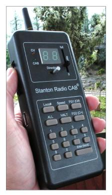
The S-CAB system operates on the 916.48 MHz frequency common to Linx boards. This makes for compatibility between the S-CAB system and others. For example the controller function could be from either an S-CAB Throttle or a TVD DRS1 transmitter. A CVP T5000 cab will work as well, using its channel 16 setting. Again, there is the interference issue with this frequency. However, the S-CAB
