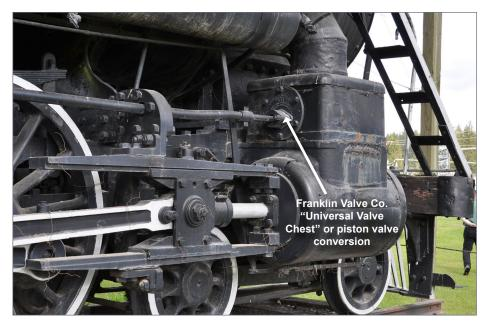
19. My prototype had an upgraded valve gear by Franklin Valve Co. I set about fabricating a new cylinder assembly to match this.
