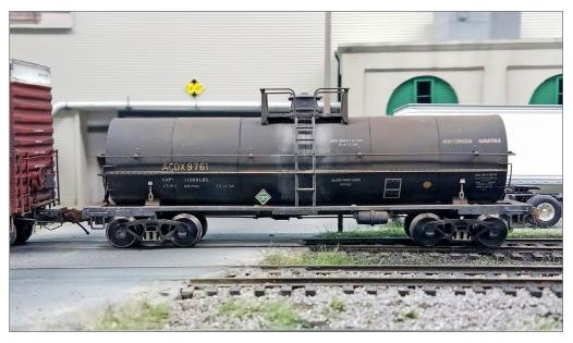
4. Neil Schofield also modeled this car following behind the MILW appliance car. This is an Atlas 11,000-gallon tank car of anhydrous ammonia headed to a local fertilizer distribution plant. The car represents an early version tank car with full-length walkways. It's an Atlas factory-painted car with some airbrush weathering, chalks, and artist oils to replicate 30-plus years of service.
