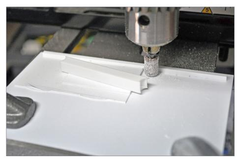
20. I built my new cylinders from styrene. I used a small Dremel sanding drum to form the proper concave curves in the square styrene tubes that would form the valve chests.
