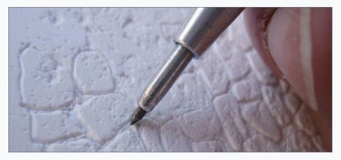
8. A standard steel scribe has many modeling uses. Here I'm using it to scribe the mortar lines on a stone wall.
