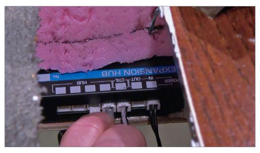
17. After the glue cured, I plugged the AC transformer in the expansion hub, along with the rocker switch connecting plug and two connecting cables that will run to each light hub.
