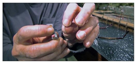
19. I twisted the fine wires, grouping three lights at a time and inserted these wires into the linker plugs supplied with the lights. Simply press down the buttons and insert the wires into the plug matching the color-coded polarity of red to red, and black to black.
