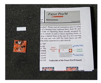
4. The Fusee PRO/M comes with the board, complete instructions, and an small piece of 0.020" styrene (optional) to help align the board and keep from shorting the rails when you place it on the track.
