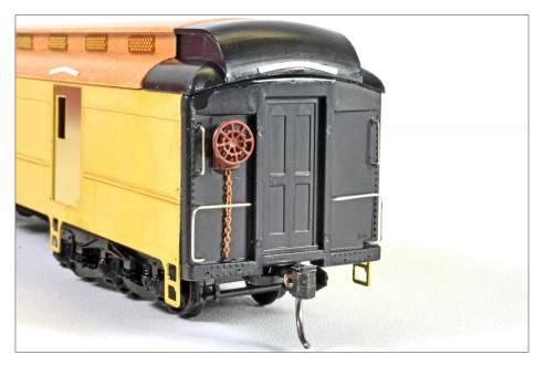
14. The plastic end has a plethora of grab irons, along with a brake wheel and drip strip.
