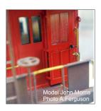
**Black Cat Publishing** has etched brass storm doors for both Canadian National and Canadian Pacific wood sheathed cabooses. CPR prototype doors had two window panes which were replaced in the summer with screens. CNR's wood storm doors have four
