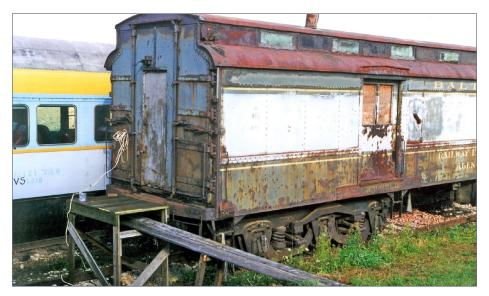
24. A close-up of 749's end doors. It is unknown if the large pipe on the roof was installed later, or existed when the car was in service.
