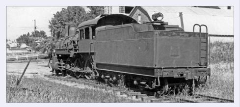
35. In temporary storage behind the Potlatch depot, we get a good view of Number 1's tender. Originally built with a coal bunker, it was converted to an oil bunker in 1912. During WWI, the engine was switched back to burn coal, and then re-converted to oil at the end of the conflict. *Ivan Ergish photo, WI&M Ry. HPG collection*
