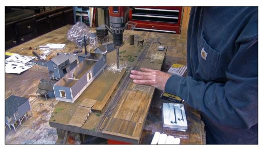
24. Using a 3/32-inch bit, I drilled eight holes through the <sup>3</sup>/<sub>4</sub>-inch plywood base to accept the lamps. I also drilled <sup>1</sup>/<sub>2</sub>-inch holes in the scene to feed the wires up to the buildings.
