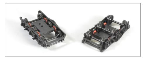
8. The Branchline trucks are assembled with minor modifications – Kadee red washers space the side frames out from the central span piece to keep the Kadee wheelsets from binding, and the rear brake beam is left off to avoid interference with the center sill.
