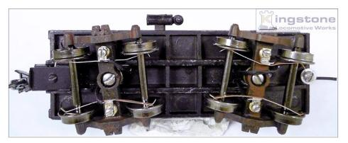
2. Bernd's design uses phosphor bronze wire and picks up directly from both wheels, creating a current path with as few wiping contact points as possible.
