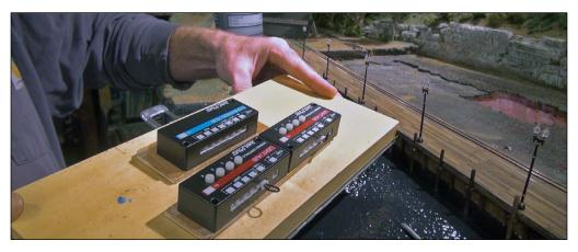
14. I used Gorilla Glue to attach two light hubs side by side in a piece of plywood. The expansion hub was also attached to its own piece of <sup>1</sup>/<sub>4</sub>-inch oak plywood. I set this aside for 30 minutes until the glue cured.
