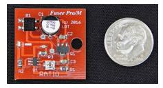
3. This gives you an idea of the Fusee PRO/M's size. It can sit across the rails from S through Z scale, and is powered directly from the rails. It will also work in O scale if you place it diagonally across the rails. territory. A railroad fusee is timed to burn for ten minutes and they are dropped behind a train to ensure a safe spacing. If a following train encounters a burning fusee it is not to pass until the fusee burns out.
