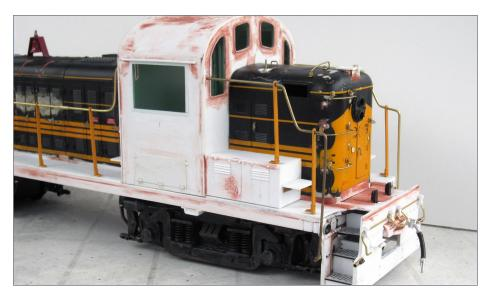
7. The RS-3 was extensively rebuilt, with a new cab, deck, pilots, handrails, and other details..
