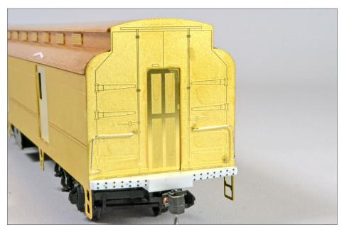
15. The brass end has fewer grabs, but Archer rivets, which shouldn't be added until immediately before painting.
