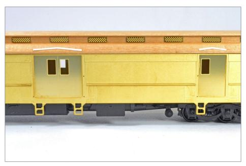
16. Drip strips are formed from styrene strip, and glued to the roof above each baggage door.
