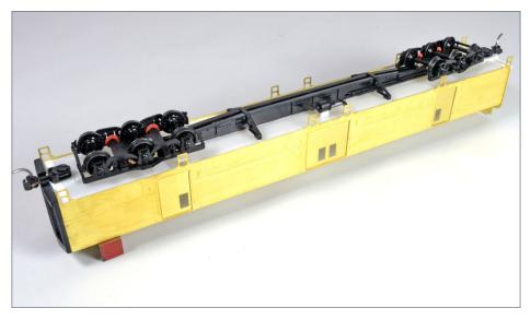
10. The center sill, air brake cylinder, trucks and couplers mount onto the carbody Note that the brake cylinder points to the brass end.
