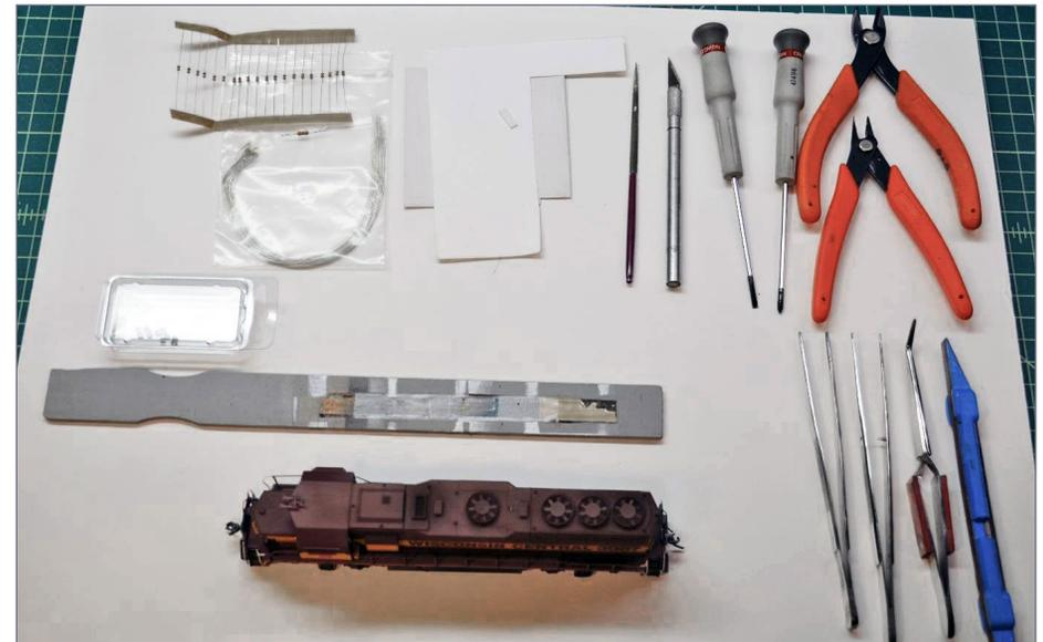
1. Various tools used for ditch light installation. Also needed are a soldering iron and multimeter.
