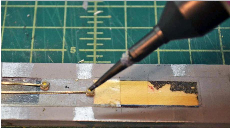
6. Testors Glue for Windows secures the LEDs in place.
