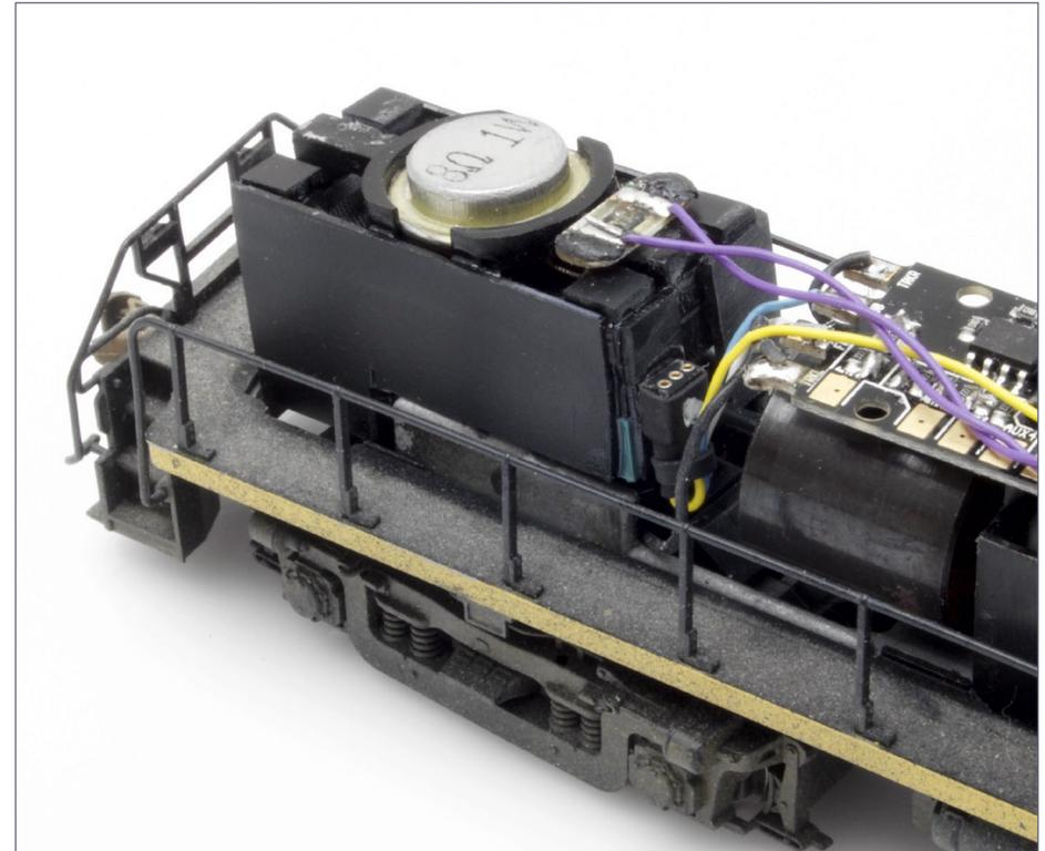
15. Detail view of left side of speaker baffle showing 3-pin lighting connector glued to the the side. The white dot on the side of the lighting (female) connector needs to be aligned with the similar dot on the male connector coming from the shell to get the correct lights on for the loco direction.
