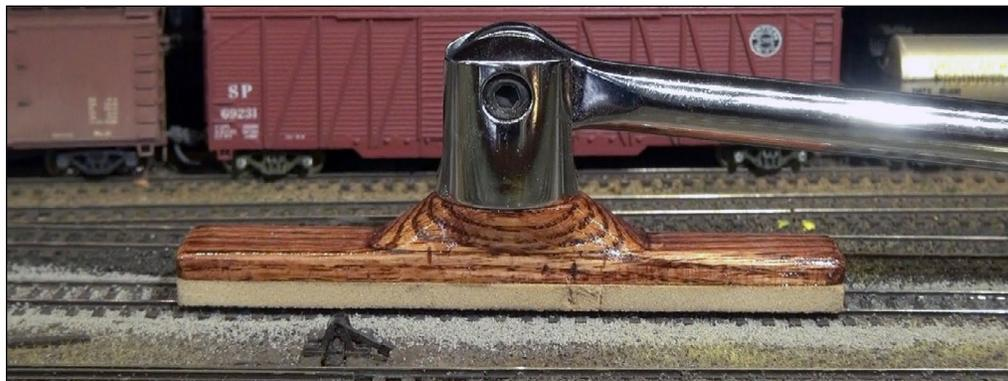
2. Last month I talked about tipping over the breaker bar with the higher center of gravity. It wasn't working very well with the two and a half inch long head. I suggested using a six-inch head instead, as this worked with the higher pivot point found on a lot of breaker bars on the market. Well, the six-inch head turned out to not be very functional on HO scale right of ways.
