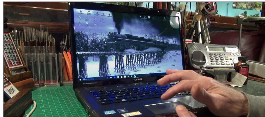
21. The last step in the process was to connect the laptop computer to the DCS 240 through the USB cable. Upon launching Decoder Pro, I got a prompt that COM 3 Port was not found. Upon further investigation by checking my computer's device menu, I found the DCS 240 wanted communicate through the USB COM 5 Port.
