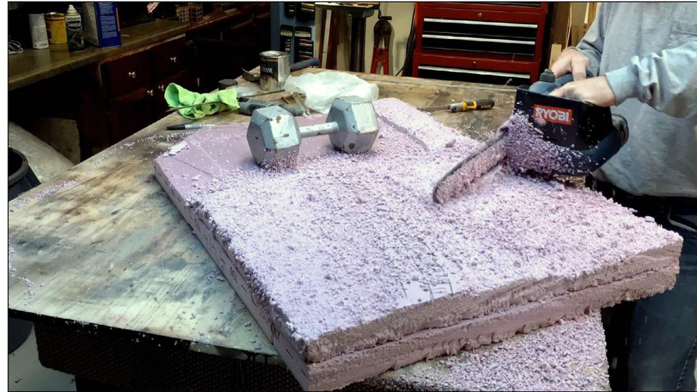
27. I carved the topography on the foam scene using a pruning saw, a chainsaw and a Stanley Surform planer, working my way around the diorama and checking measurements for the bridge's placement until everything looked prototypically accurate to create a realistic looking scene.
