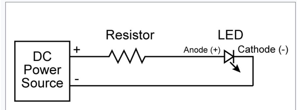
would limit the current exactly the same if wired between power source's negative terminal and the LED's cathode pin.
