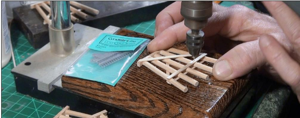
35. Using a #65 drill bit in a drill press, I drilled holes in 11 locations on each side of the trestle bents where the bolts would hold the structure together. I then glued Grandt Line 2½ inch bolt castings into each of the bolt locations.
