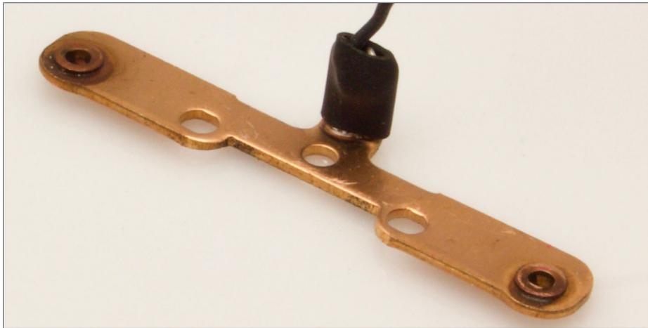
8. The truck side frames with wire soldered and shrink tubing providing some strain relief.
