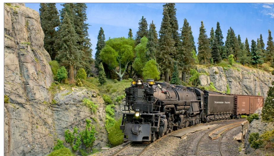
1. An Athearn Genesis Z-8, weathered to be a workhorse, drifts downgrade through Cascade siding on Mike McGinley's "Southwestern Pacific" freelance 18'x22' layout. The image is a Helicon Focus stack of exposures taken with a Canon XL resting on the track. The main line is 36" radius superelevated Precision Scale code 83 flex track, the rock formations are carved blue polystyrene insulation board, the trees are commercial products, and the sky is painted on the wall.
