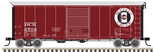
Like the prototypes, the HO scale ready-to-run models will have a variety of details such as three end styles (4/4 Murphy, early and late Improved Dreadnaught), two roof designs (diagonal and straight panel),
