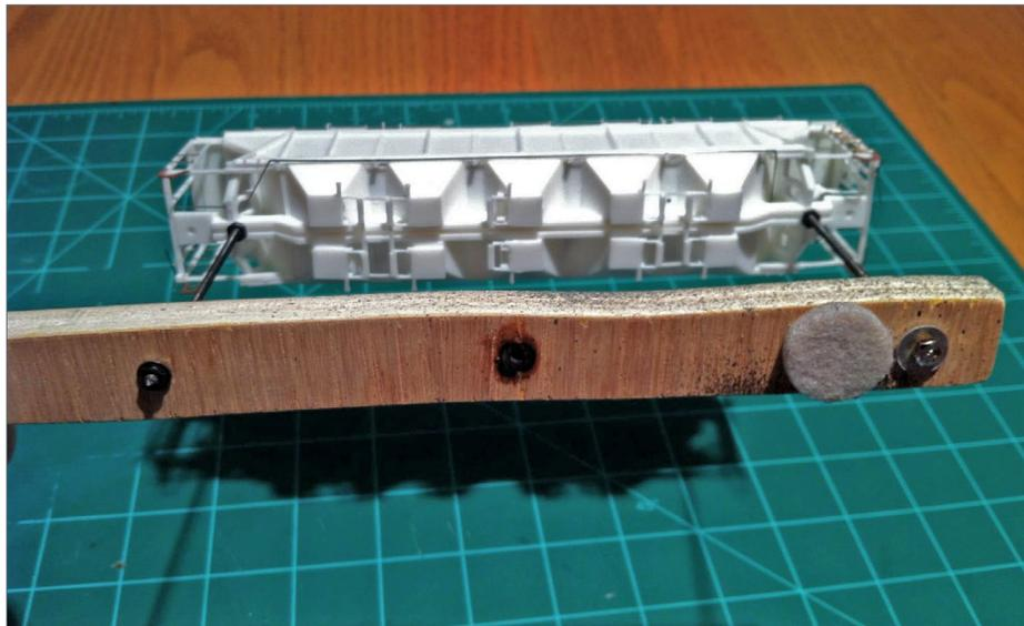
3. Threaded rods screw into the truck mounting bosses and can be spaced to fit different models by drilling new holes. The foam or fiber pad allows the holder to rest on the workbench.
