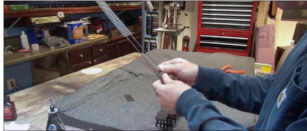
43. I peeled the ties off of a piece of code 70 Micro Engineering track the length of the bridge. This rail will lay flat atop the bridge deck, giving a smooth transition from the land to the bridge.
