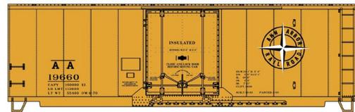
New HO scale car kits available from **Accurail** include this 40-foot Ann Arbor insulated plug-door boxcar. The model is based on a prototype built in 1950 and rebuilt in 1970.
