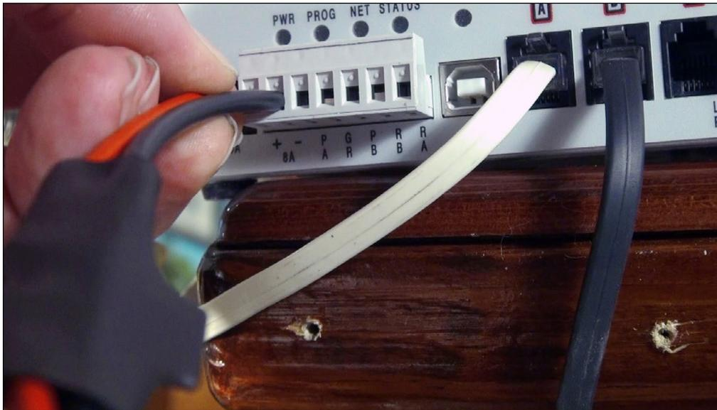
18. I hid most of the power wires' length under the shelf. They emerge just where they attach to the DCS240 terminals with screws. You can also see the five-amp automotive inline fuse covered in black shrink wrap.
