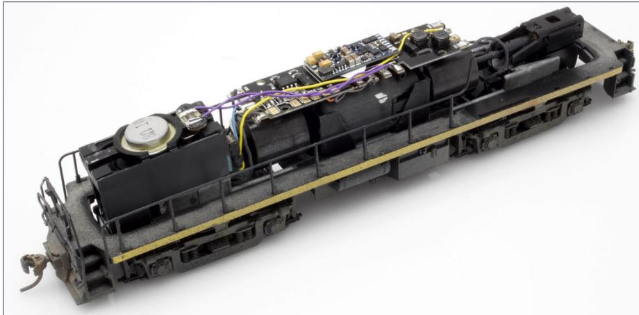
14. The finished frame, ready for shell installation. The lighting connector was plugged together with the white and yellow wires oriented to be together.
