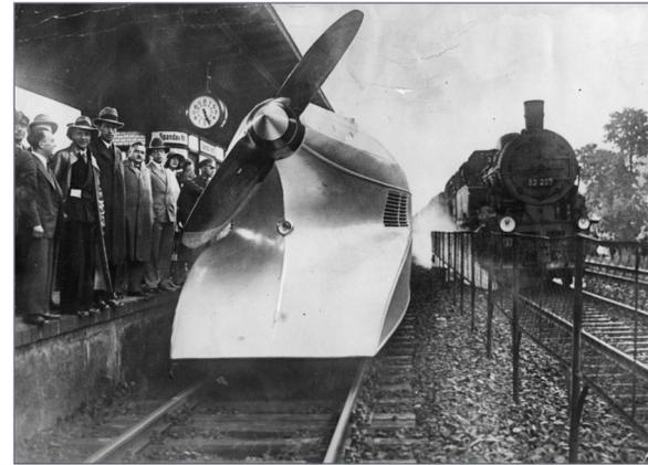
The Schienenzeppelin, was designed by German engineer Franz Kruckenberg in 1929. Made to look like a zeppelin, the Schienenzeppelin reached a world record speed of 143 mph. ■
