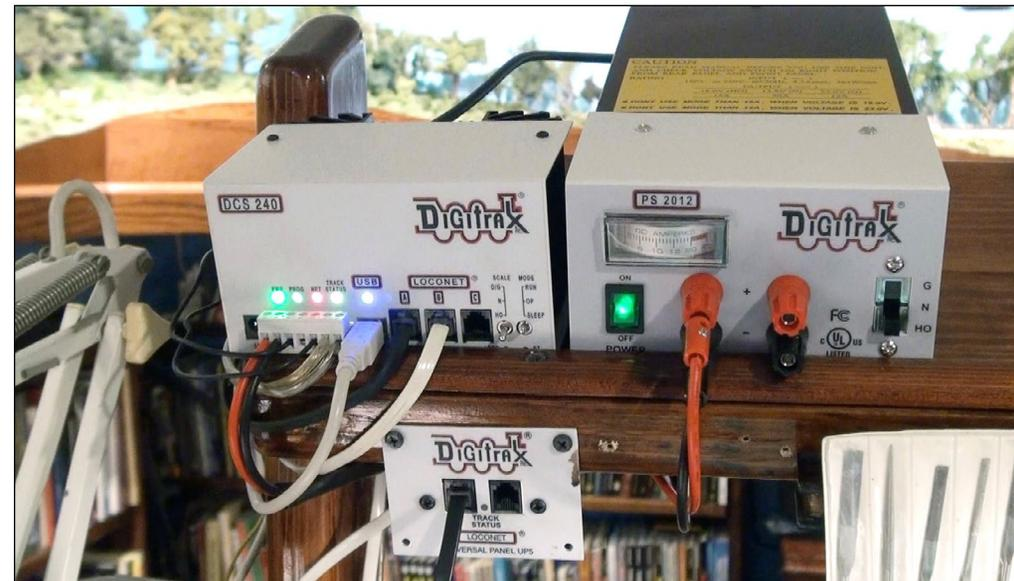
23. In a future month, we will separate the layout into 14 power districts for signaling, but for now I have made a good choice upgrading my DCC system with the new Digitrax DCS 240 and a new power supply providing my layout with a solid 14+ volts to the system, not to mention the pretty rainbow of LEDs lighting up the front panel of the Digitrax DSC 240. It should last me another 17 years of reliable use on my layout, as my DCS 100 did.
