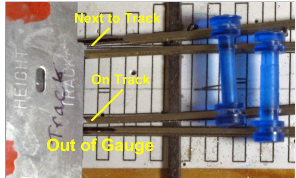
12. NMRA gauge at the points doesn't fit. Time for more adjustments: keep working until things are perfectly in gauge.
