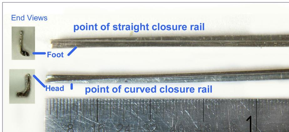
13. Top and end view of point closure rails before soldering.
