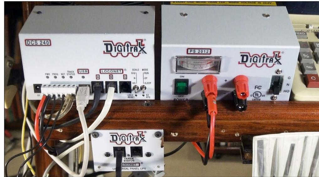
19. I attached the programming track wires, the LocoNet 6 conductor jacks, and the USB cable. That finished the hardware installation. With the power supply turned on, the DCS-240 lit up with colorful LEDs and sounds immediately started coming from my train on the main line. I turned the knob on my throttle and the train started running, just like that.
