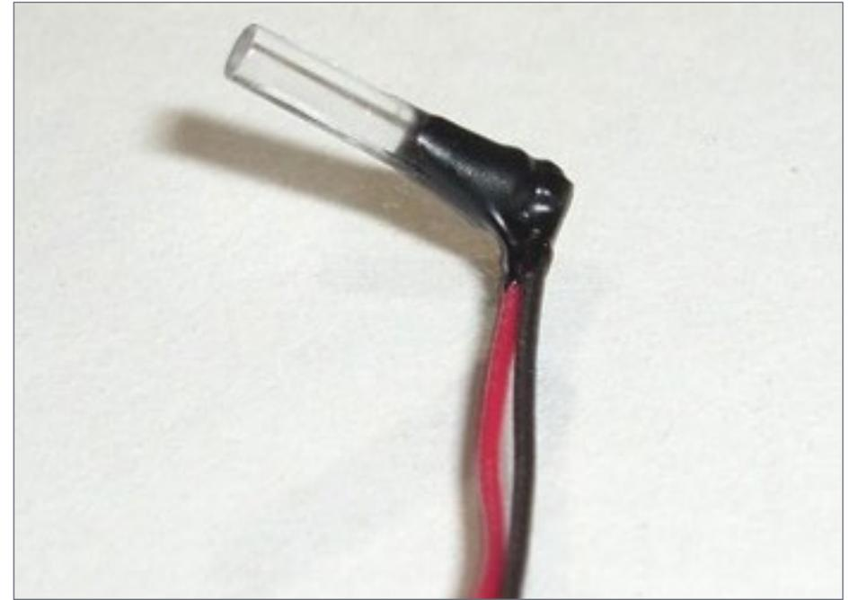
3. LED mounted to a clear light pipe from Streamlined Backshop. Designed to fit Athearn openings, they work just perfectly in the Atlas/Kato. *SBS4DCC photo*
