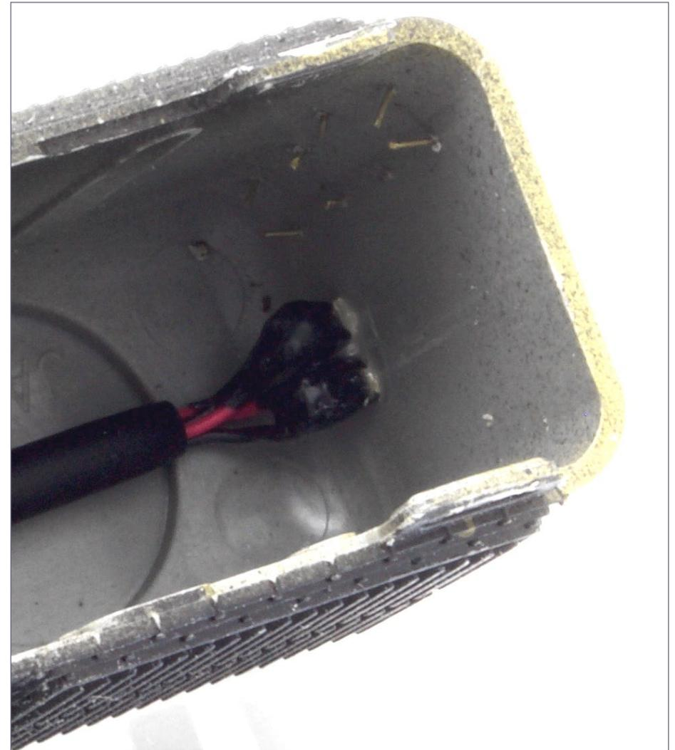
9. Detail of the installation of the LEDs in the long hood of the RS3.
