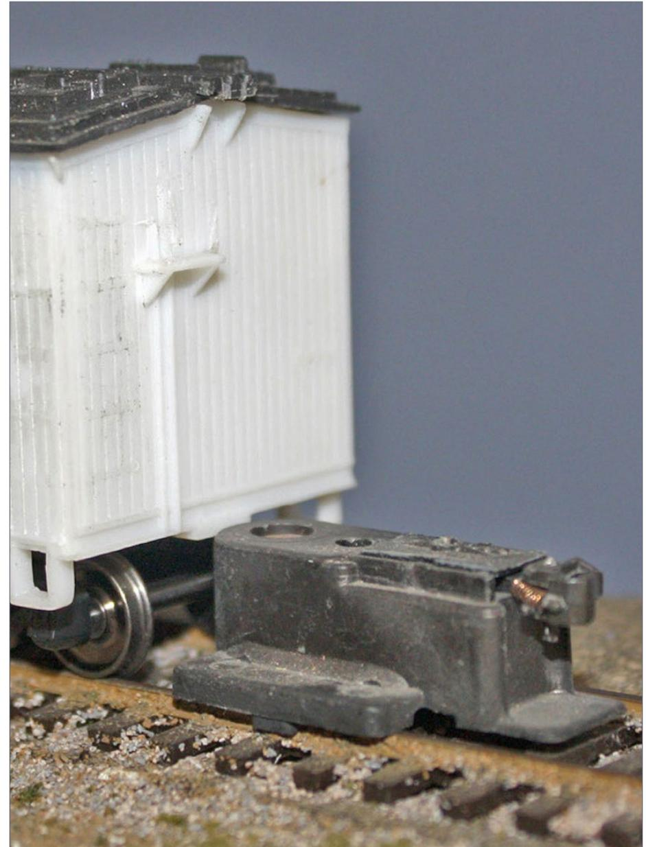
2. Here the back of the Kadee height gauge shows that the coupler pad on this car body is a little too low.
