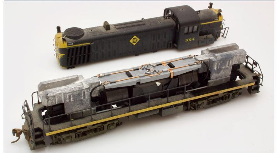
2. The interior of the Atlas RS3, showing the single centrally located bulb. The light pipes are inside the shell and not shown in this photo. The weights sitting on each end of the frame are not attached to anything. They are wedged into the shell when the loco is assembled. I call the assembly in front in this photo the "frame" and the one in back the "shell".
