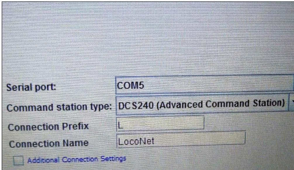
22. This meant I had to program the preferences setting in JMRI Decoder Pro to match the hardware. I did this using the multiple-choice dialog box in Decoder Pro's preferences settings. I set the serial port to COM 5 and the command station type to DCS 240 Advanced command station. Just like that, JMRI Decoder Pro program opened on my laptop with a green icon indicating that I can now program decoders and run trains using my computer interface.
