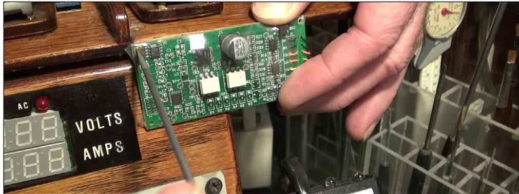
14. I removed the PTB-100 power booster for the programming track and the eight or so wires associated with that, making the wood power box look better without the electronics screwed to the front of it.
