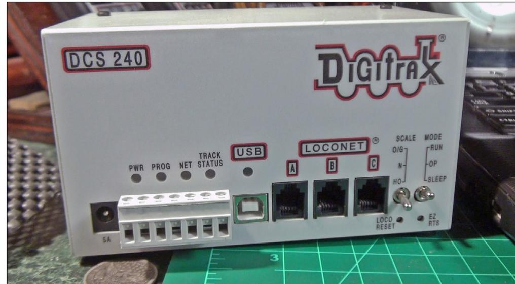
9. This month we look at the new DCS 240 power command station. I really like the new features included in this unit, like the USB port which will allow me to eliminate my Digitrax PR3 and all the wiring associated with that. It also comes with a built-in power booster for the programming track and means I can eliminate my Soundtraxx PTB-100 programming track power booster and all the wires attached to that. It is also convenient to have three Loco-Net jacks on the front panel.
