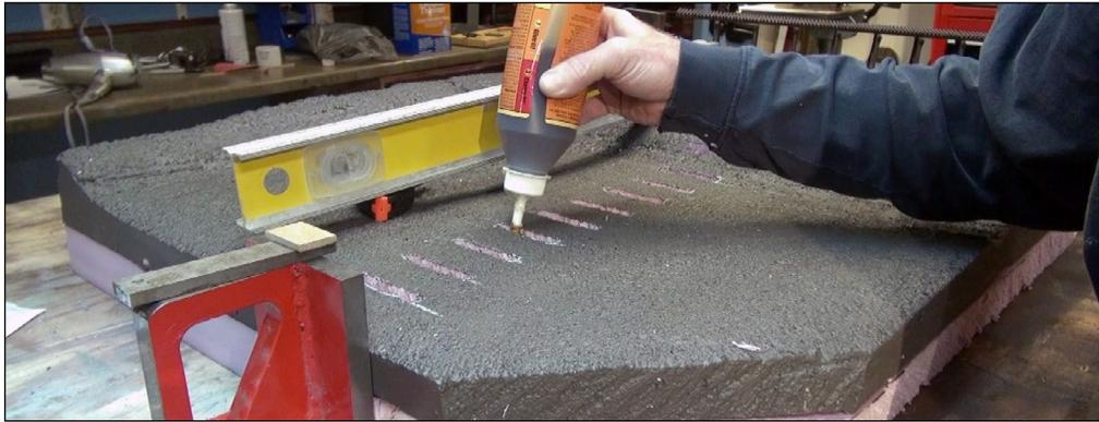
41. I filled the grooves in the foam with a bead of Gorilla Glue. I then placed the bridge on the scene, sinking it into the glue, and lining things up level and straight using a steel block on one end, and shimmed a little to make everything level.
