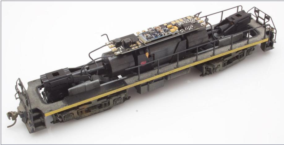
12. Decoder and motor wired. Now is the time to test the loco on the programming track.
