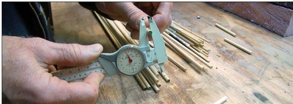
29. Going through my dowel rod stock, I looked for poles with a scale diameter of 13 or 14 inches. 3/16th-inch dowel rods fit this bill. I sanded the poles lengthwise with 80 grit paper, cutting wood grain into the dowels and decreased their diameter to about 12 scale inches.
