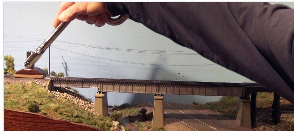
7. When you flip over the reversible head, the tool offers a very powerful feel. I can exert a lot of pressure on the track with the grip offered in this position, as the handle lines up well with the arm for accuracy and stability.
