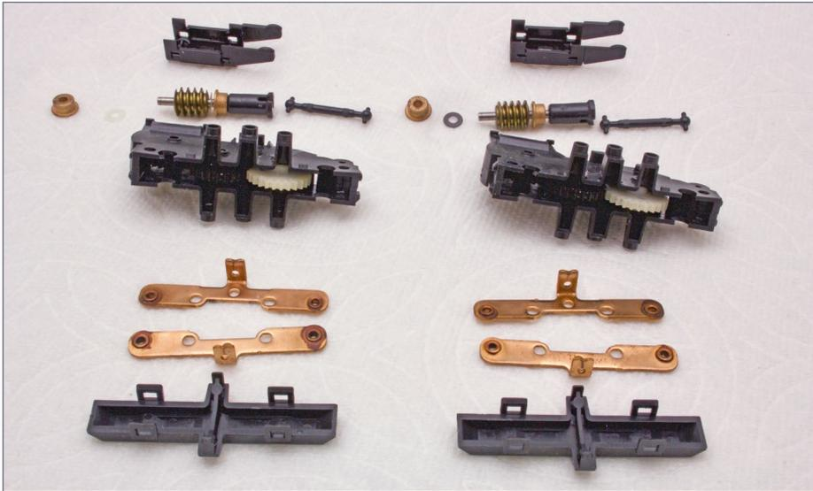
6. The parts of the loco drive train after cleaning. They are laid out drying on a paper towel and organized like an exploded view. Note the (new) black thrust washer near the right gear. There is an original (white to clear) one that is barely visible next to the left gear. These guys are easy to lose. That's why I ordered extras.
