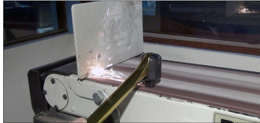
3. I had to redesign the tool to lower the center of gravity and did this by grinding down the square tip of the breaker bar to the spring-loaded ball. A belt sander or bench grinder will work for this. Keep a bowl of cool water on hand for this process.
