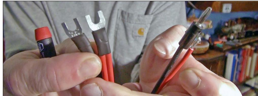
16. I modified the Digitrax power harness, removing two of the four wires but keeping the inline fuse in place. I cut off the crimped-on wire connectors and replaced these with banana plug jacks.
