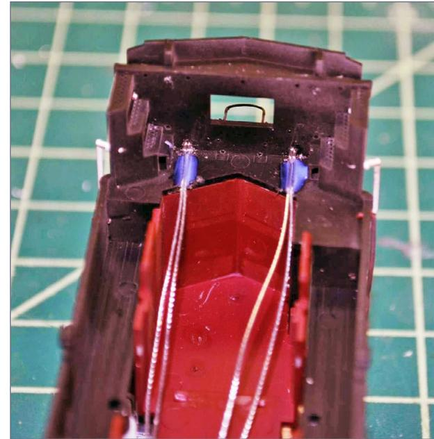
10. Wires routed and glued into their channels.
