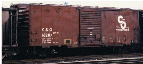
**Kadee** plans to release a Chesapeake & Ohio PS-1 boxcar with 10-panel welded sides, narrow bolster tabs, and 8-foot Youngstown sliding doors
