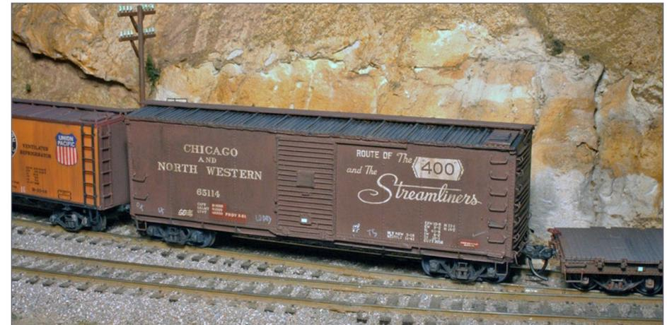
14. This Sunshine box car has fresh paint patches both for its reweigh data, and for its repack data over the right truck. Note in this case that all weight digits have been replaced, unlike [13]. Note also the route card on the door. The flat car at right has one too.
