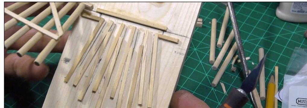
31. To build the jig, I glued HO scale switch ties to the jig surface, placing them on each side of the dowel rods leaving no space for movement or slippage. After the glue started to set up, I carefully removed the trestle bent from the jig, revealing my new trestle building tool.
