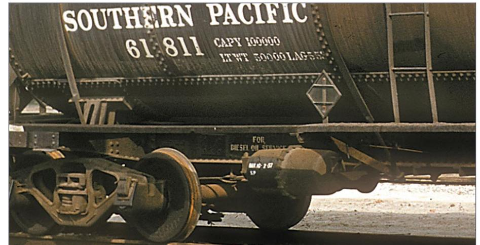
17. This detail from a photo of a Southern Pacific tank car with its reservoir readily visible shows the fresh stenciling for brake servicing. Tank cars often show brake stenciling very prominently because of the reservoir location. *Bruce Petty collection*
