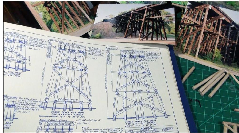
30. Checking through prototype photos and dimensions taken from prototype railroad standards books, I handbuilt the first trestle bent piece by piece. This first bent was used to make a trestle building jig.
