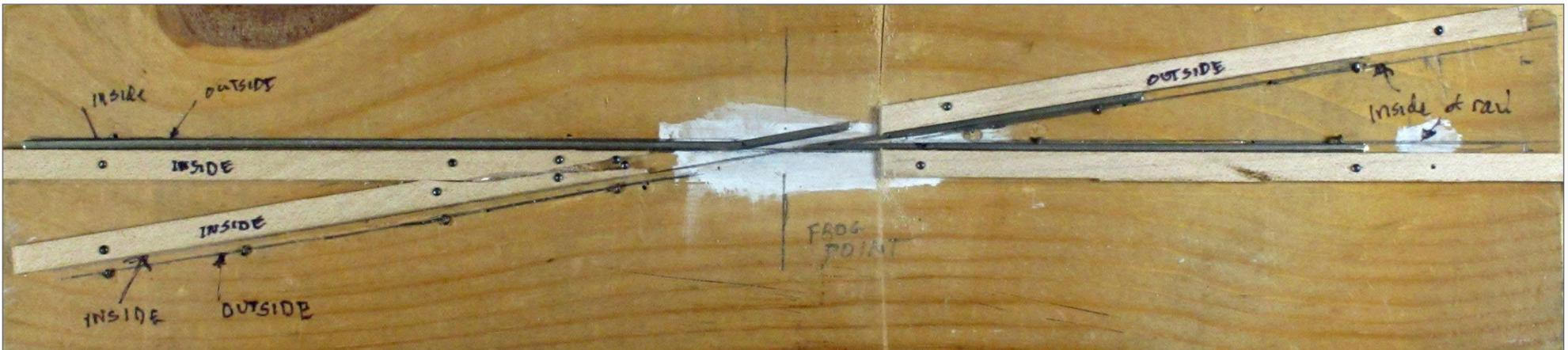
5. Frog assembly fixture with frog point and one closure-wing rail.
