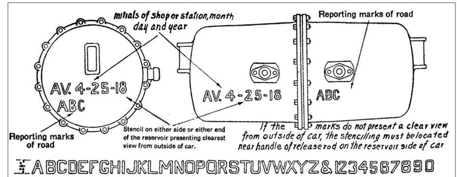
16. This is the 1952 AAR drawing showing arrangement and location of lettering on the reservoir to document date and place of brake servicing. Note that the reservoir end would be stenciled if more visible.
