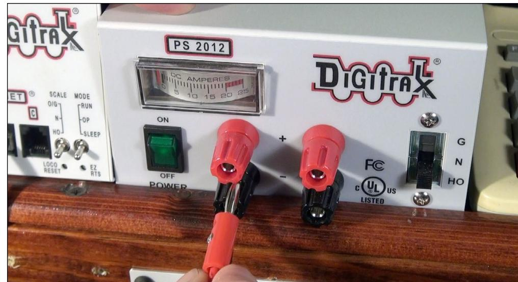
17. These banana connectors plug in to the power supply's front power jacks. Matching the red to positive and black to negative is easy and fast.
