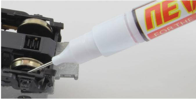
16. Applying Never-Stall lubrication to the rolling contacts on the loco trucks.
