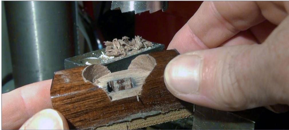
4. I then cut a bigger hole in the wood block to accept the breaker bar's round head. This lowers the tool's high pivot point and moves its center of gravity closer to the track.
