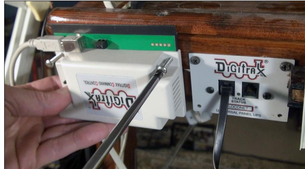
13. To start the DCS 240 installation, I needed to un-wire and pull everything apart. I started with the Digitrax PR3 which was attached to my bench with wood screws. I moved the Digitrax face plate about eight inches to the left to open up more space.
