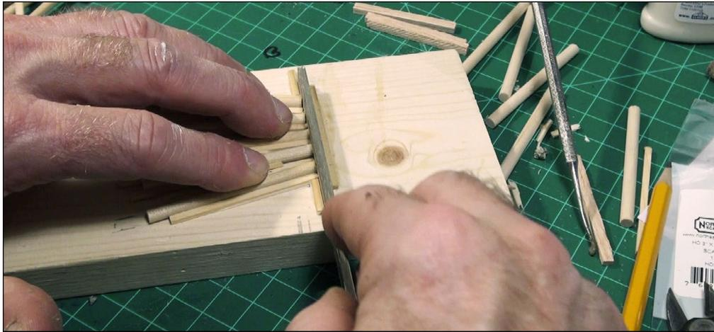
32. To build a trestle bent using the jig, I placed five dowel rods into the jig's grooves. I filed the tops of the poles so they would match up flush with the 14-foot-long top cap.
