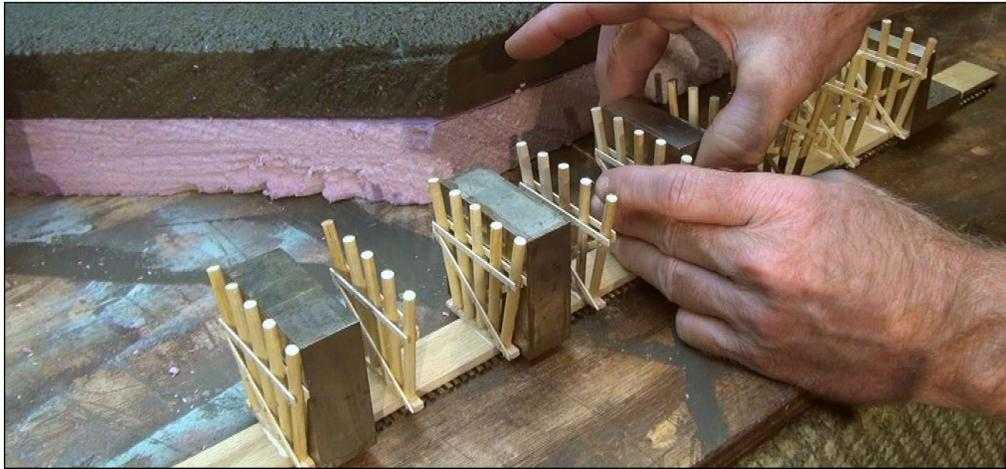
37. I glued the finished trestle bents to the bottom of the bridge deck on 14-foot centers using wood glue. I also used steel blocks to ensure everything was square as the glue dried.
