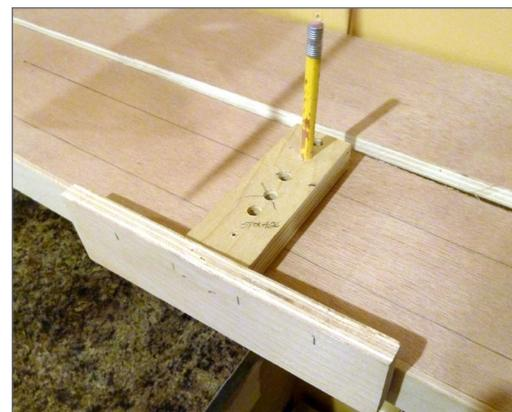
1. Bill made this marking gauge, which is basically a homemade T-square using scraps of plywood he had on hand. Bill drilled holes in the leg of the T to hold a pencil at the correct yard track locations, as measured from the front fascia board.
