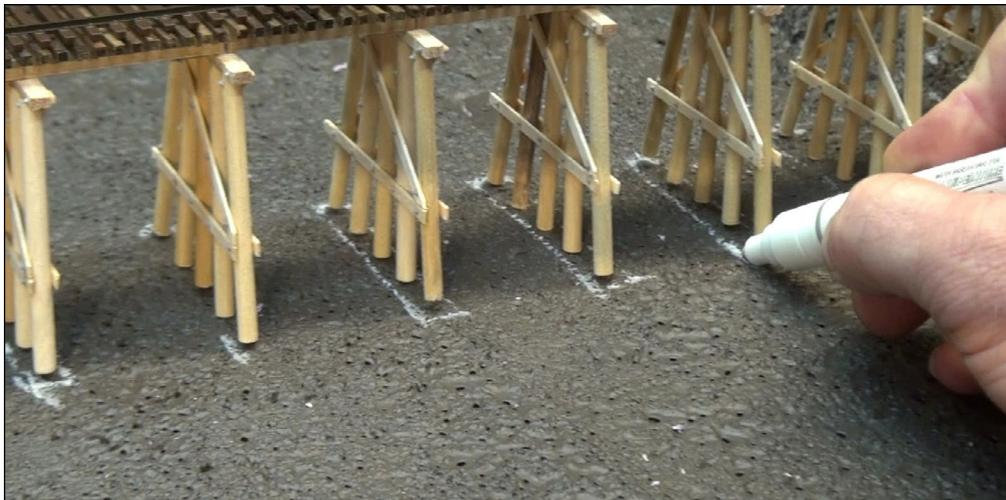
38. I placed the bridge on the diorama and used a white marker to show where the bents would be sunk into the foam scene. I then cut these grooves out with a Dremel motor tool and a router bit attachment.
