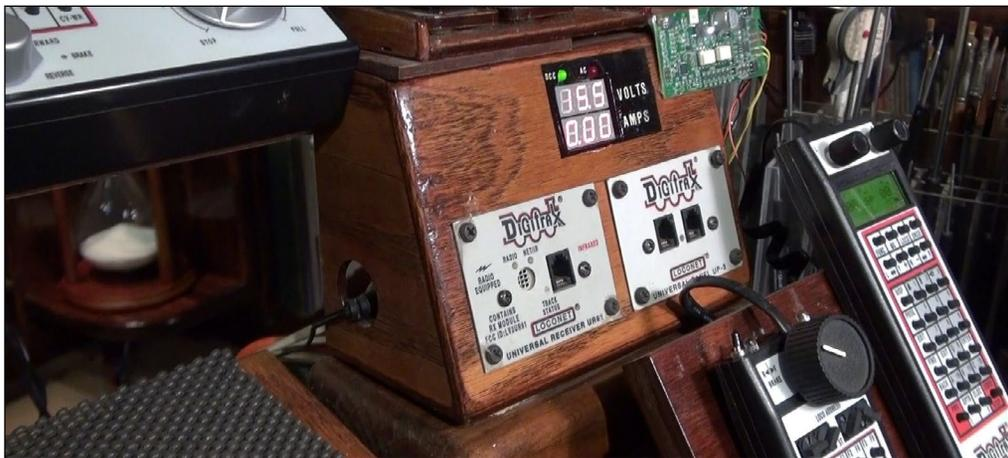
12. I also installed a Digitrax UR91 radio receiver in the wood box to allow good radio reception in that area of the layout room. I stained and varnished the control box to match the layout room decor.
