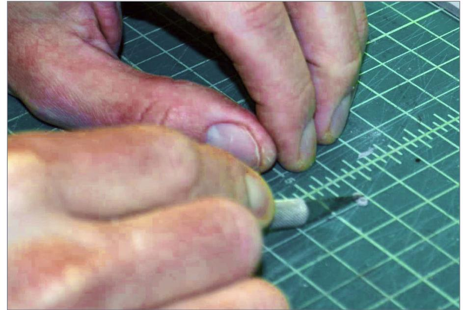
3. A delicate touch and many passes prevent cracking the modified light housings.
