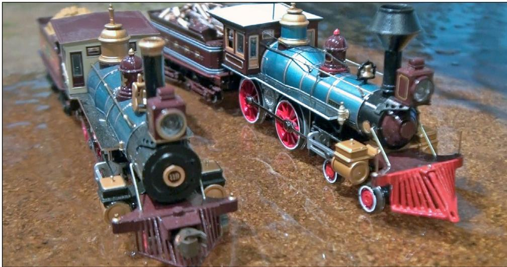
55. A new pilot/cow catcher was added to the model with link and pin coupler bar details attached. A detailed smoke-stack was attached to the boiler, along with flag posts.
