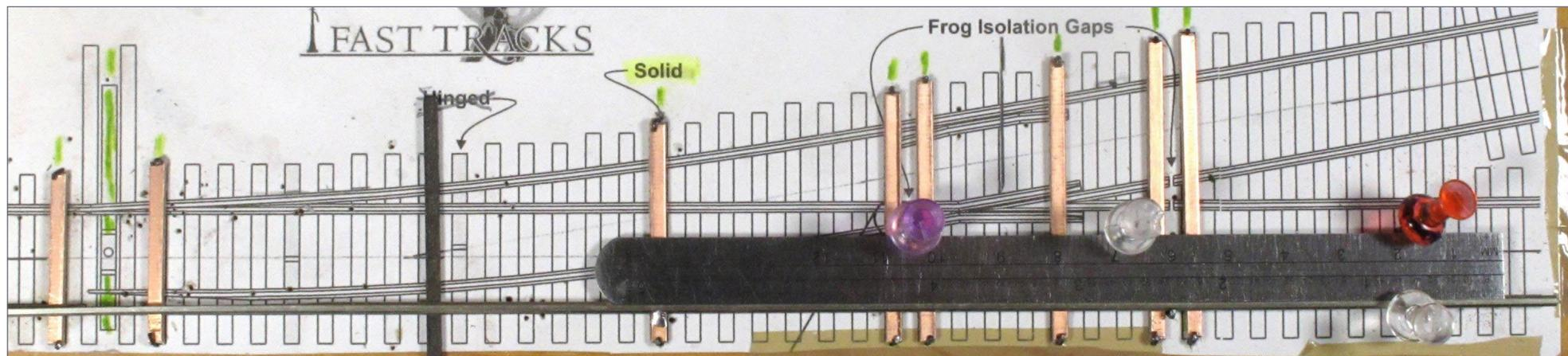
9. Soldering straight through rail to PC ties.
