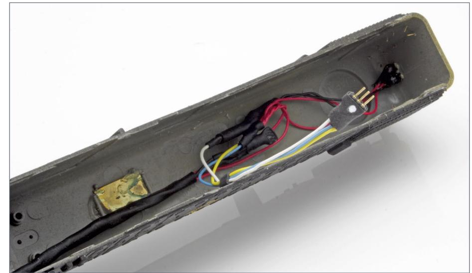
13. The wiring details inside front end of the shell. The brass plate is a heat sink from the original bulb installation.
