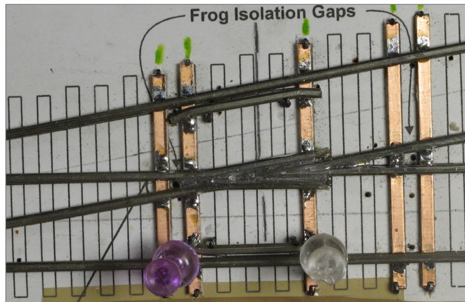
16. Soldering the guard rails in place.
