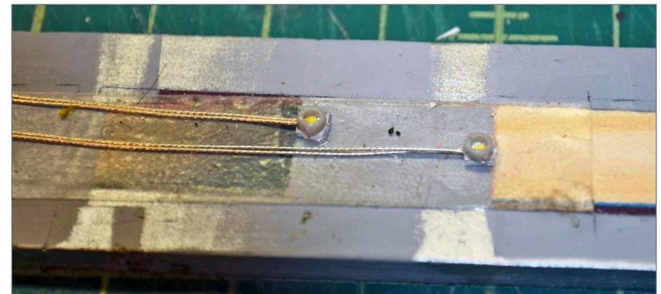
5. LEDs, backer boards and ditch light housings all in one piece.
