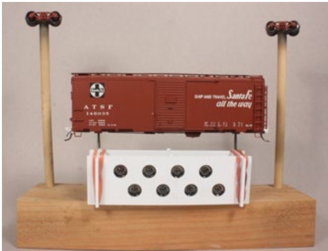
27. As usual, I began with a thorough washing of the car body, trucks and wheelsets, using distilled water for the final rinse to eliminate mineral residue. After air-drying, I mounted the components in painting jigs to apply the matte finishes, and handled the model only with thin, powder-free gloves.
