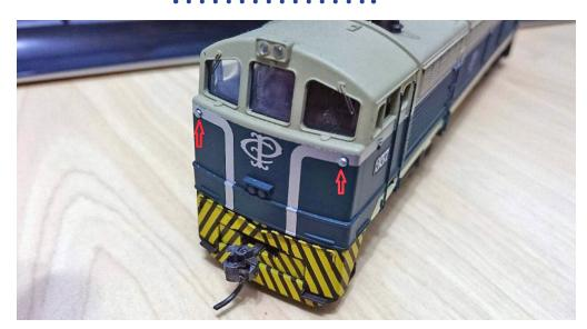
2. So far, lighting descriptions by other modelers have usually referred only to the lights that illuminate the front of the locomotive. Modelers use white or yellow microLEDs for these but have ignored these small rear red lamps, for understandable reasons. The technique presented here uses optic fibers and considerably expands the arsenal of tactics for modelers, as it dramatically reduces the size of the light source.
