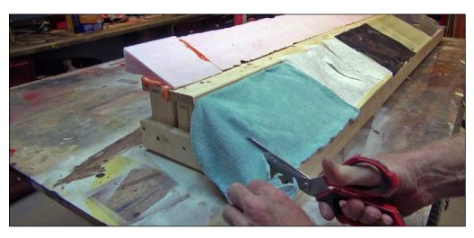
14. In this photo, you see all five sections of the layout with various sub-bases in place: window screen, masking tape, black duct tape, simple paper towels, and blue microfiber cloth. The cloth and wire screen are stapled. The tape sections and paper towels are held in place with tape.
