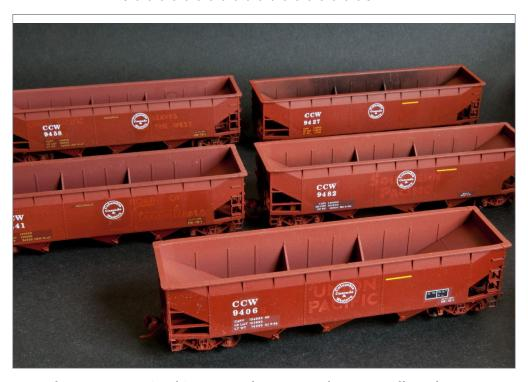
1. The CCW acquired its 26 rock cars on the secondhand market. Some cars got a light spray job with Krylon #1317 ruddy brown primer, and some are Southern Pacific freight car brown. The yellow lines indicate the maximum fill level for crushed rock and gravel. The models are Accurail 7500-series three-bay 70-ton offset hoppers, with Kadee #5 couplers and InterMountain 33-inch wheelsets.
