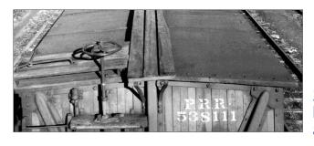
29. Wood running board, latitudinal, and brake step.
