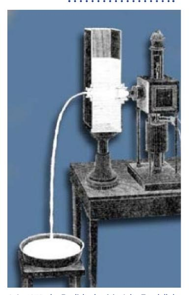
3. In 1870, the English physicist John Tyndall demonstrated the principle of guiding of light by means of a simple experiment. Using a leaky container with water, a bucket and a light source, Tyndall observed that the beam was illuminated through the hole in the container.
