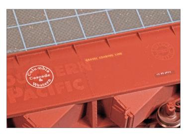
3. Rock is more dense than coal, so a smaller volume makes up a full load in a 70-ton car, and tops out several feet below the top chord. Cars assigned to aggregate loading are marked with a lettered notice or a 4-foot-long yellow line.
