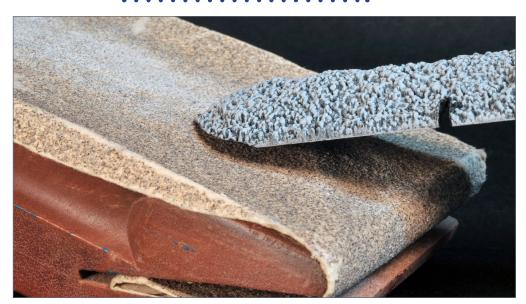
6. To make the load sit naturally in the car at the load line, taper the ends to match the angle of the slope sheets. A cutting tool with a disc, medium grit sandpaper, or a small belt sander will work. The precise modeler with a lot of loads to modify could build a jig and use a saw to cut or grind the angle.
