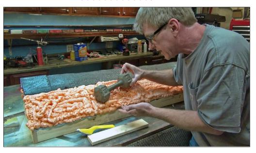
16. After the foam cured, I placed a 10-pound dumbbell to weight each section to see if it would hold up and could be used as a viable way to make scenery. All five sections held the weight without cracking.
