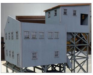
thing is going together nicely and the finish has the "look" that I was aiming for [13-14]. Once the assemblies are glued together, start adding all the detail. The floor is well braced but the walls will probably need bracing to keep them square and prevent warping. After gluing the main building walls together with Titebond, sit it on the base to check the fit. So far so good.
