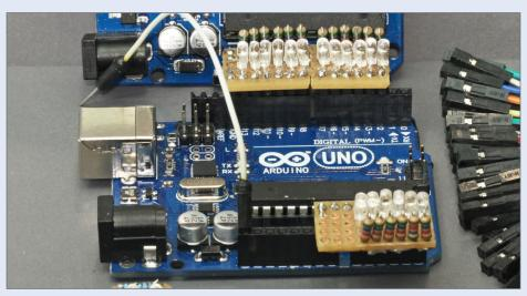
11. I wired all 18 LEDs shown here with 10k resistors, resulting in a total combined current draw for all the LEDs of less than 20ma – well below the Uno's 200ma board limit.
