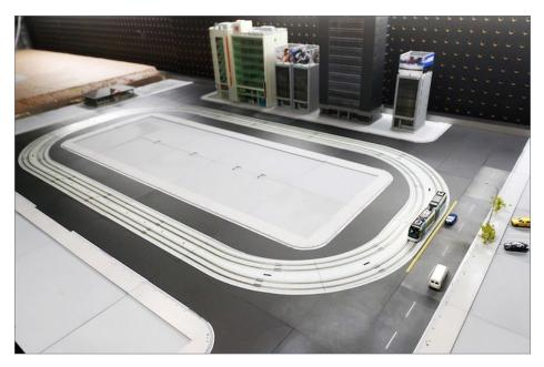
2. An N scale tram system is a major test of track maintenance – rails are buried in pavement, and the lightweight rolling stock has short wheelbases and small wheels. *Metrolink photo*
