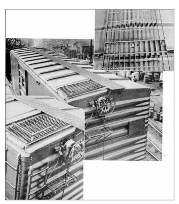
they used a spiral rod to hold the serrated metal strips in position [36]. The Kerrigan, Blaw-Knox and Tri-Lok running boards were all composed of 12 rows of edge-mounted serrated steel. It is difficult to distinguish among the three.
