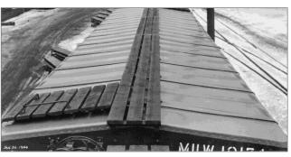
20. Milwaukee Road ribbed-side boxcar built in 1940 with unpainted galvanized steel Murphy double panel welded roof.
