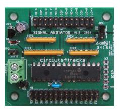
Circuits4Tracks has released a new product called the Signal Animator. It works in conjunction with their Quad Occupancy Detector. The product drives LEDs wired either common anode or cathode and implements speed restriction indications from switch machine inputs. It can be driven by an
