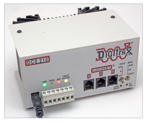
3. The new DCS210 system box is the basis of the Digitrax Evolution system.
