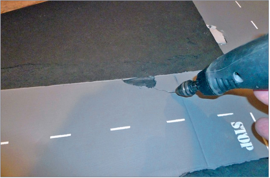
21. A pin chucked in a Dremel tool creates cracks.
