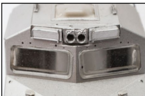
High headlight variant with optional PTC antenna array or antenna dome.
