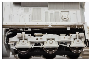
Separately-applied plumbing and traction motor cables.
