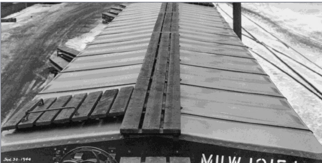
20. Milwaukee Road ribbed-side boxcar built in 1940 with unpainted galvanized steel Murphy double panel welded roof.
