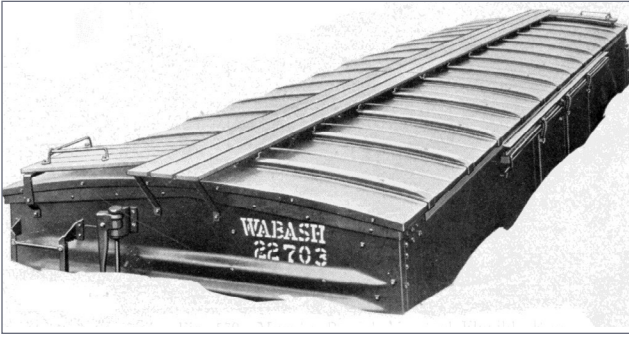
16. Murphy all-steel radial roof manufactured by Stanray circa early 1930s.
