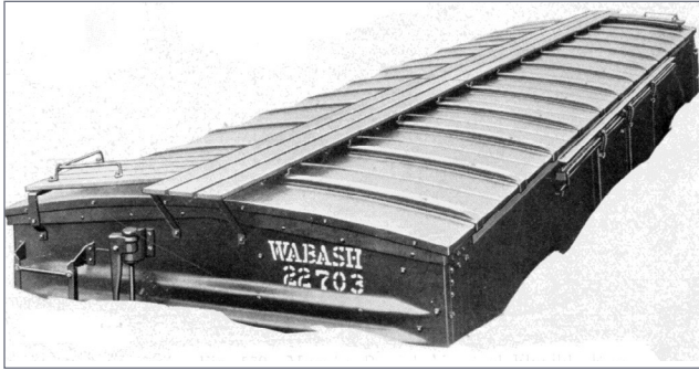
16. Murphy all-steel radial roof manufactured by Stanray circa early 1930s.
