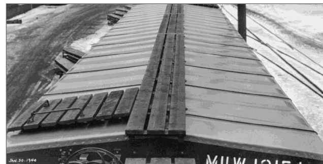
20. Milwaukee Road ribbed-side boxcar built in 1940 with unpainted galvanized steel Murphy double panel welded roof.
