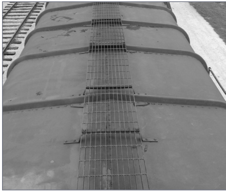
21. Wagon top roof with a Blaw-Knox Steel running board.
