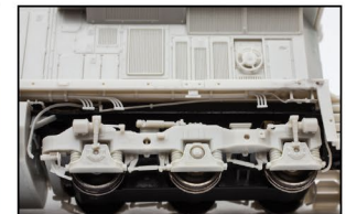
Separately-applied plumbing and traction motor cables.
