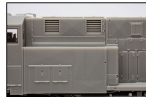
DC style dynamic brake grilles spaced apart.
