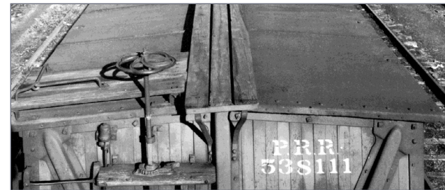
29. Wood running board, latitudinal, and brake step.
