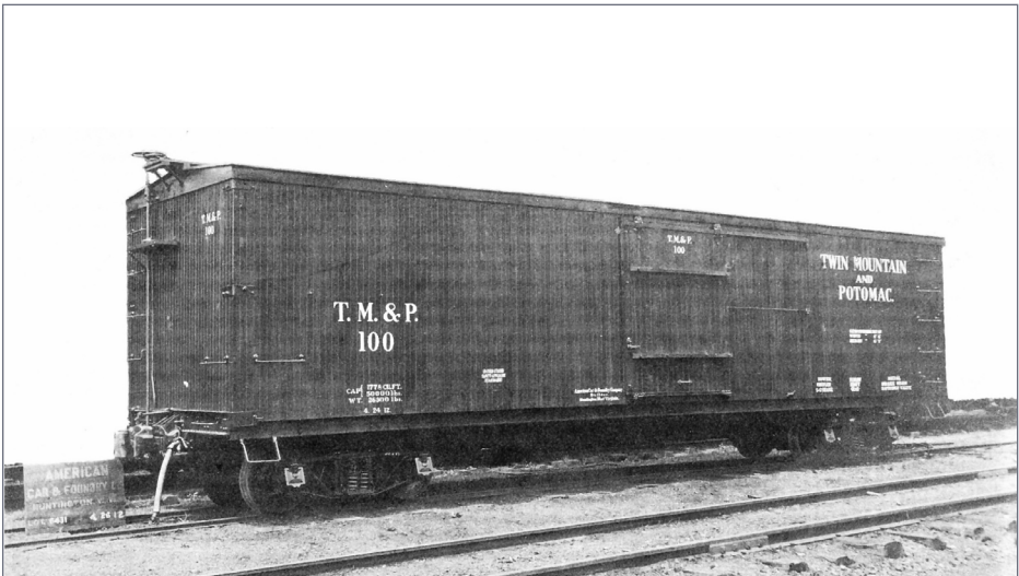
Builder's photo of boxcar #100, one of seven (#100-106) built for the TM&P by ACF in 1912. ACF photo, author's collection LENGTH OVER End Sills 37' 2" Buffers 38' 2½" Inside 36' 0" WIDTH OVER Sidesills 7' 6½" Eaves 8' 7" All 9' ¾" Floor 8' ½" Inside 7' 6" HEIGHT Inside 6' 7" Sill to Plate 6' 4¾" Rail to top of Floor 3' 4¼" Rail to Center of Draw Bar 2' 2" DISTANCE BETWEEN Center Sills 12' ¾" Truck Wheel Base 4' 10" WEIGHT OF Body 20,180 lbs. Trucks 8,040 lbs. Total Weight 28,220 lbs. Capacity 50,000 lbs.
