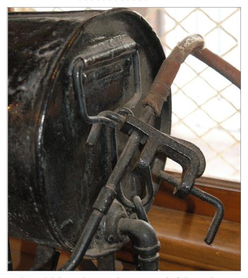
8. The red delivery hose tank on one end of the Keeley is connected to the outlet pipe and valve at the bottom of the tank. The hose is 30 inches long and terminates at the long nozzle and clamp which is hanging on the handle. The clamp let a brakeman attach the nozzle to the front lip of the open journal box and aim the cooling water directly on the hot axle.
