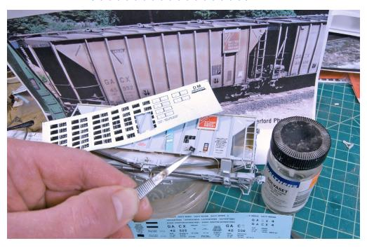
6. I duplicate the prototype lube plates from multiple sets. After I have applied all of the decals, I set the model aside to give the decals time to dry. I then use a new sharp X-Acto number 11 blade to lightly poke multiple tiny holes through the decal film. I apply Solvaset decal solution to the surface. Capillary action allows the liquid to seep under the film and insure a good painted-on lettering look. The ACI plates are MicroScale set MC-4280.
