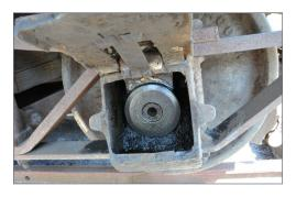
2. Looking into a narrow gauge arch bar truck journal box with the journal box lid raised. The oily waste below the axle bearing surface is visible, as is the axle journal collar. Directly above the axle is the plain bearing.
