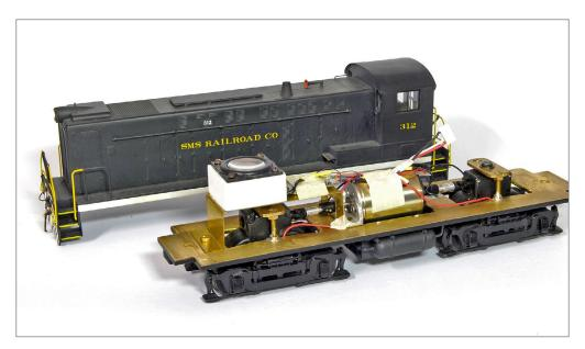
6. This is my Baldwin S12 with Atlas trucks, Faulhaber 2842 coreless motor, and HO LokSound decoder. I scratchbuilt this locomotive – see my blog for more details.
