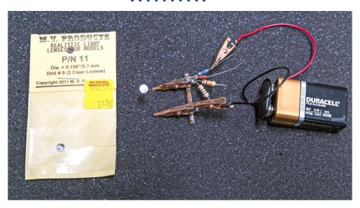
7. The MV Products Realistic Light Lenses come in various sizes. In the center is an example of a 0603 LED glued to the back of an MV Lens. Here I use a 9V battery connected to a resistor to test the headlight, but the brightness may change when powered by a decoder.
