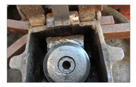
3. Looking up in the journal box toward the bearing. The actual contact surface between the bearing and the axle can seem small, but it covers the entire top surface of the axle and transfers the weight of the
