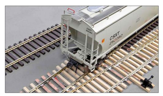
3. The track is a mix of Atlas code 148 flex track and hand-built turnouts. Turnout control is with Caboose Industries HO ground throws.
