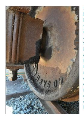
5. Not only oily lubricants but also waste are leaking out of the back side of this journal box. The leaking oil has also covered the area adjacent to the rim of the wheel. This freight car, in service on the narrow gauge South Pacific Coast RR at Ardenwood Historic Farm in Fremont, CA, only runs about 6-8 mph. It is easy to see how standard gauge freight cars in service in the 1920s and beyond could have the entire face of the wheel covered with lubricating oil.
