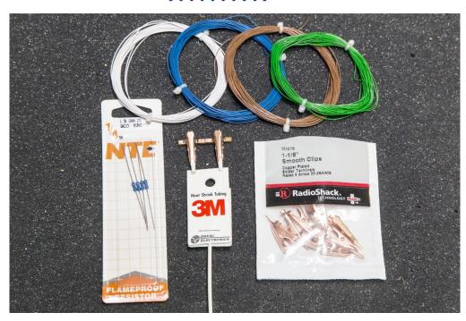
3. I use the Radio Shack clips as holding clamps. I buy heat-shrink tubing from an electronics vendor like Mouser (mouser. com) or Digi-Key (digikey.com). It comes in various sizes and colors, and in three-foot lengths. These vendors also sell resistors. I found the decoder wire on sale at a local hobby shop. Decoder wire comes in 10-foot lengths in a variety of colors.
