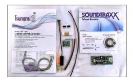
Dead Rail Installs is selling a kit that includes all of the components needed to install a Soundtraxx Tsunami2 or Econami Decoder in a dead rail model. In addition to optional decoders, the kit includes
