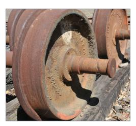
1. A prototype wheel and axle. The larger diameter section on the end of the axle is the "journal collar" while the portion of the axle next to the wheel with the same diameter is the "wheel seat." The axle bearing surface is the portion of the axle between the journal collar and the wheel seat. A
