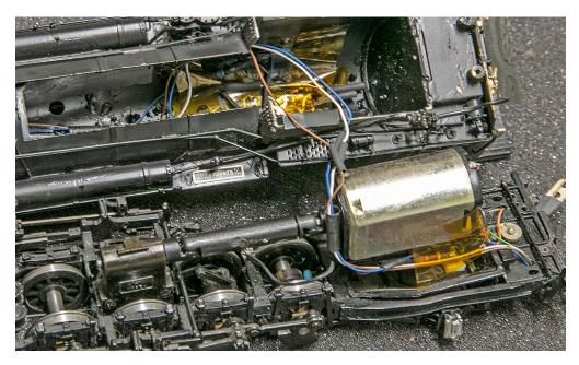
10. The wire harness is threaded through the engine. Heat-shrink tubing serves as a conduit to keep the wires in place.
