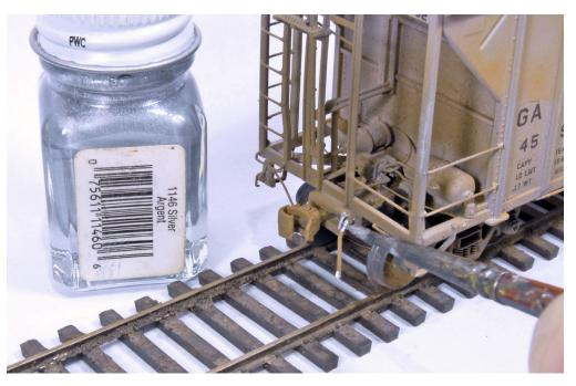
22. The weathering process is almost complete. One final step is to highlight the air hose coupling detail with silver paint.
