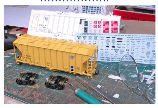
1. The GACX 45992 sports the triangle reinforced slope sheets. Athearn offers this option. These models are not in current production but I was able to find this model on eBay. I start by removing the trucks, and replace the plastic couplers with the tried and true Kadee #5.
