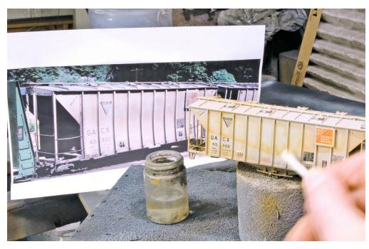
17. I clean the face of the ribs using a new Q-tip and Turpenoid thinner.
