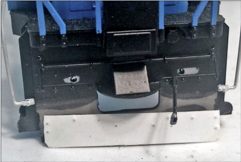
10. The sanded pilot and steel plate with drill holes marked with a sharp needle point to show where the bolt heads will be added once it's glued in place.
