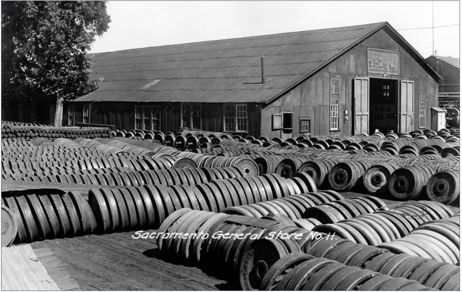
13. The wheel storage area outside Building 11 of the General Stores at Sacramento General Shops of the Southern Pacific. Wheels here are mostly new, but some rows of worn-out wheels can also be seen. A line of wheel-sets is near the building. Southern Pacific photo X8351-04, John R. Signor collection
