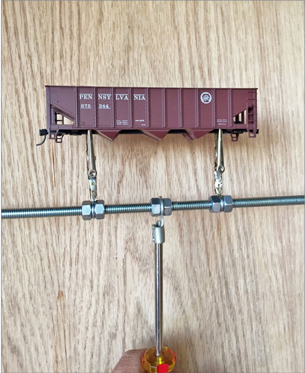
4. Close-up of a Roundhouse hopper mounted on the painting handle.
